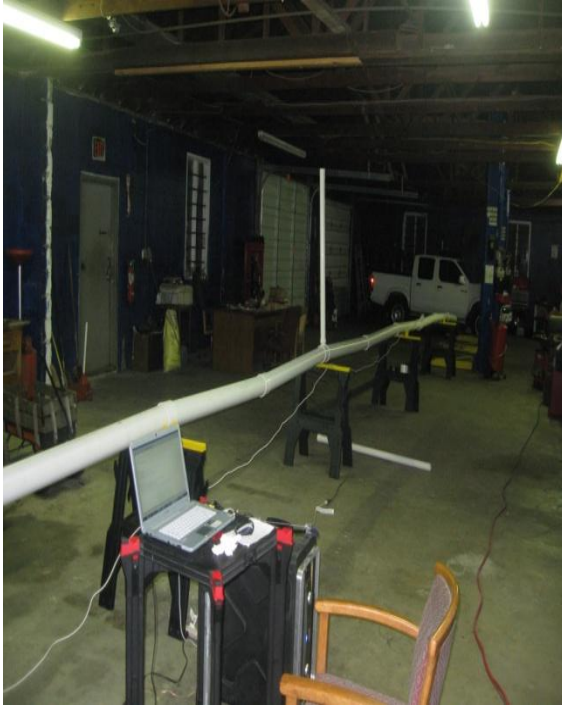
Figure 36: Test set up – 17.56 m long conduit with one side branch.
