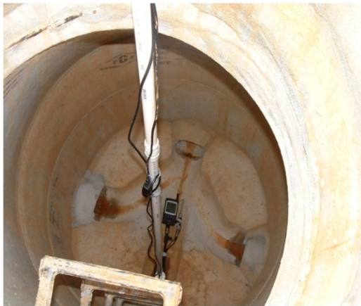
Figure 29: Audio spectrum analyzer and condenser microphone at receiving location.
