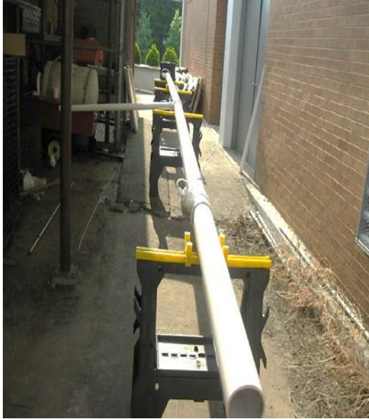
Figure 33: Conduit with one side branch.
