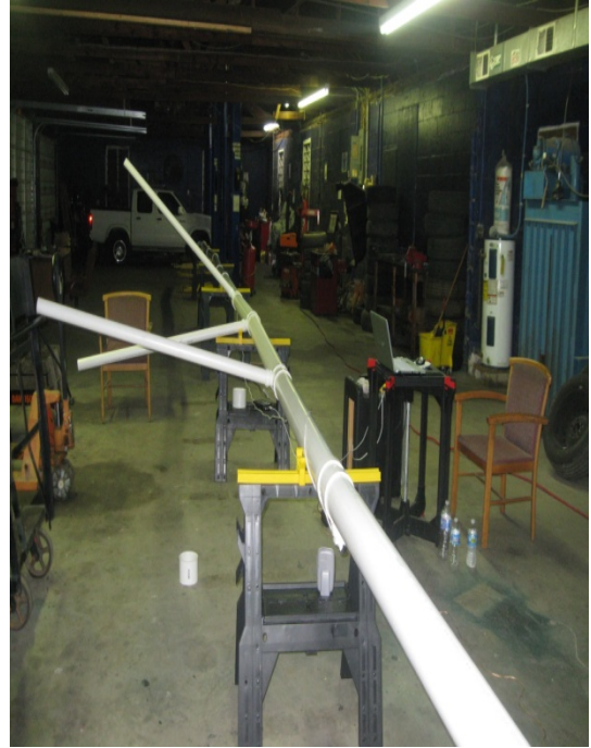
Figure 37: Test set up – 17.56 m long conduit with three side branches.
