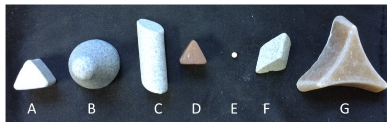
Figure 5.2: Seven media types used. A) RS 10/10, B) RS 19K, C) RS 10/22 ZS, D) RDP 09/09, E) 2mm Ball, F) RS 10/10S and G) 2050 40/13 DZ
