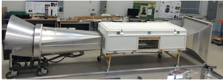
Figure 4.1: Original configuration of UNC Charlotte Motor Sports Research Lab scale wind tunnel
