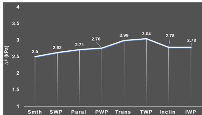
Figure 9. Pressure drop for *turbulent flow* ( $Re = 4000$ ).
