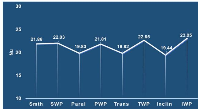
Figure 6. Nu for *laminar flow* ( $Re = 1000$ ) conditions. See the nomenclature section for interpretation of the horizontal axis labels.
