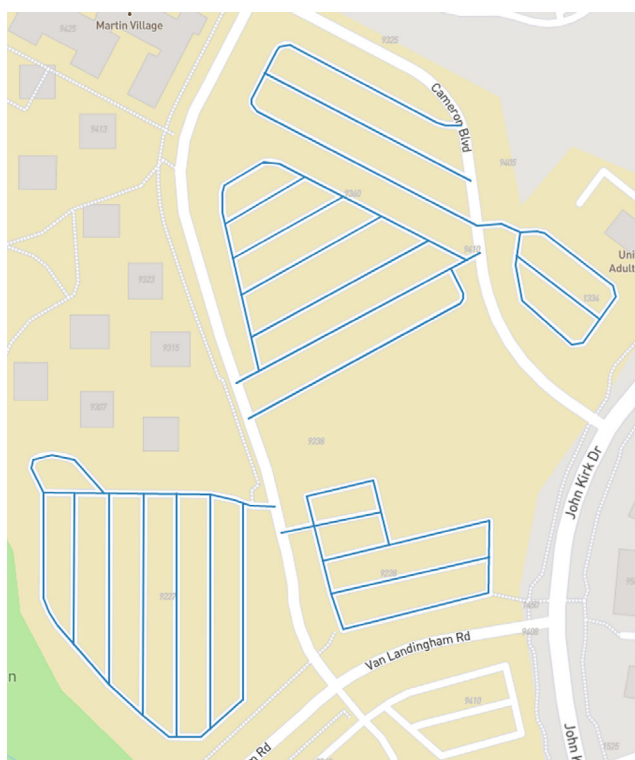
FIGURE 15 A network of lanes specified on a set of parking lots: The total length of the lanes is 2982 m. There are 90 vertices, 104 required edges, and 4005 non-required edges. The required edges form four connected components.
