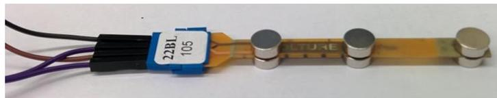
Figure 25: Harvester 2 construction for physical layout I
