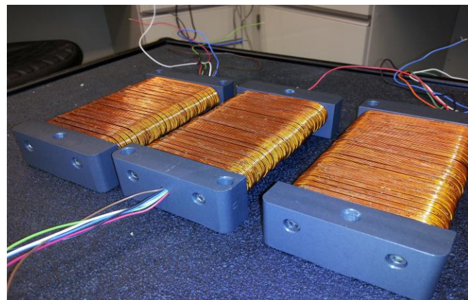
Figure 70: Halbach motor's stators.
