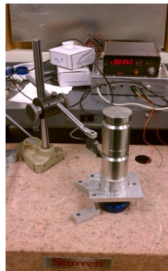
Figure 83: Air bearing calibration setup.
