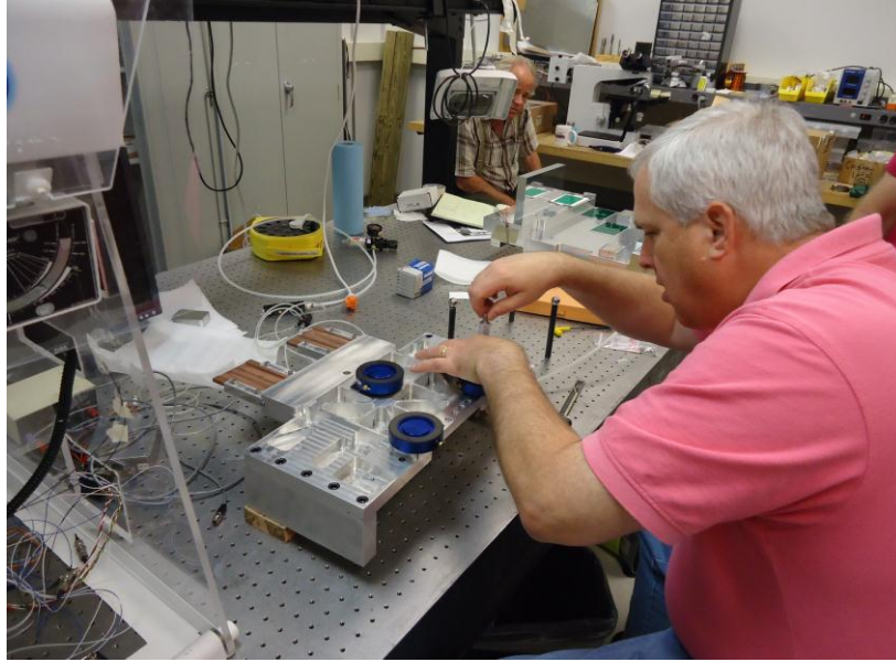
Figure 110: Greg Caskey, of the Center for Precision Metrology at UNC Charlotte, checking the level of the air bearings after assembly.
