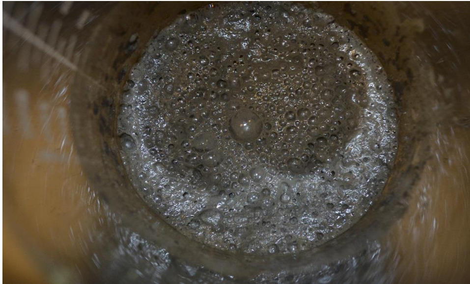
Figure 3.1b: Foam index test end point (100% Foam Coverage)
