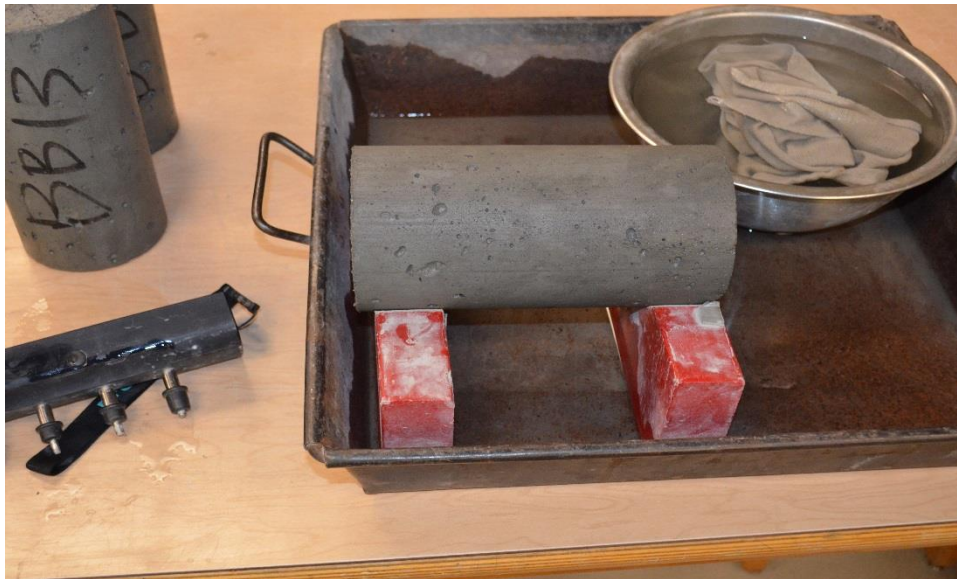
Figure 3.7a: Concrete cylinder specimen on supports
