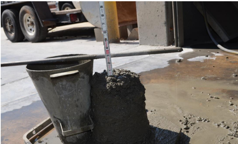
Figure 3.4b: Measurement of slump
