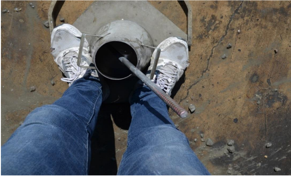
Figure 3.4a: Slump mold held firmly to prevent vibration
