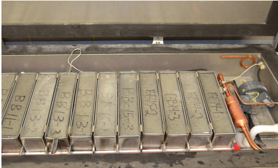
Figure 3.8b: Concrete specimen in freeze thaw apparatus
