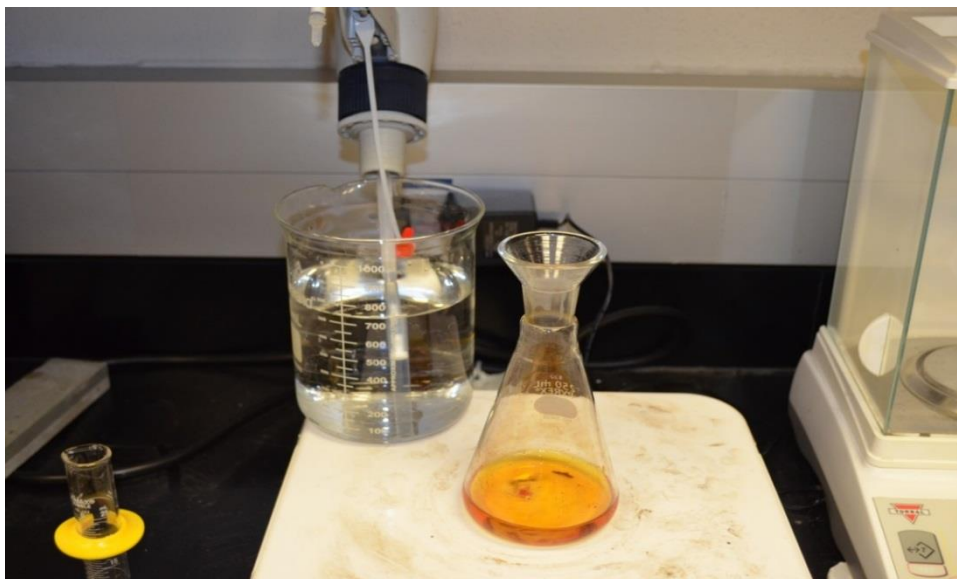
Figure 3.2a: Pale yellow solution after addition of 0.025N sodium thiosulfate solution
