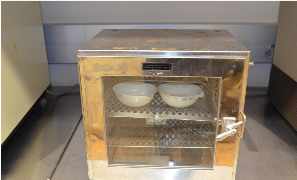
Figure 3.3b: Specimens of fly ash cooling in desiccator
