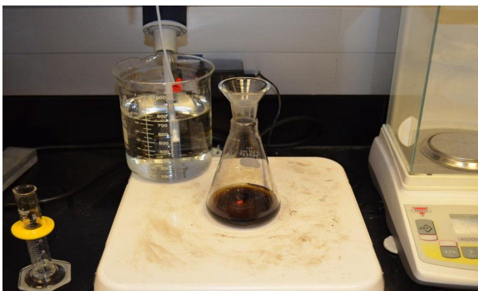
Figure 3.2b: Black solution after addition of 1% starch solution as indicator
