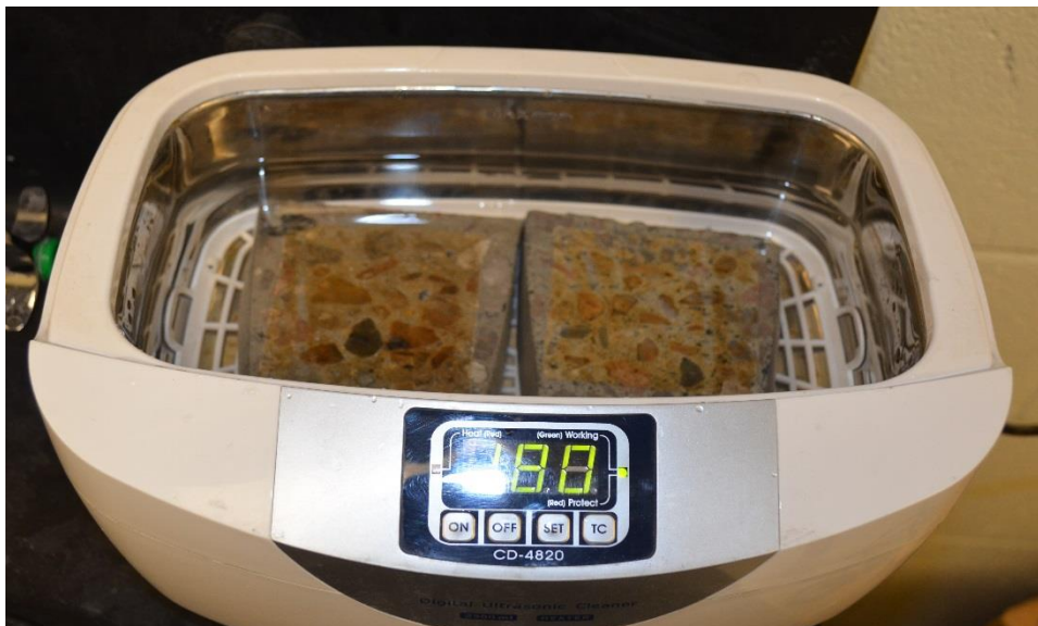
Figure 3.9d: Polished Concrete specimen in ultrasonic cleaner
