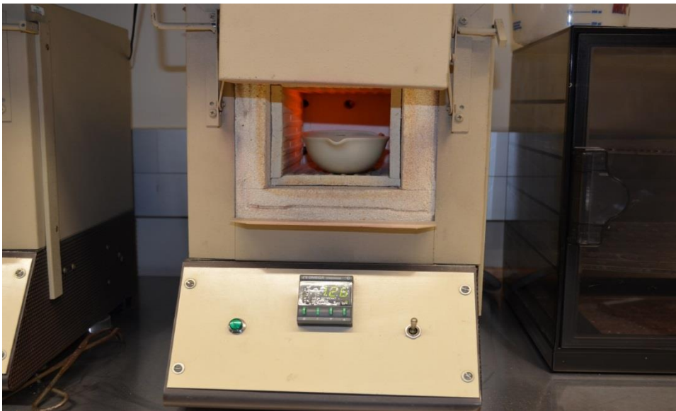
Figure 3.3a: Specimens of fly ash heating in muffle furnace
