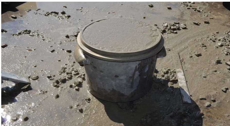
Figure 3.5a: Fresh concrete in SAM bowl with rim cleaned properly
