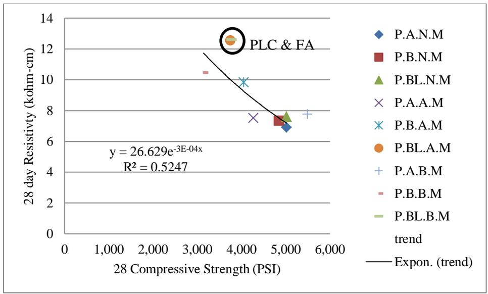
Figure 5.11: 28 day resistivity vs. 28 day compressive strength
