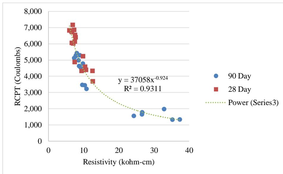
Figure 5.10: Combined RCPT vs. surface resistivity
