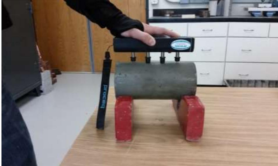
Figure 3.8: Surface resistivity Proceq set up
