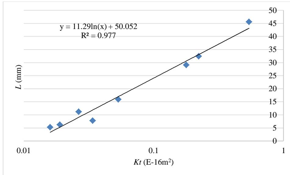
Figure 5.1: Air permeability  $Kt$  vs.  $L$
