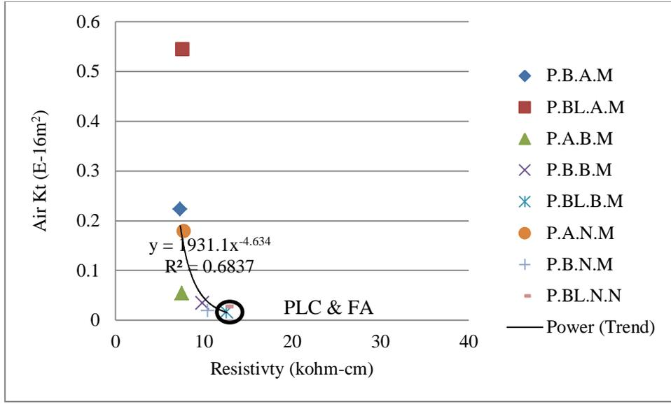
Figure 5.4: Air permeability vs. 28 day surface resistivity results
