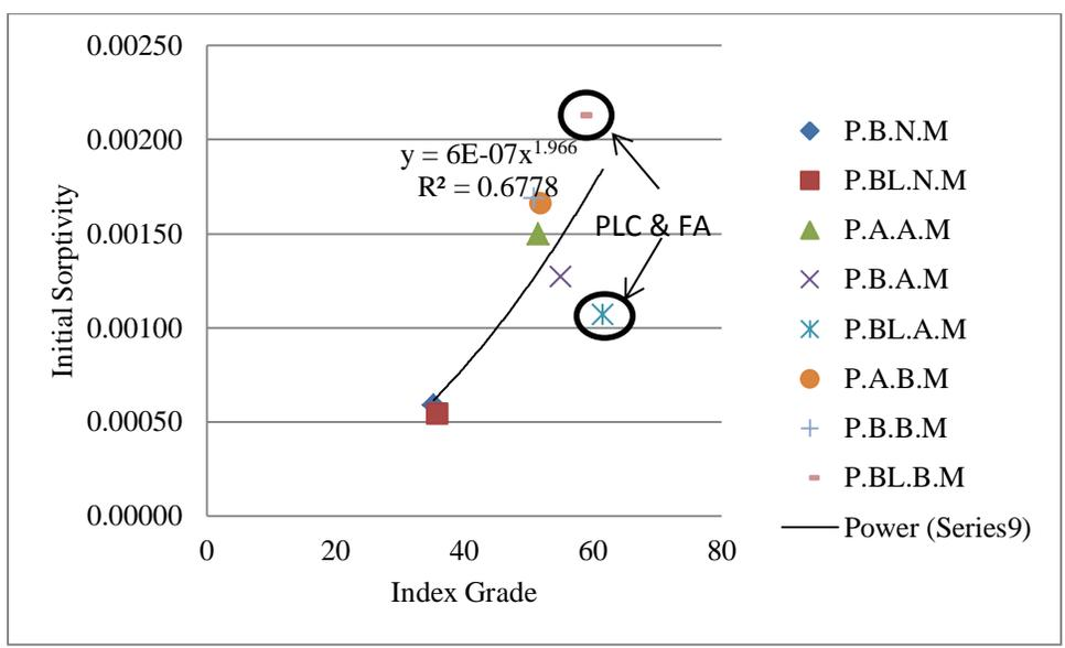
Figure 5.22: Initial sorptivity vs. index grade
