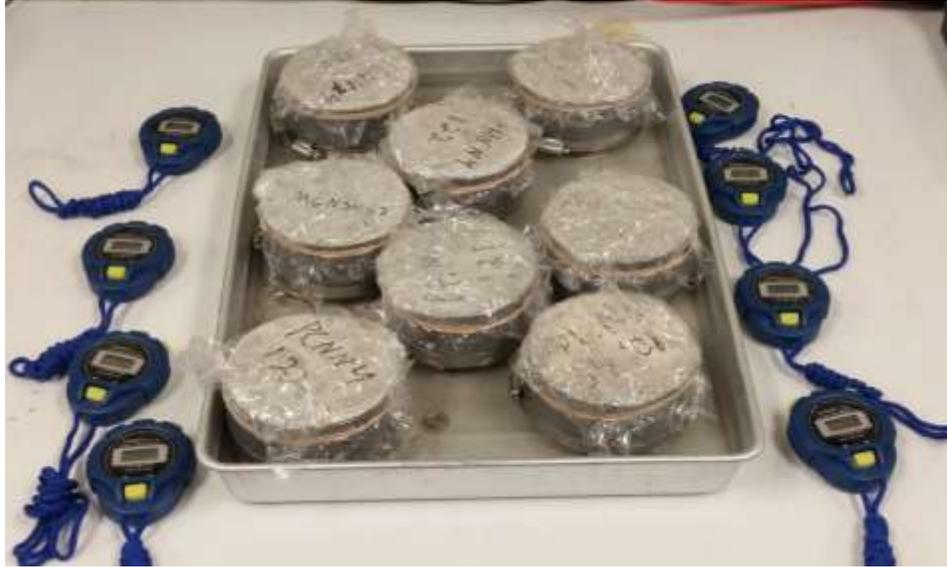
Figure 3.4: Suction method test set up
