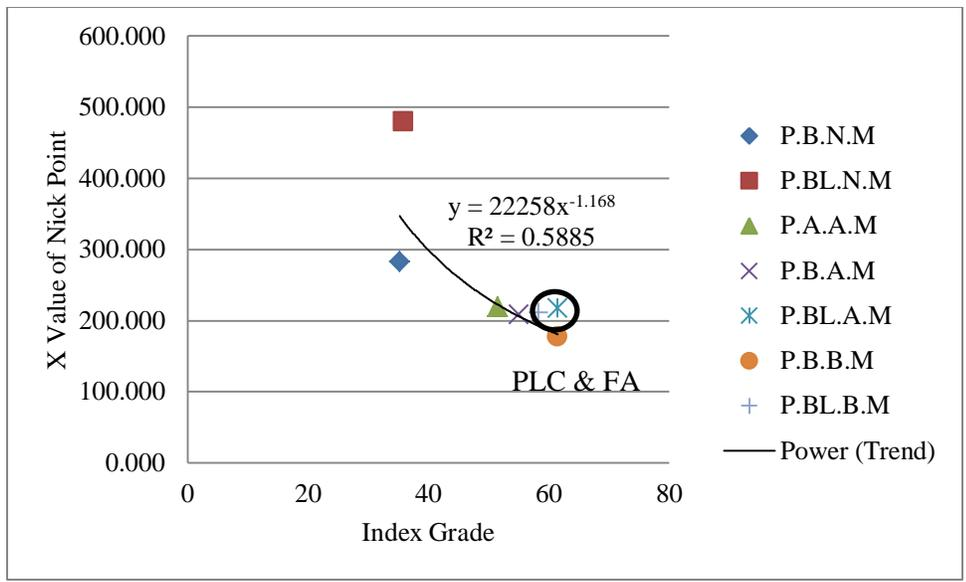
Figure 5.24: X coordinate of nick point vs. index grade
