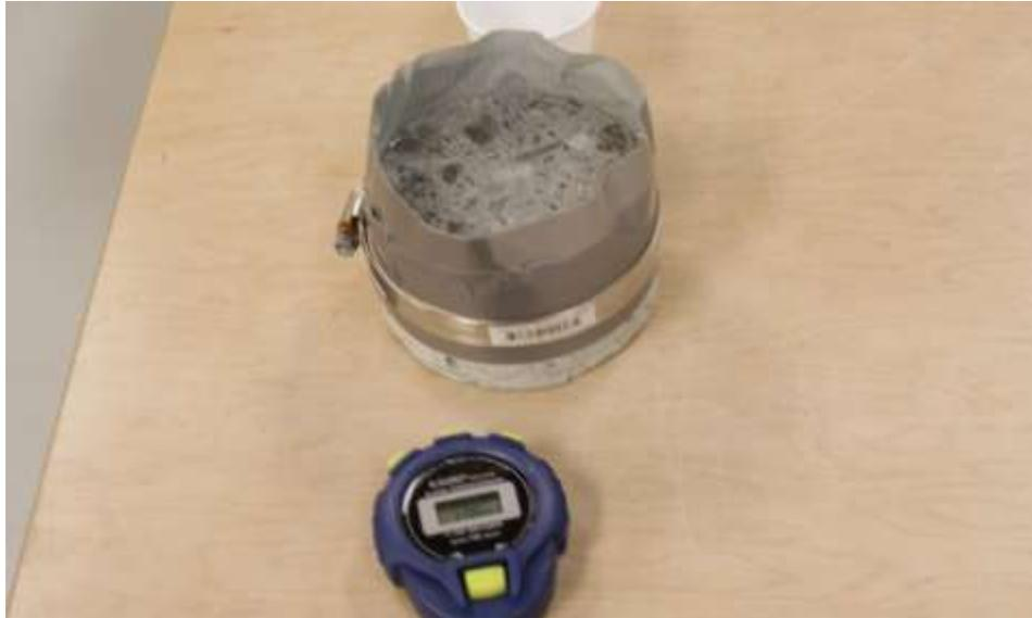
Figure 3.5 Ponding test set up
