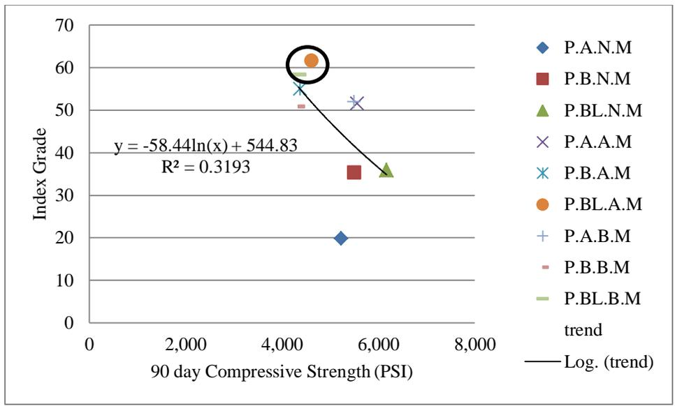
Figure 5.15 Index grade vs 90 day compressive strength
