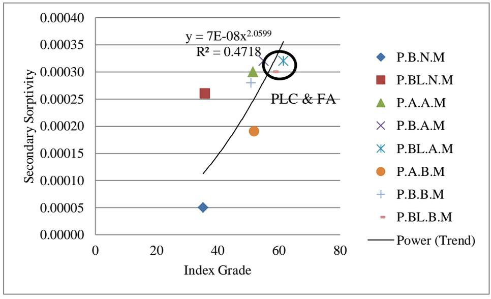
Figure 5.23: Secondary sorptivity vs. index grade
