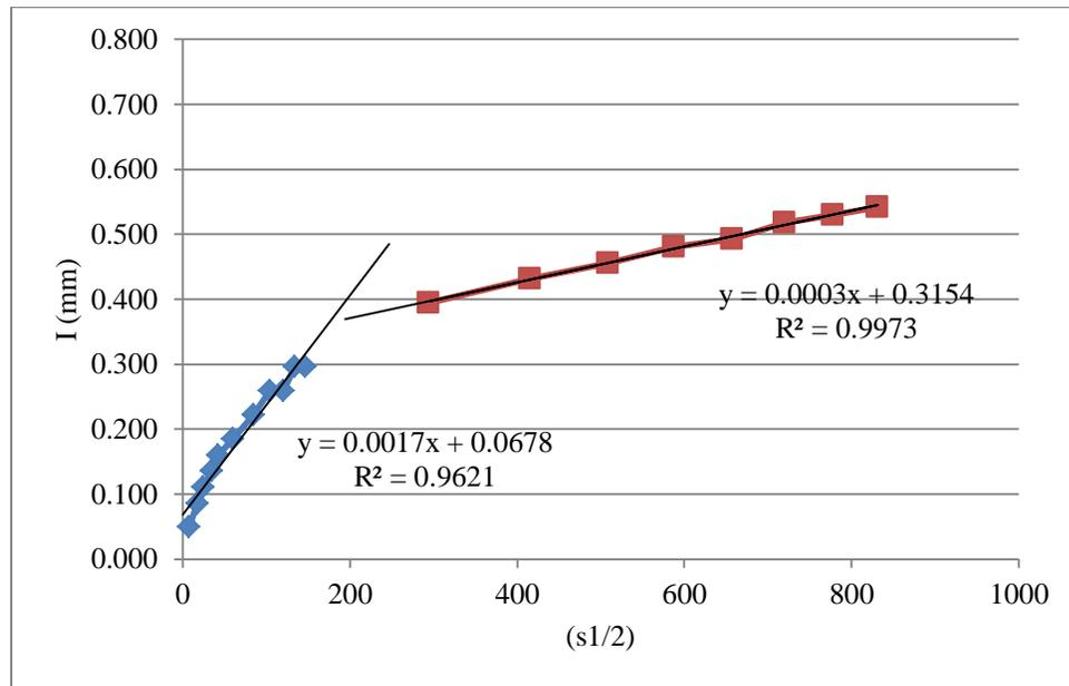
Figure 4.1: Example sorptivity graph (Sample P.B.B.M)
