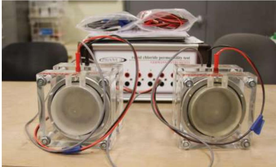
Figure 3.7: RCPT sample test set up
