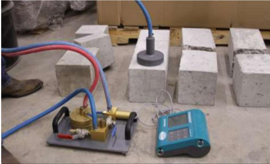
Figure 3.9: Torrent air permeability set up
