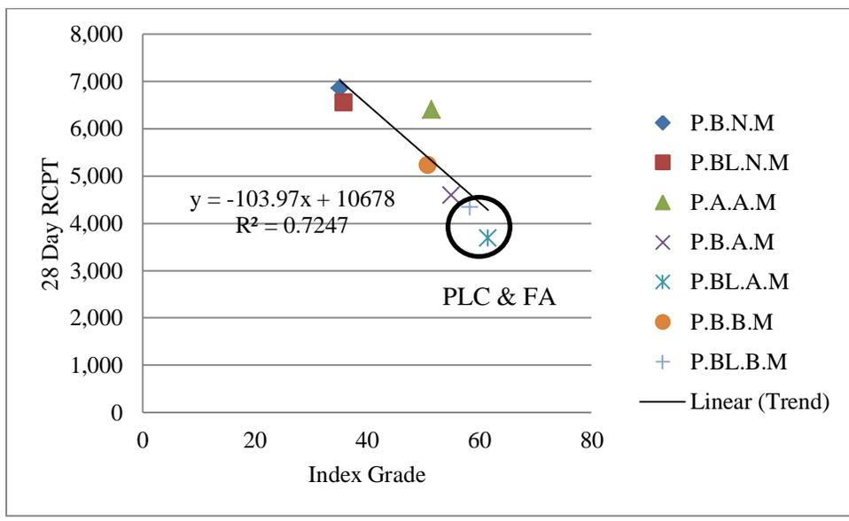
Figure 5.17: 28 day RCPT vs index grade
