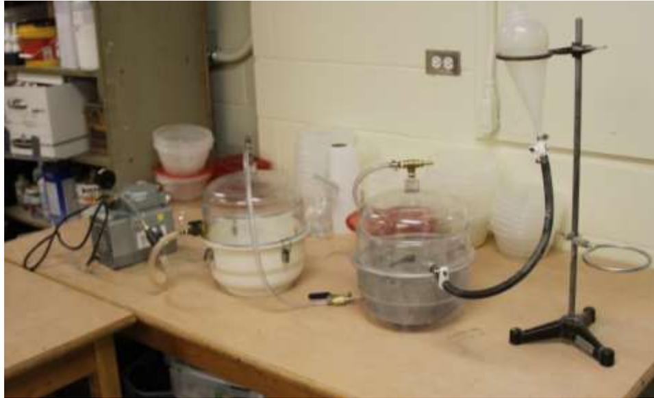
Figure 3.6: RCPT samples conditioning
