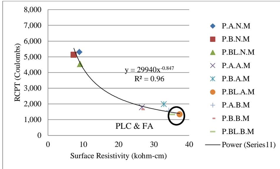
Figure 5.7: Select 90 day RCPT vs. surface resistivity
