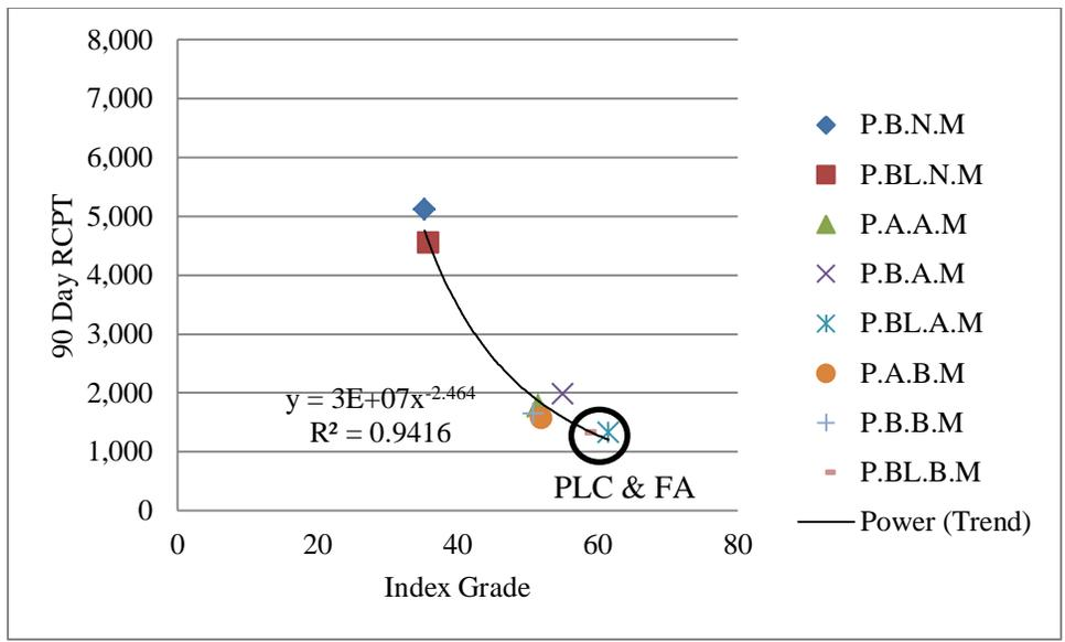
Figure 5.18: 90 day RCPT vs index grade
