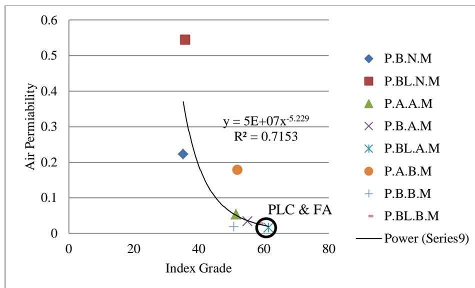
Figure 5.21: Air permeability vs index grade
