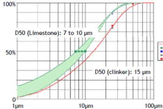
Figure 2.1: Limestone particle size distribution (Tennis et al., 2011)
