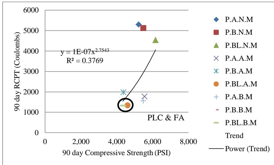
Figure 5.14: 90 day RCPT vs compressive strength
