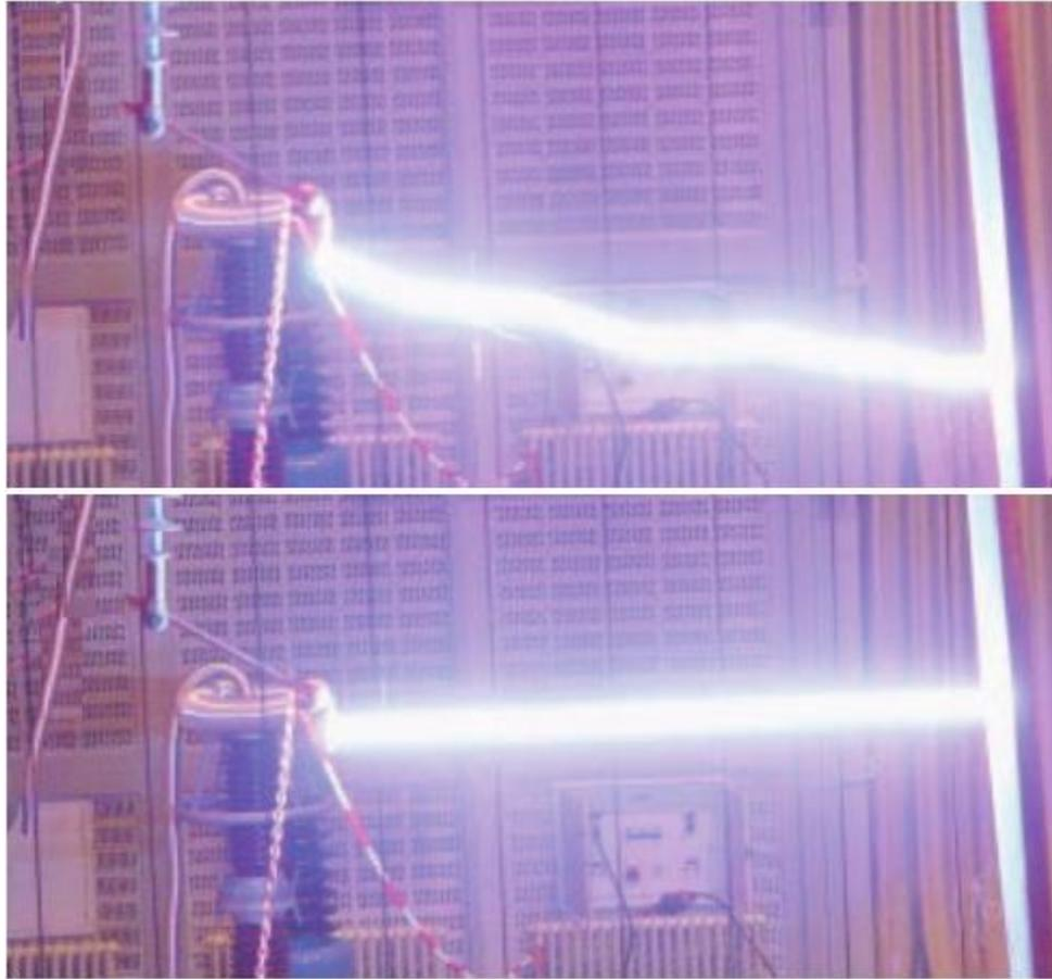
Fig. 6. Laser control of high-voltage plasma discharge [21]
