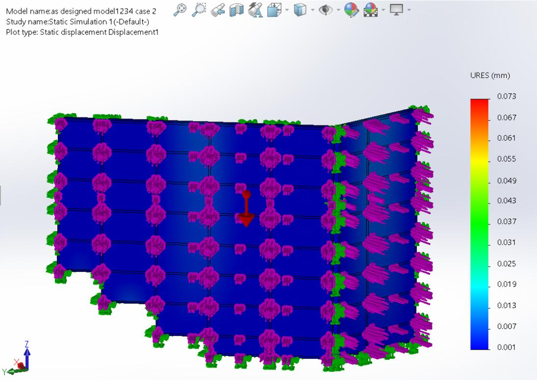
FIGURE 15: Deformation of the as-designed Model (Case 2- 20mph)
