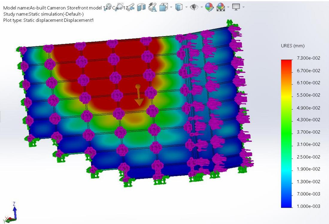
FIGURE 36: Deformation of the as-built Model (Case 12- 70mph)
