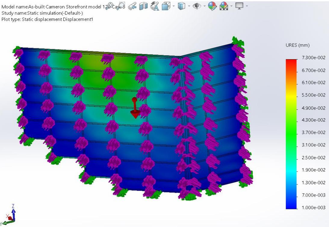
FIGURE 22: Deformation of the as-built Model (Case 5- 35mph)
