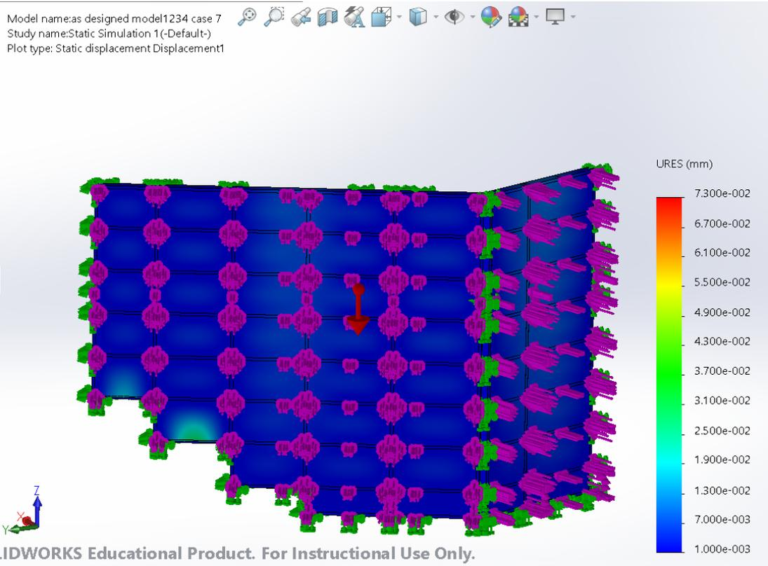
FIGURE 25: Deformation of the as-designed Model (Case 7- 45mph)
