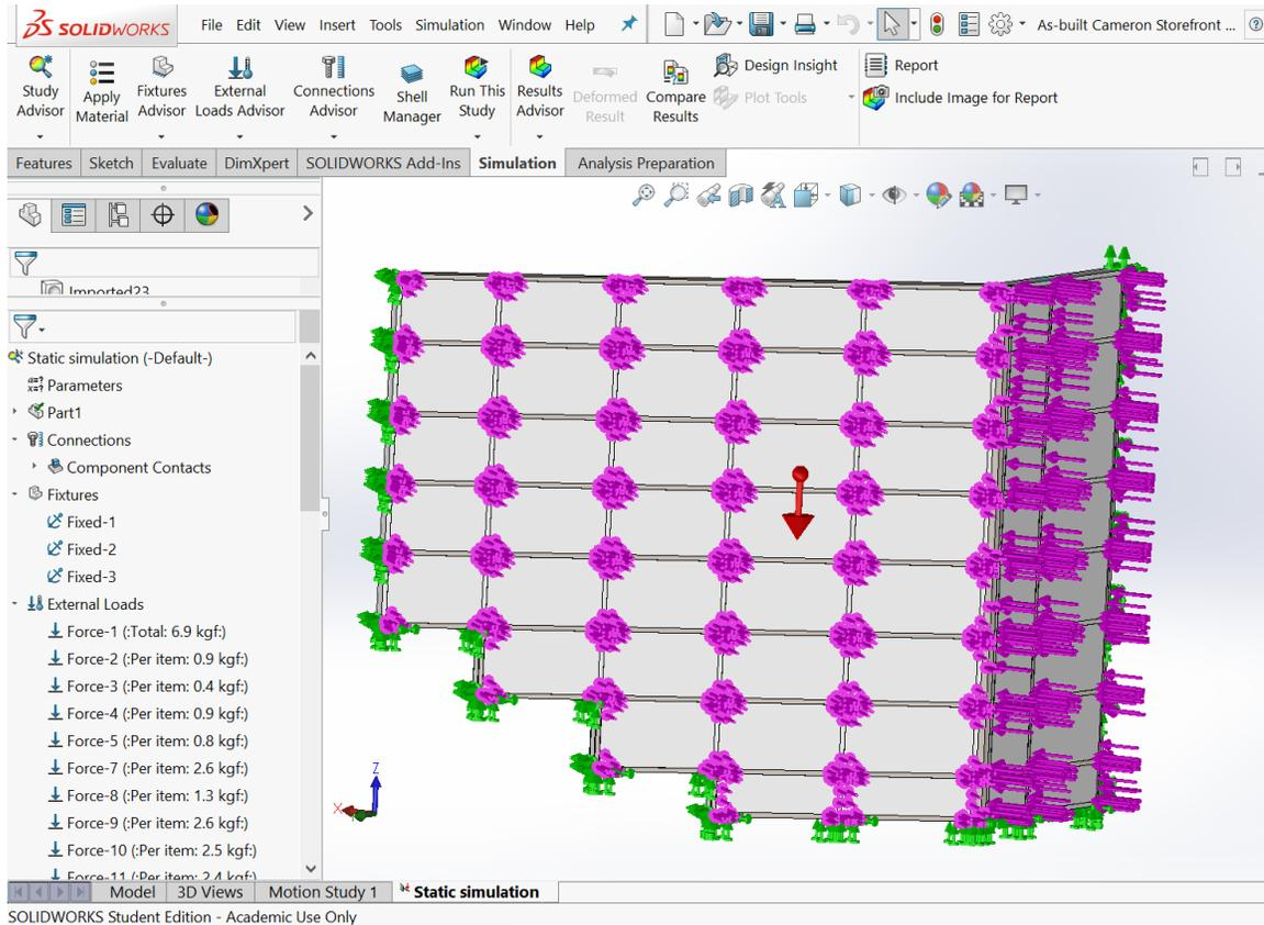
FIGURE 11: Boundary conditions and Loads applied to the wall
