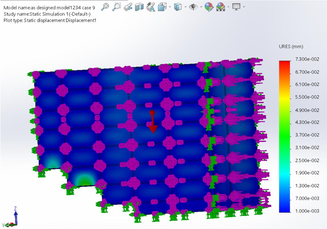
FIGURE 29: Deformation of the as-designed Model (Case 9- 55mph)
