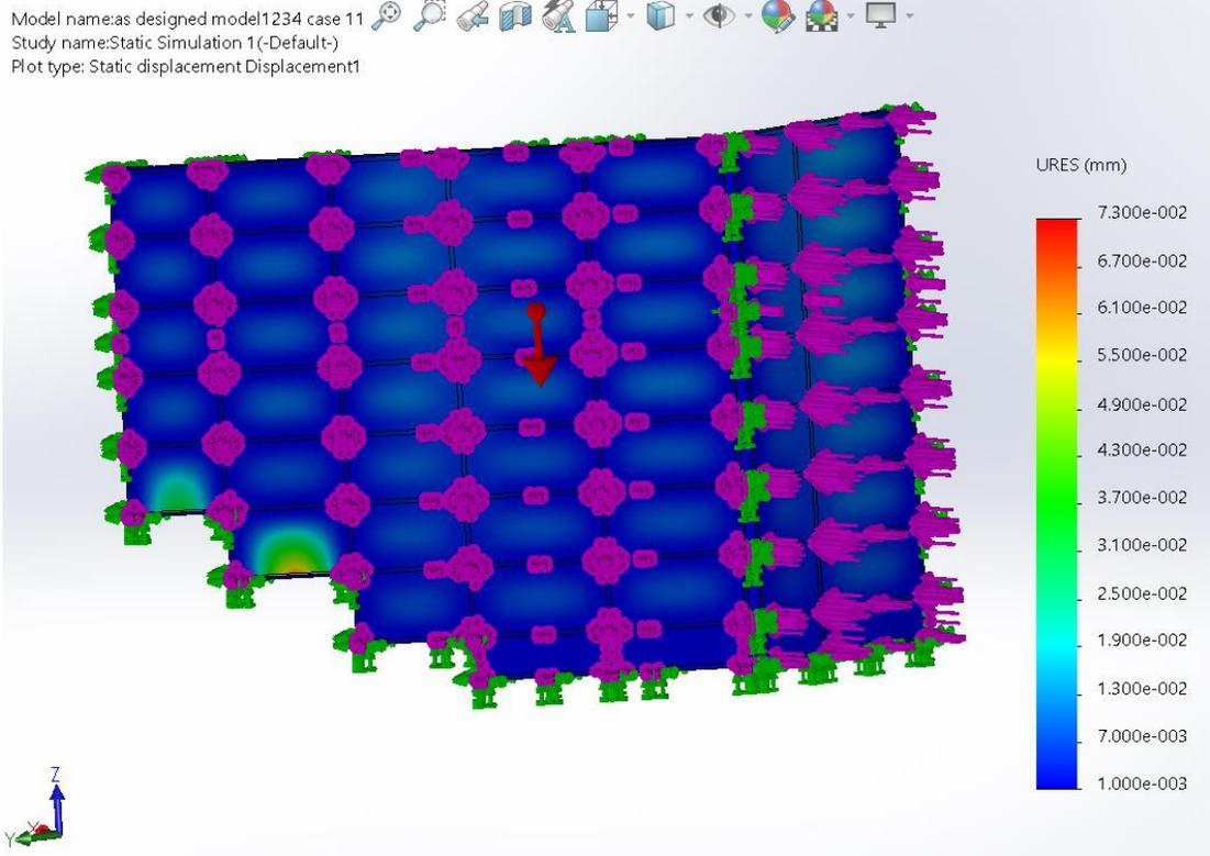
**FIGURE 33: Deformation of the as-designed Model (Case 11- 65mph)**
