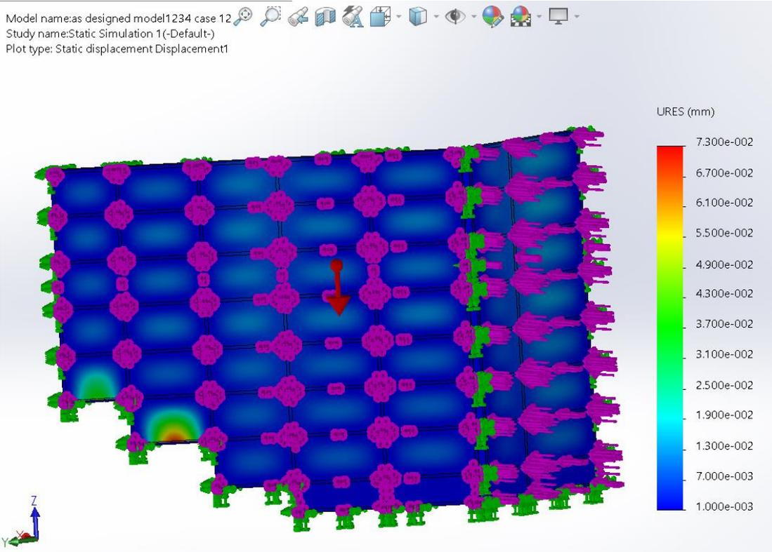
FIGURE 35: Deformation of the as-designed Model (Case 12- 70mph)
