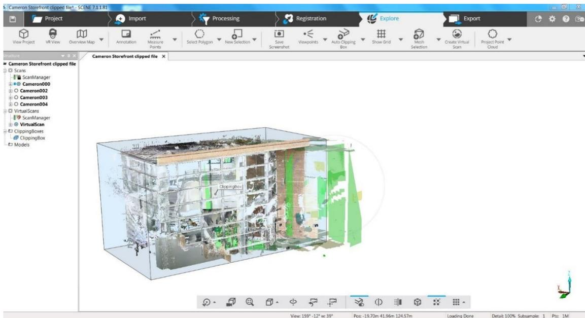
FIGURE 4: Exploring the point cloud in SCENE
