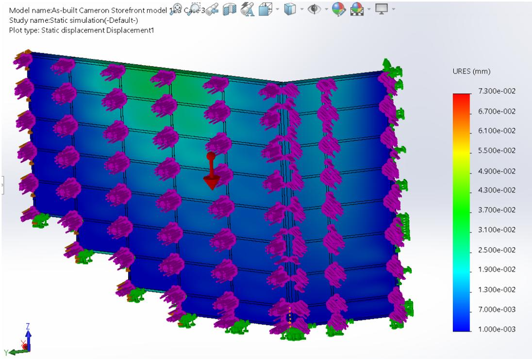
**FIGURE 18: Deformation of the as-built Model (Case 3- 25mph)**
