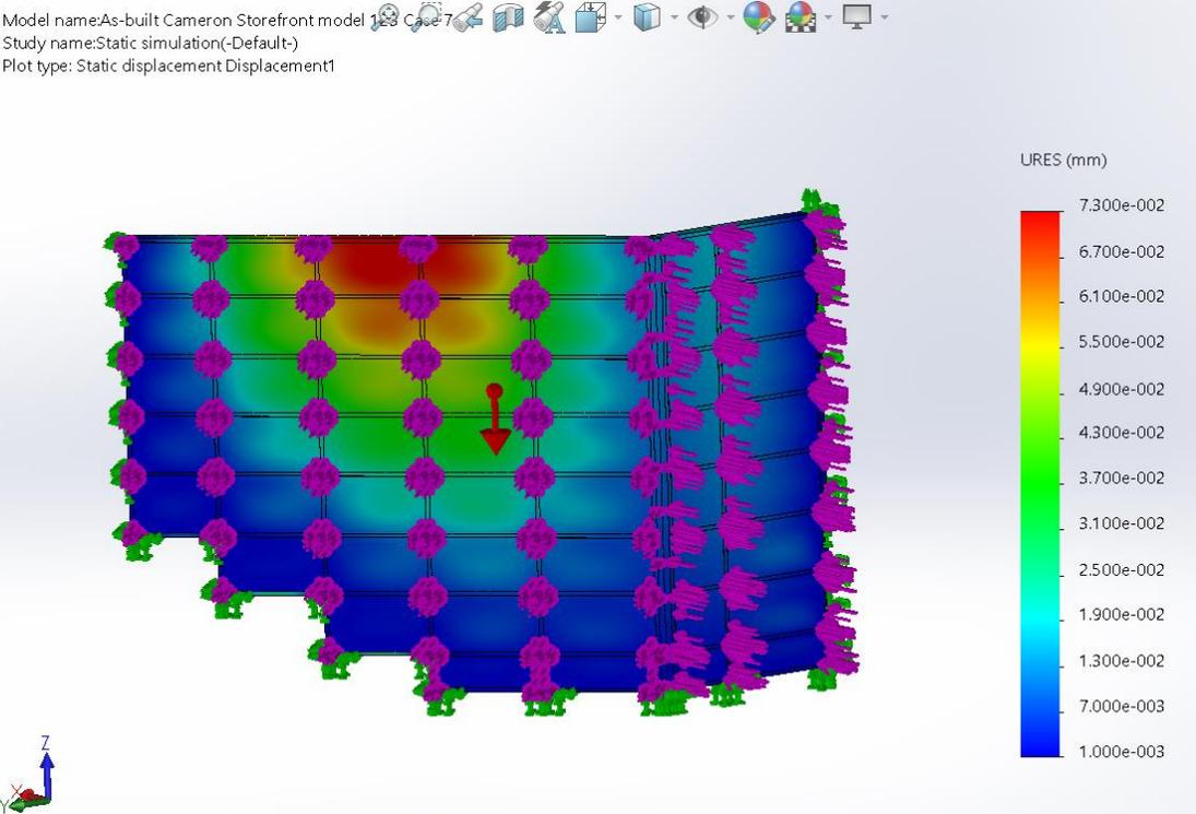
FIGURE 26: Deformation of the as-built Model (Case 7- 45mph)
