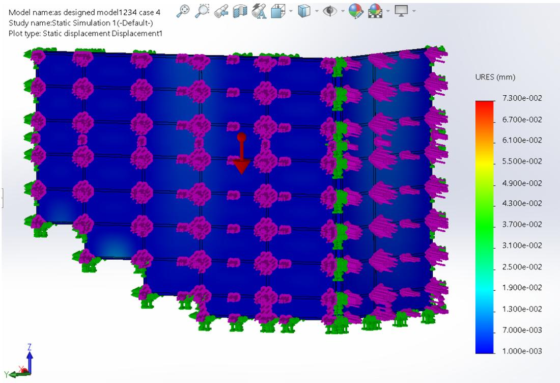
*FIGURE 19: Deformation of the as-designed Model (Case 4- 30mph)*
