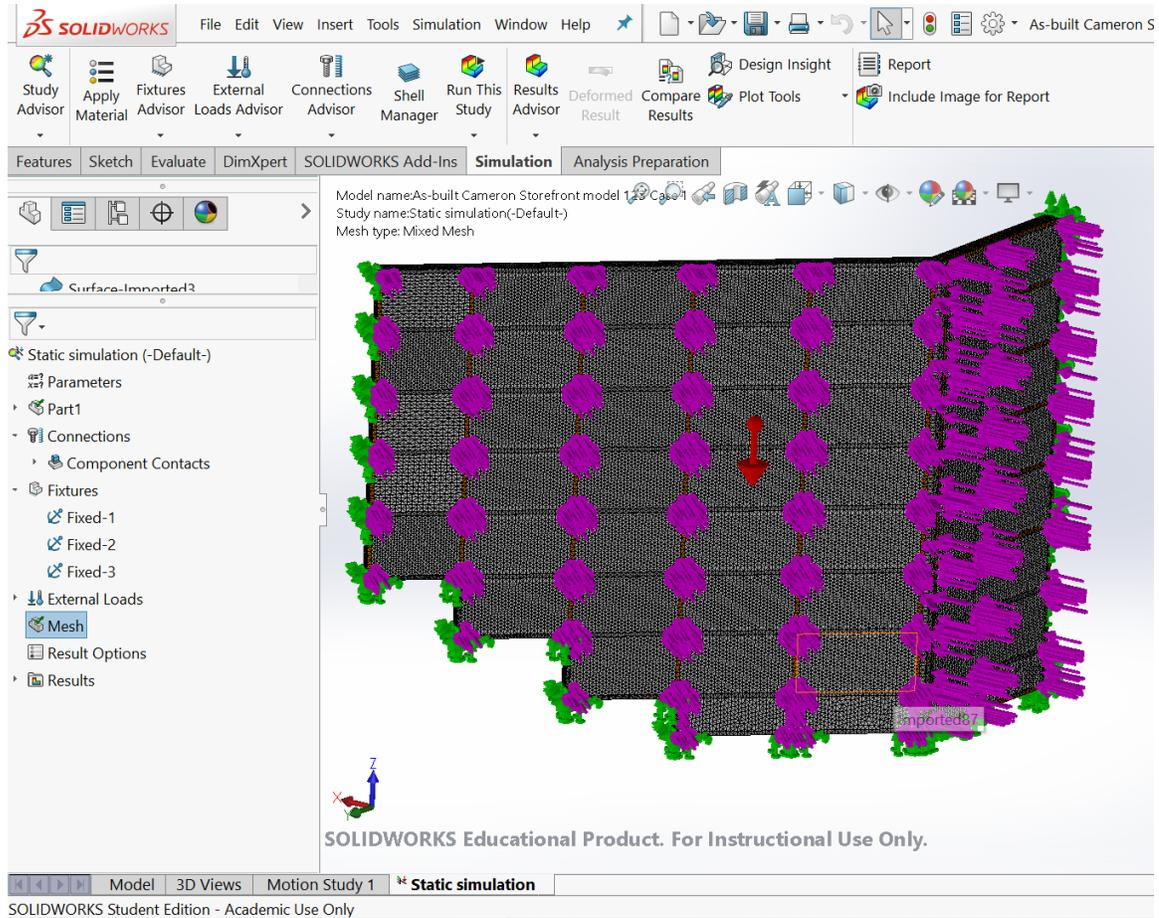
27992282.99 psi. After updating the Solid works model with material properties of the curtain wall, loading it with dead load and wind load and adding the boundary conditions of the wall, it meshes into smaller components.
