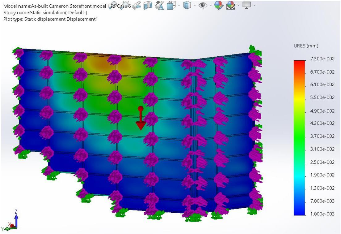
FIGURE 24: Deformation of the as-built Model (Case 6- 40mph)
