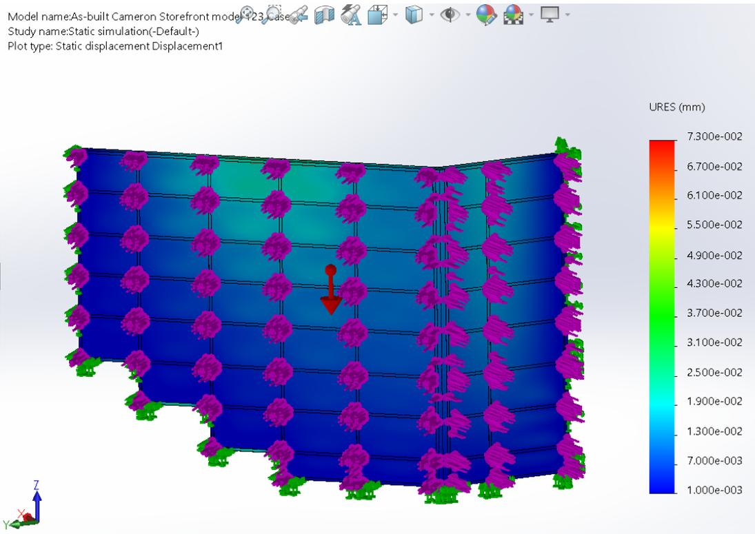
FIGURE 16: Deformation of the as-built Model (Case 2- 20mph)
