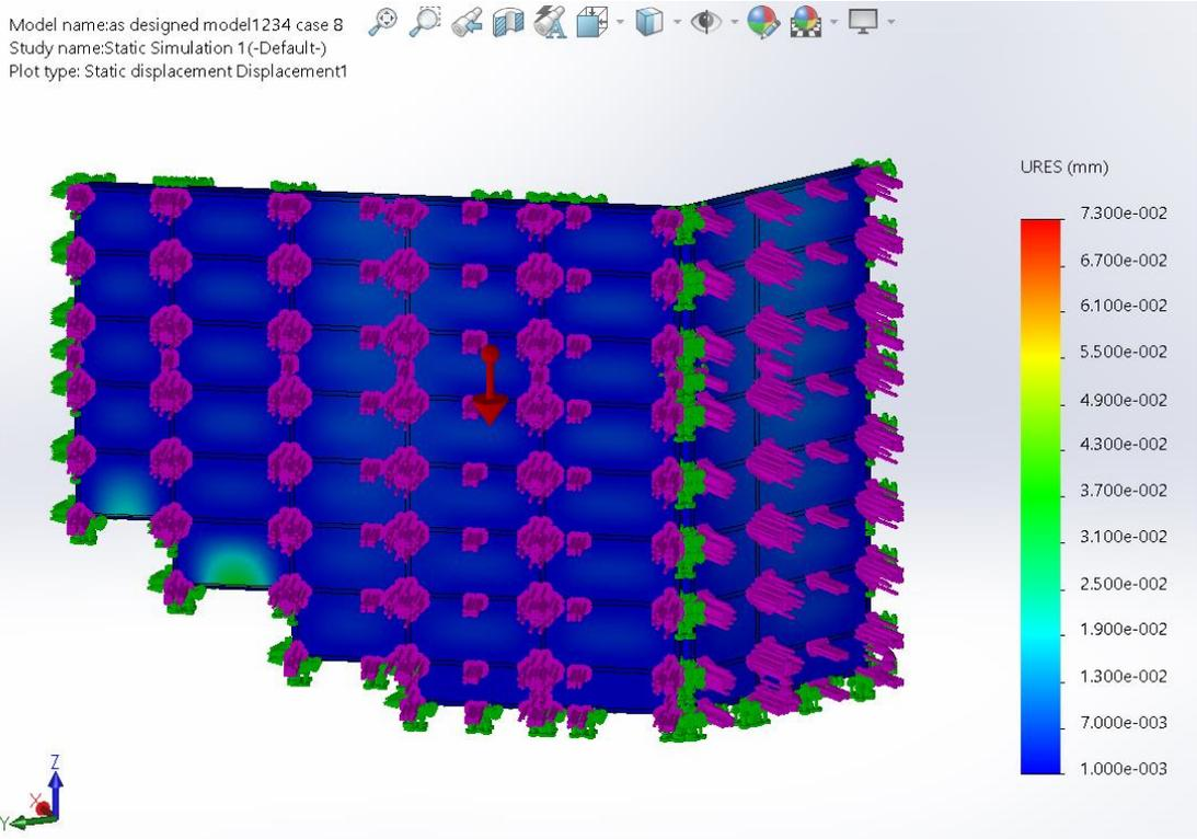
FIGURE 27: Deformation of the as-designed Model (Case 8- 50mph)
