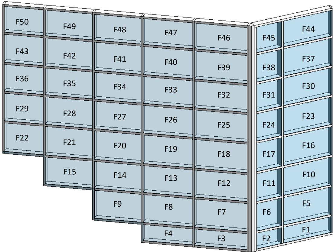
FIGURE 9: Legend of the forces applied to the curtain wall panels
