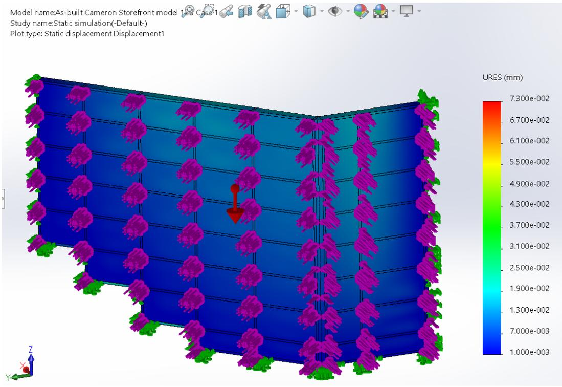
FIGURE 14: Deformation of the as-built Model (Case 1- 12mph)
