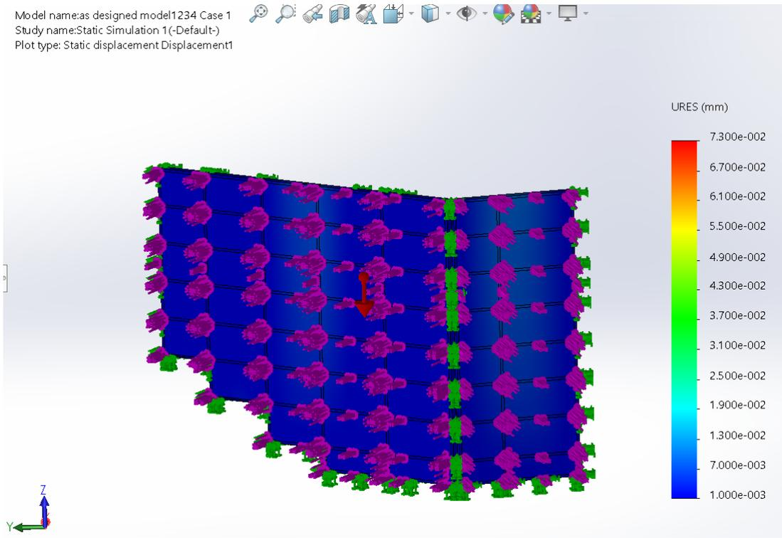
FIGURE 13: Deformation of the as-designed Model (Case 1- 12 mph)
