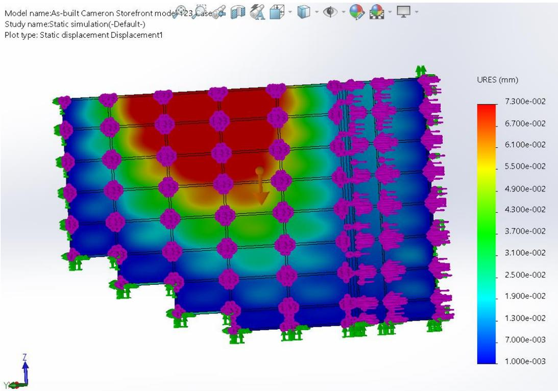
**FIGURE 32: Deformation of the as-built Model (Case 10- 60mph)**
