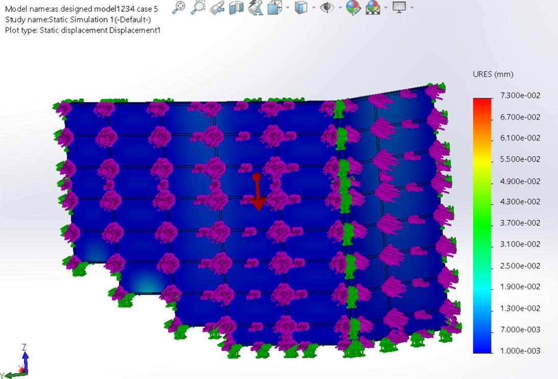
FIGURE 21: Deformation of the as-designed Model (Case 5- 35mph)
