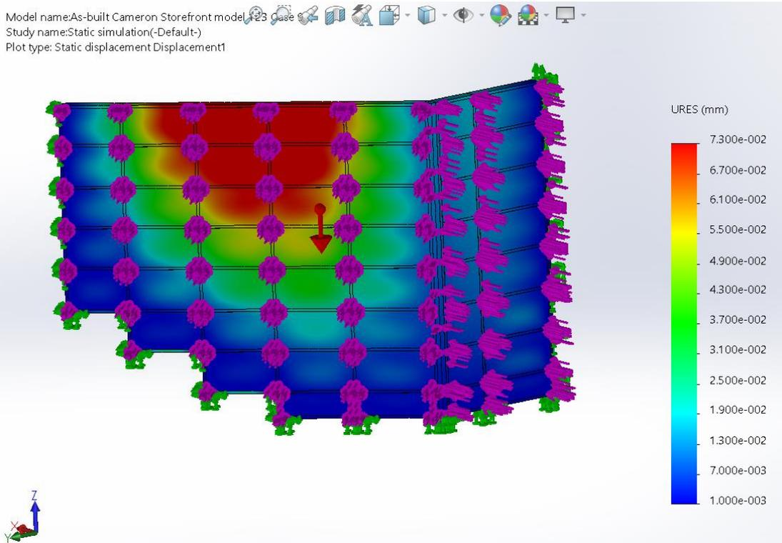
FIGURE 30: Deformation of the as-built Model (Case 9- 55mph)
