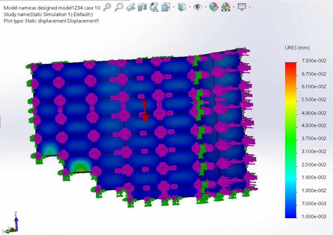
**FIGURE 31: Deformation of the as-designed Model (Case 10- 60mph)**
