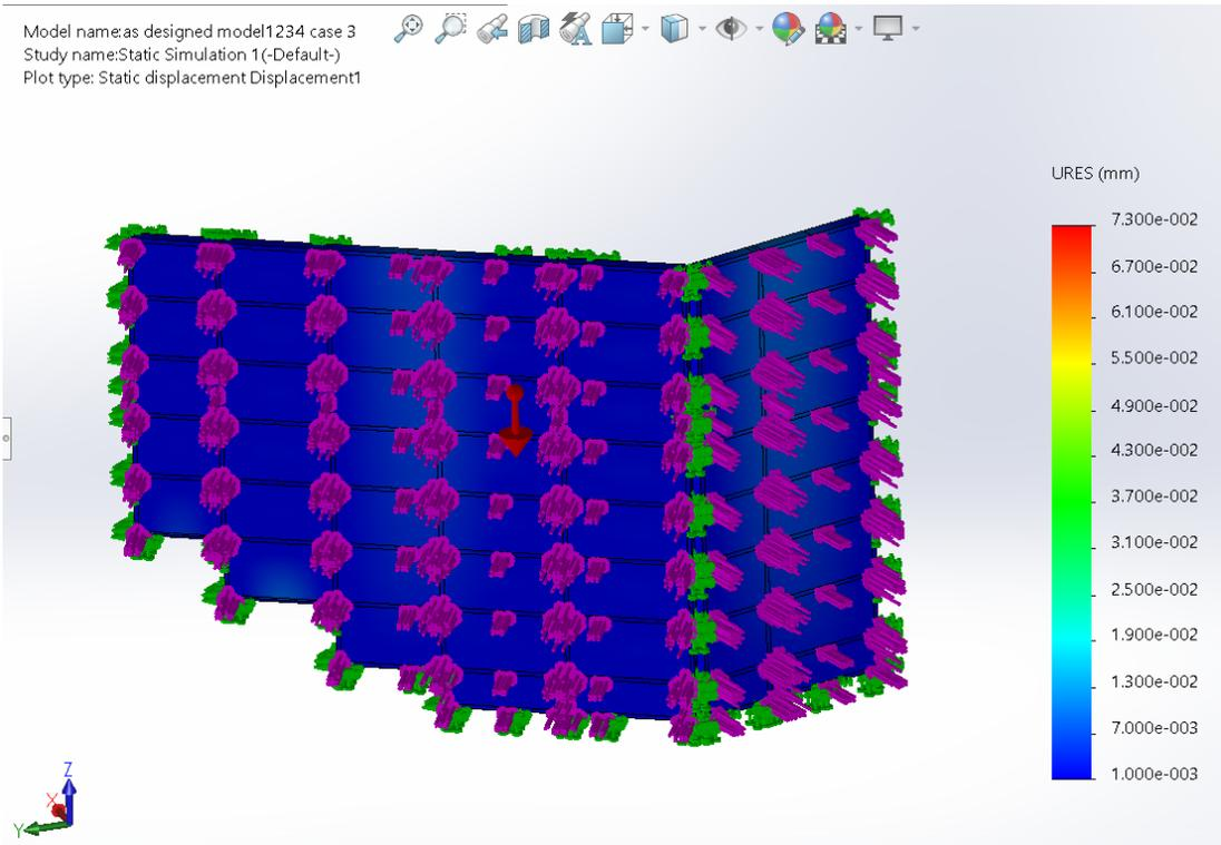
**FIGURE 17: Deformation of the as-designed Model (Case 3- 25mph)**
