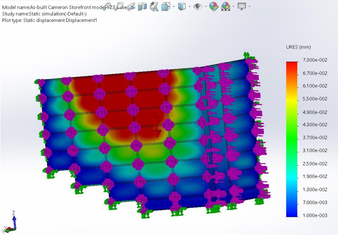
**FIGURE 34: Deformation of the as-built Model (Case 11- 65mph)**
