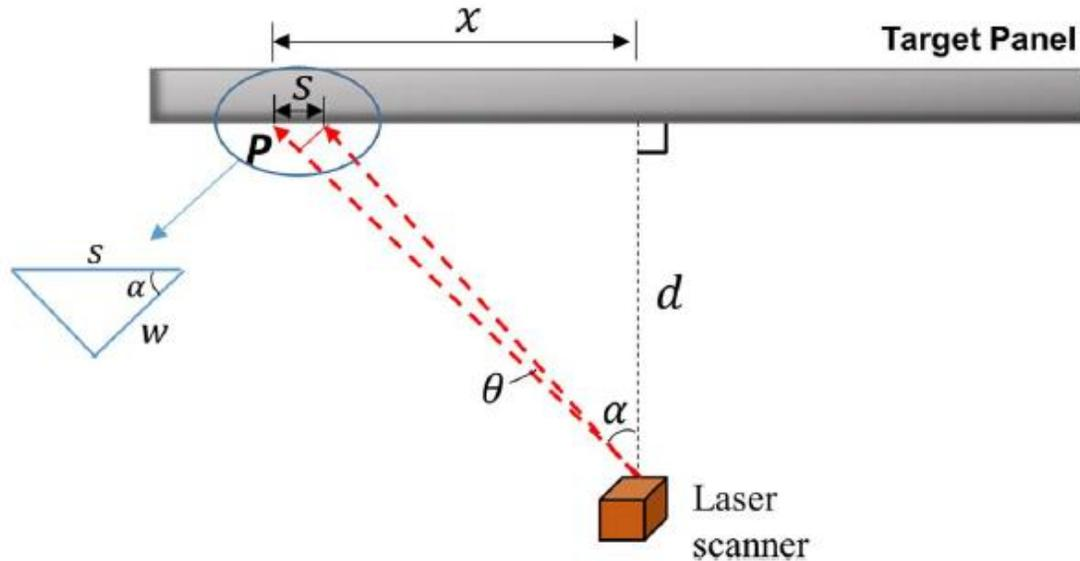
FIGURE 1: Illustrative scanning setting for a target panel showing the relationships between scan parameters such as  $d$ ,  $\alpha$ ,  $s$ , and  $\vartheta$
