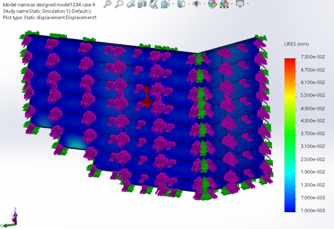
FIGURE 23: Deformation of the as-designed Model (Case 6- 40mph)
