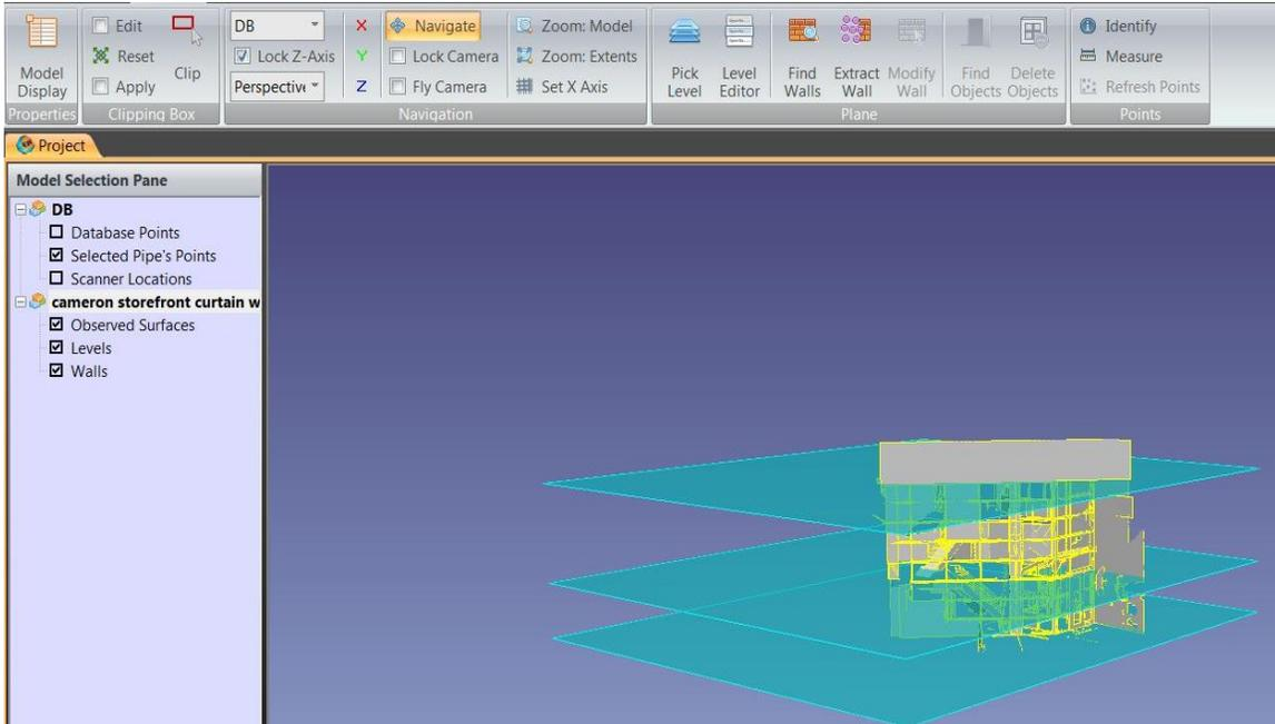
FIGURE 7: Levels automatically picked up in Edgewise
