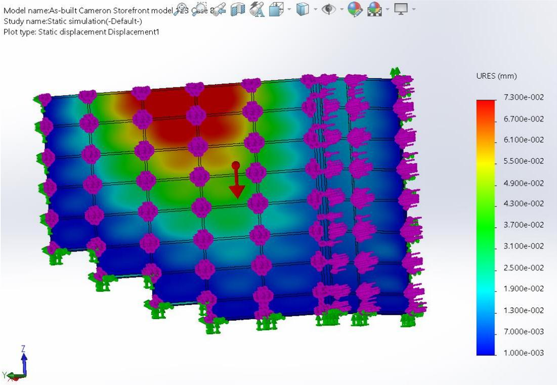
FIGURE 28: Deformation of the as-built Model (Case 8- 50mph)
