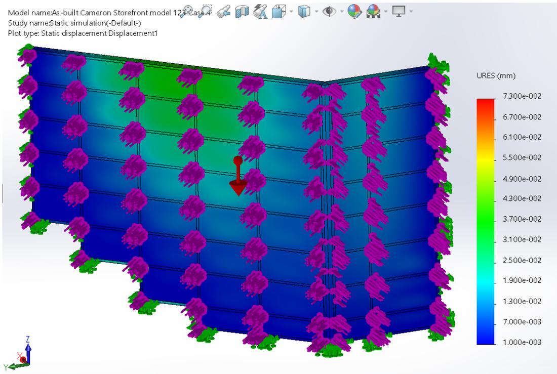
*FIGURE 20: Deformation of the as-built Model (Case 4- 30mph)*
