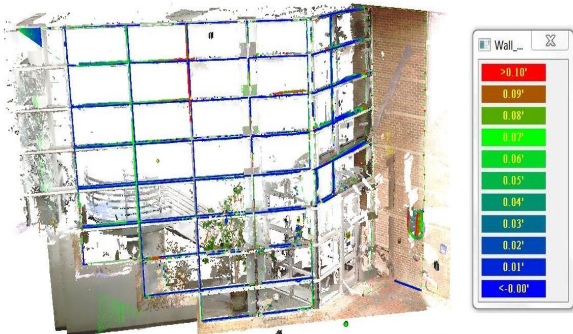
FIGURE 5: Heat mapping of the Cameron curtain wall
