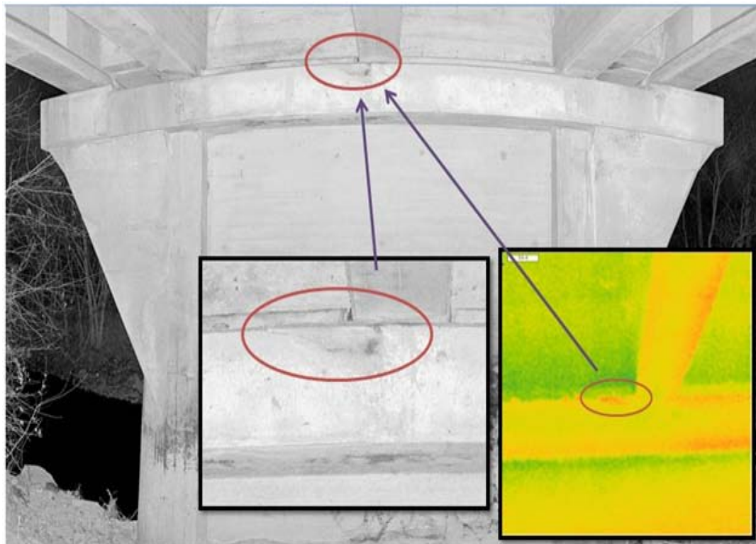
Figure 2-5 Bridge abutment defect detection from thermography (Bridge # 590049, NCDOT)
