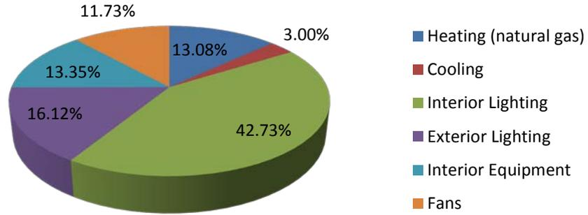
Figure 35: Los Angeles, CA strip mall lightweight concrete masonry model with expanded slate mortar annual energy consumption by end-use
