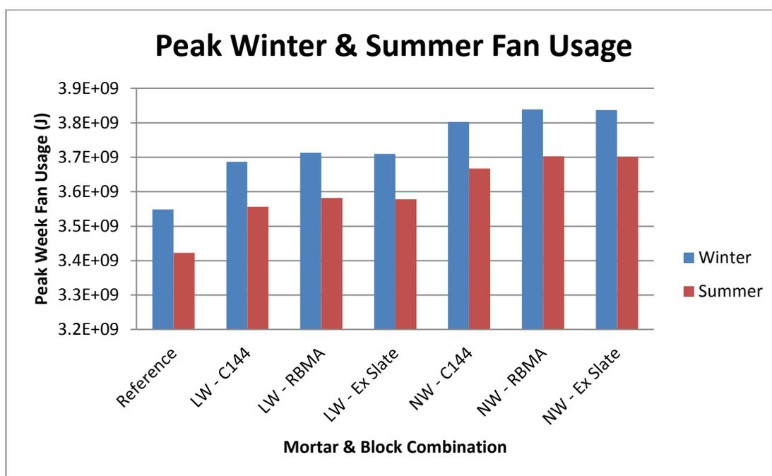
Figure 22: Miami, FL strip mall concrete masonry fan usage for peak summer and winter times
