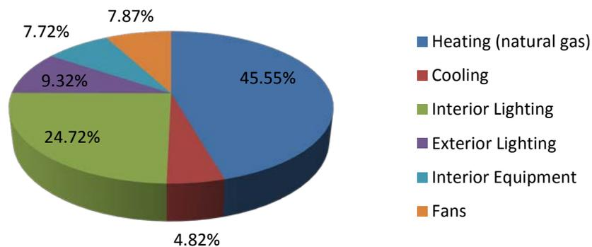
Figure 51: Baltimore, MD strip mall lightweight concrete masonry model with expanded slate mortar annual energy consumption by end-use
