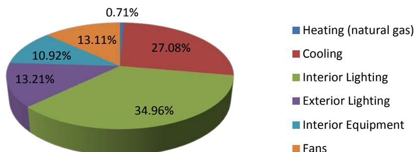
Figure 21: Miami, FL strip mall normal weight concrete masonry model with expanded slate mortar annual energy consumption by end-use
