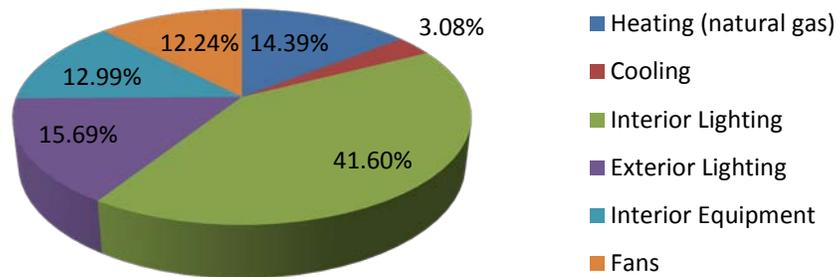
Figure 37: Los Angeles, CA strip mall normal weight concrete masonry model with expanded slate mortar annual energy consumption by end-use
