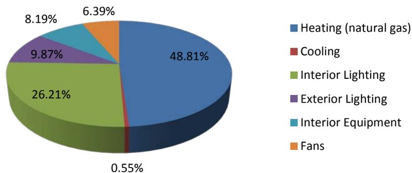
Figure 64: Seattle, WA strip mall lightweight C144 concrete masonry model annual energy consumption by end-use
