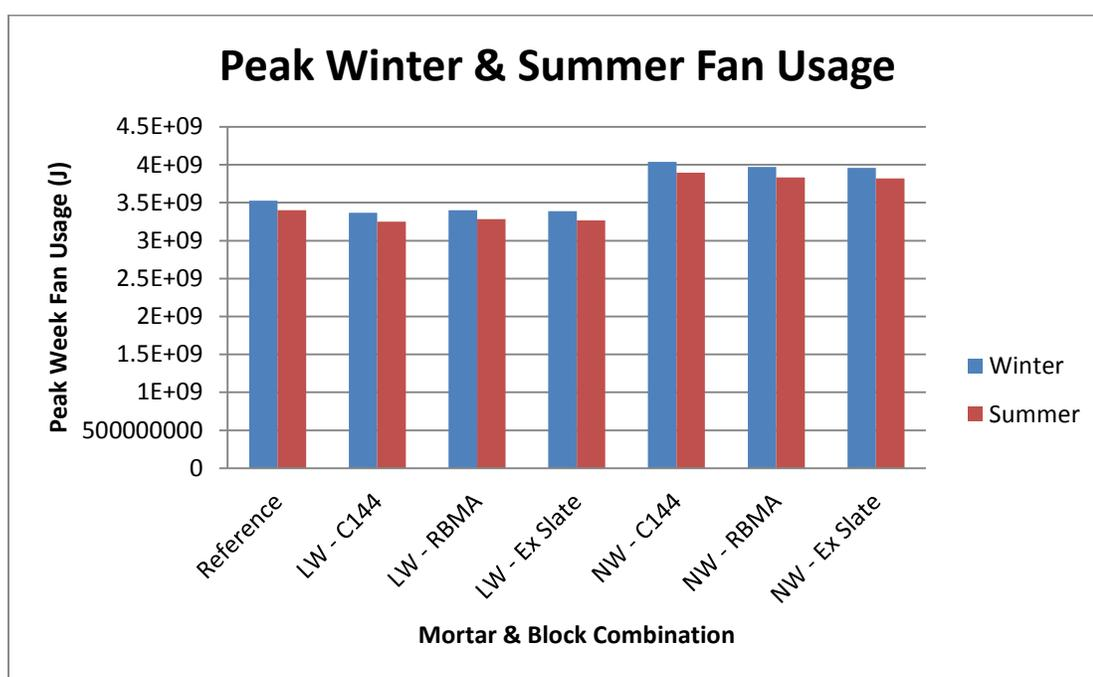
Figure 62: Phoenix, AZ strip mall concrete masonry model fan usage for peak summer and winter times
