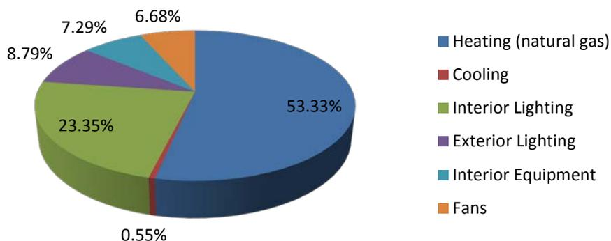
Figure 65: Seattle, WA strip mall normal weight C144 concrete masonry model annual energy consumption by end-use
