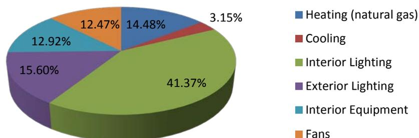
Figure 33: Los Angeles, CA strip mall normal weight C144 concrete masonry model annual energy consumption by end-use
