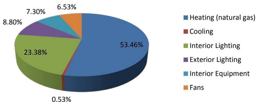
Figure 68: Seattle, WA strip mall normal weight concrete masonry model with RBMA mortar annual energy consumption by end-use
