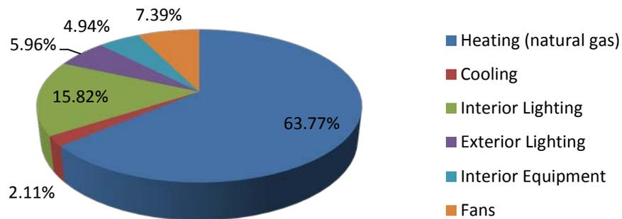
Figure 41: Minneapolis, MN strip mall normal weight C144 concrete masonry model annual energy consumption by end-use
