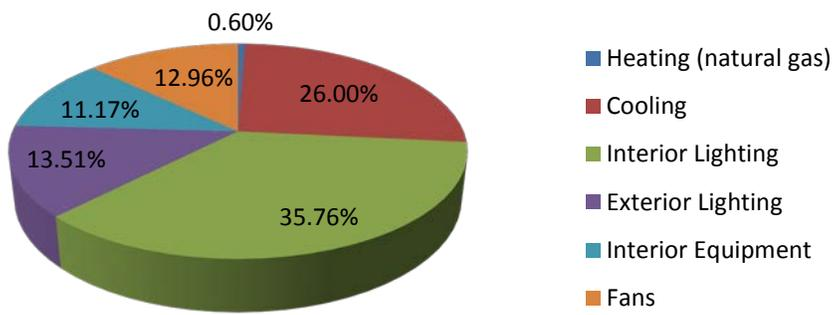
Figure 19: Miami, FL strip mall lightweight concrete masonry model with expanded slate mortar annual energy consumption by end-use
