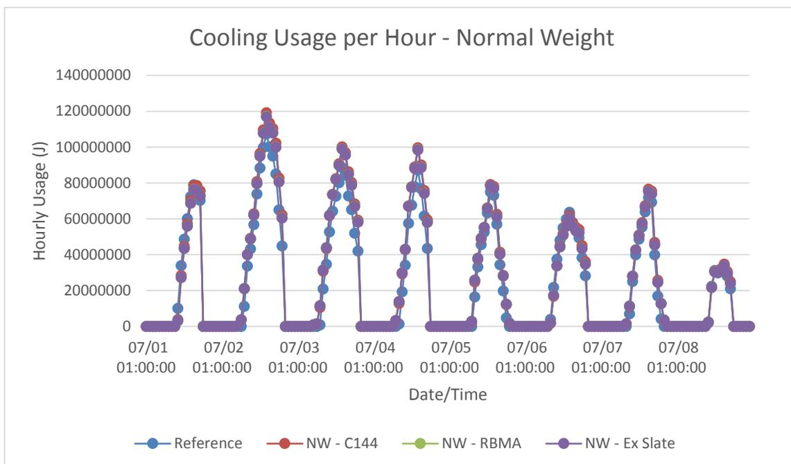
Figure B-8: Boulder, CO normal weight models hourly cooling energy consumption in summer
