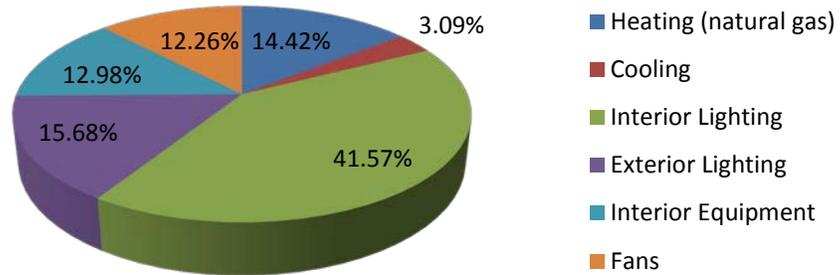
Figure 36: Los Angeles, CA strip mall normal weight concrete masonry model with RBMA mortar annual energy consumption by end-use
