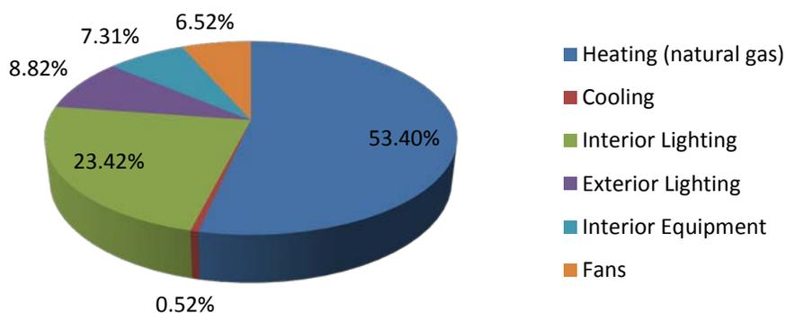
Figure 69: Seattle, WA strip mall normal weight concrete masonry model with expanded slate mortar annual energy consumption by end-use
