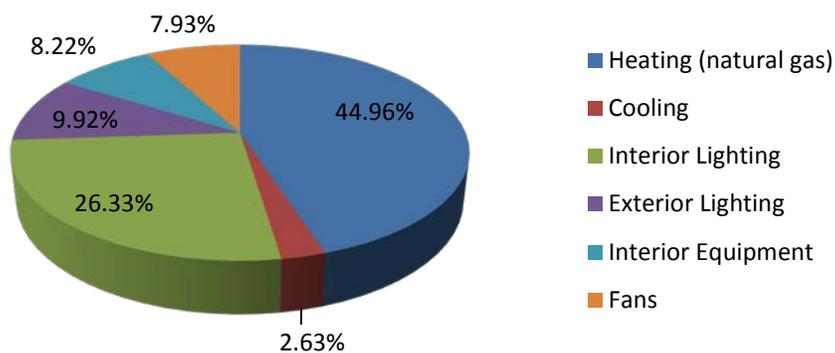
Figure 23: Boulder, CO strip mall DOE reference model annual energy consumption by end-use
