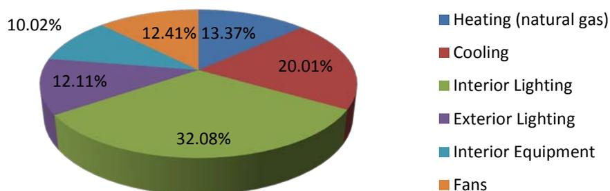
Figure 61: Phoenix, AZ strip mall normal weight concrete masonry model with expanded slate mortar annual energy consumption by end-use
