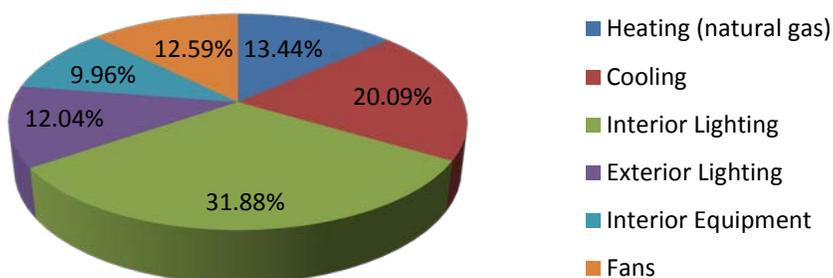
Figure 57: Phoenix, AZ strip mall normal weight C144 concrete masonry model annual energy consumption by end-use
