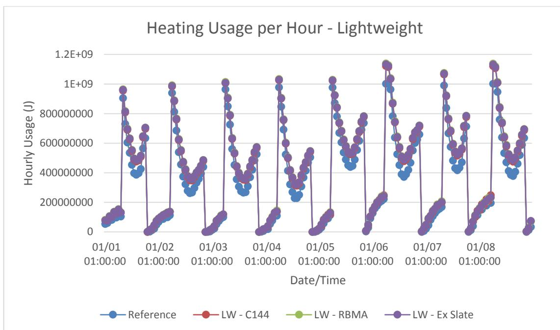
Figure 14: Boulder, CO heating usage per hour for lightweight concrete masonry models example graph
