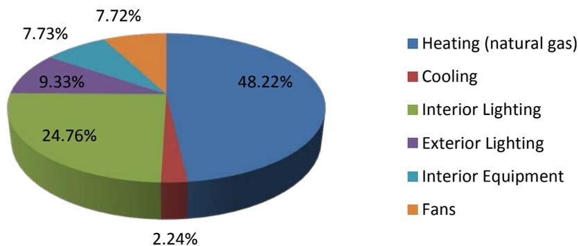
Figure 24: Boulder, CO strip mall lightweight C144 concrete masonry model annual energy consumption by end-use
