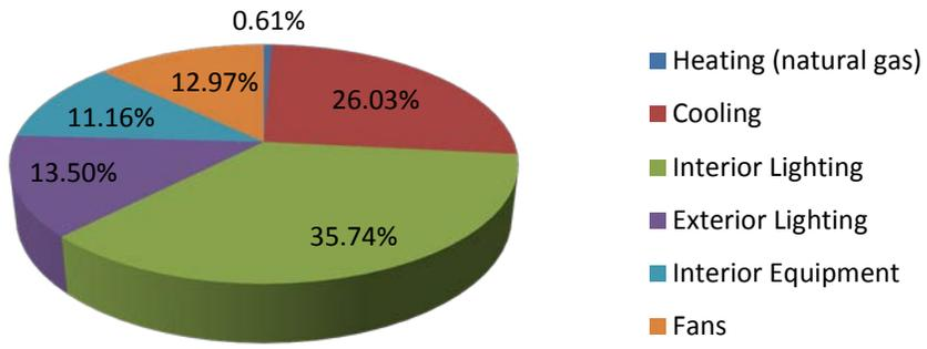
Figure 18: Miami, FL strip mall lightweight concrete masonry model with RBMA mortar annual energy consumption by end-use
