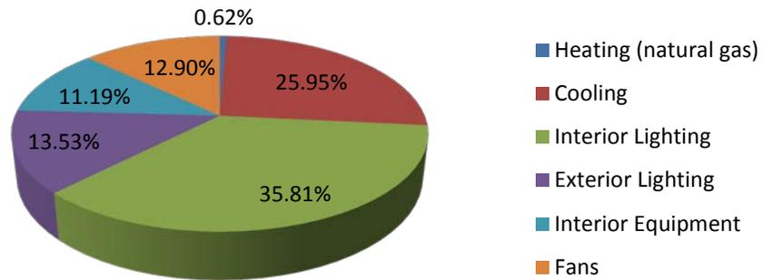
Figure 16: Miami, FL strip mall lightweight C144 concrete masonry model annual energy consumption by end-use
