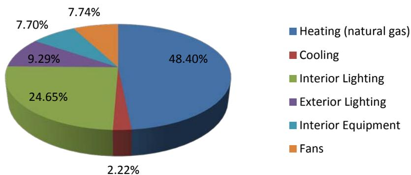
Figure 27: Boulder, CO strip mall lightweight concrete masonry model with expanded slate mortar annual energy consumption by end-use
