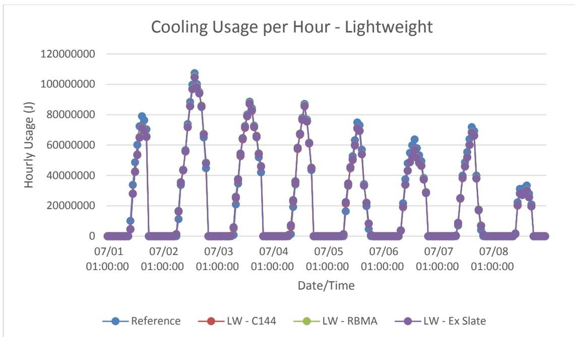
Figure B-7: Boulder, CO lightweight models hourly cooling energy consumption in summer
