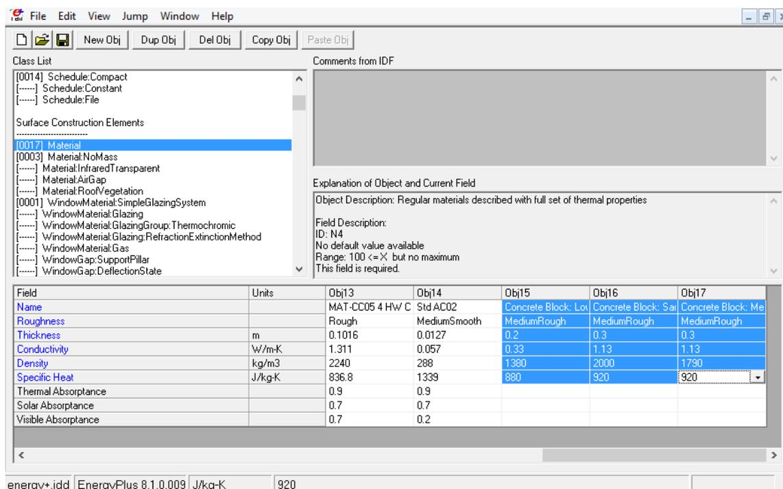
Figure 9: Importing concrete masonry into reference model
