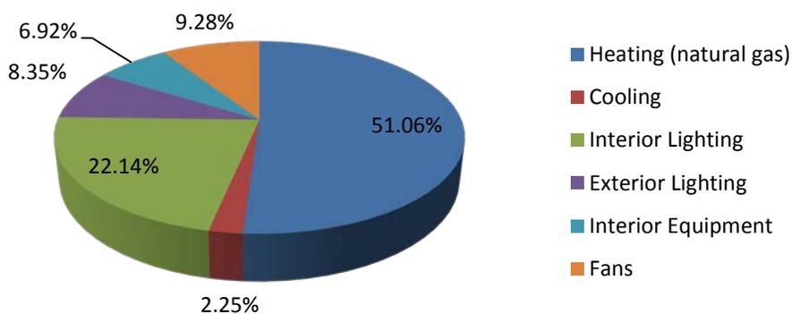
Figure 28: Boulder, CO strip mall normal weight concrete masonry model with RBMA mortar annual energy consumption by end-use
