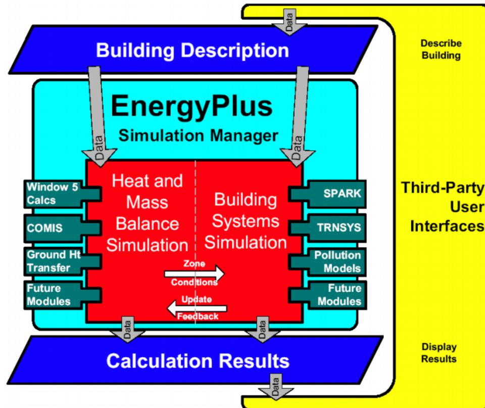
Figure 3: EnergyPlus simulation structure (Crawley et al., 2000)
