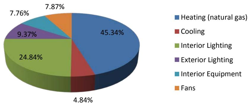
Figure 48: Baltimore, MD strip mall lightweight C144 concrete masonry model annual energy consumption by end-use
