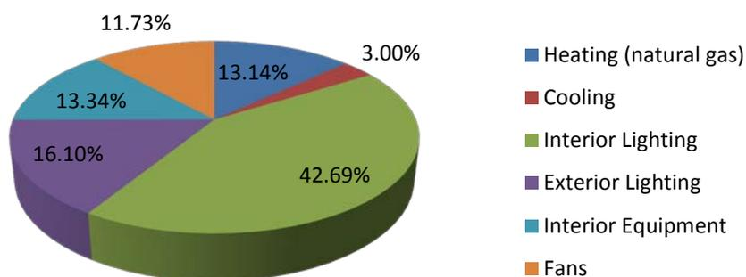
Figure 34: Los Angeles, CA strip mall lightweight concrete masonry model with RBMA mortar annual energy consumption by end-use
