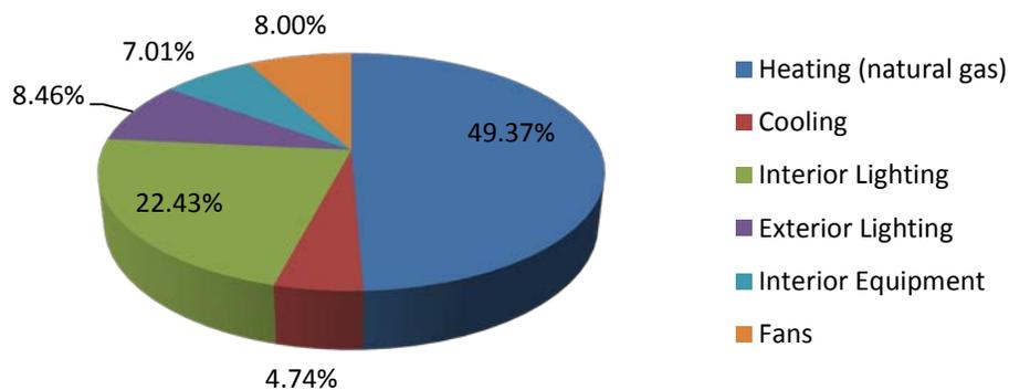
Figure 52: Baltimore, MD strip mall normal weight concrete masonry model with RBMA mortar annual energy consumption by end-use
