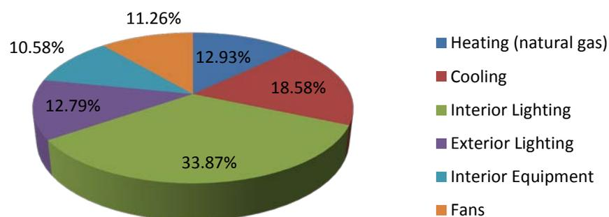
Figure 58: Phoenix, AZ strip mall lightweight concrete masonry model with RBMA mortar annual energy consumption by end-use
