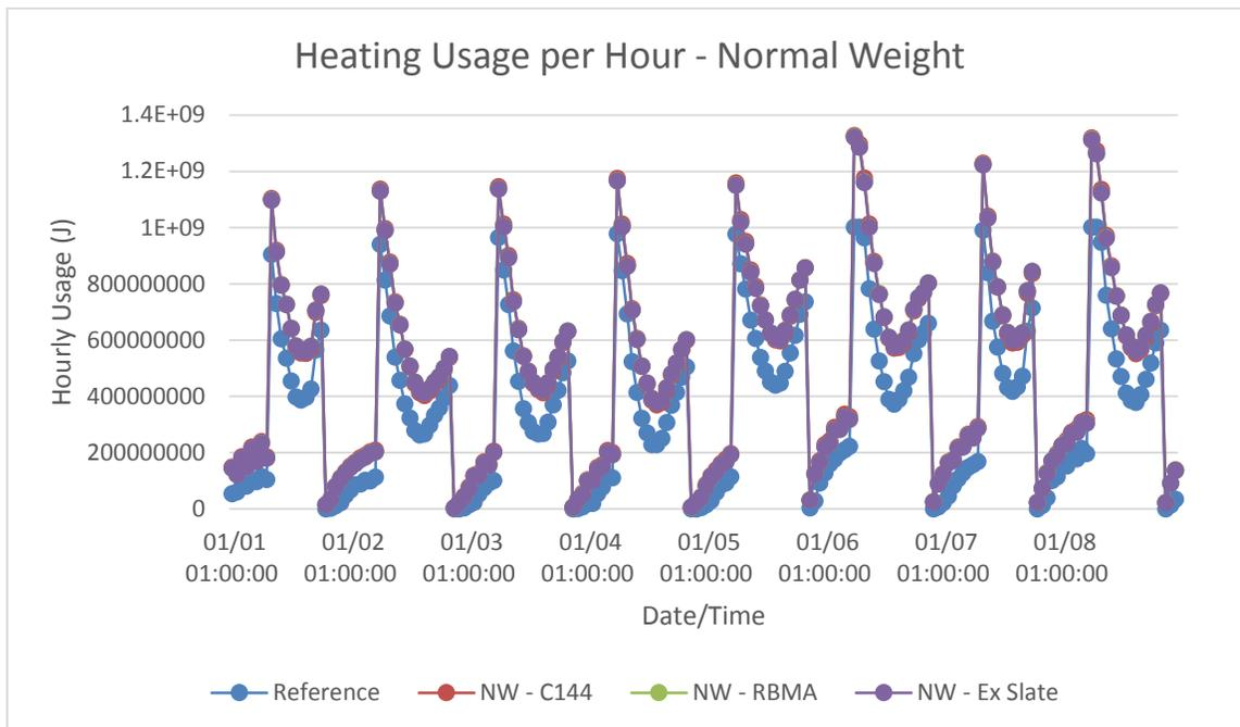
Figure B-6: Boulder, CO normal weight models hourly heating energy consumption in winter
