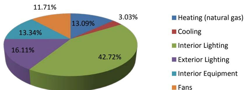
Figure 32: Los Angeles, CA strip mall lightweight C144 concrete masonry model annual energy consumption by end-use
