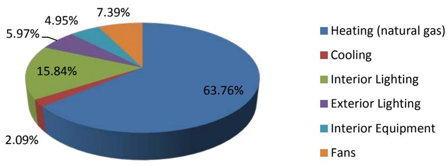
Figure 44: Minneapolis, MN strip mall normal weight concrete masonry model with RBMA mortar annual energy consumption by end-use
