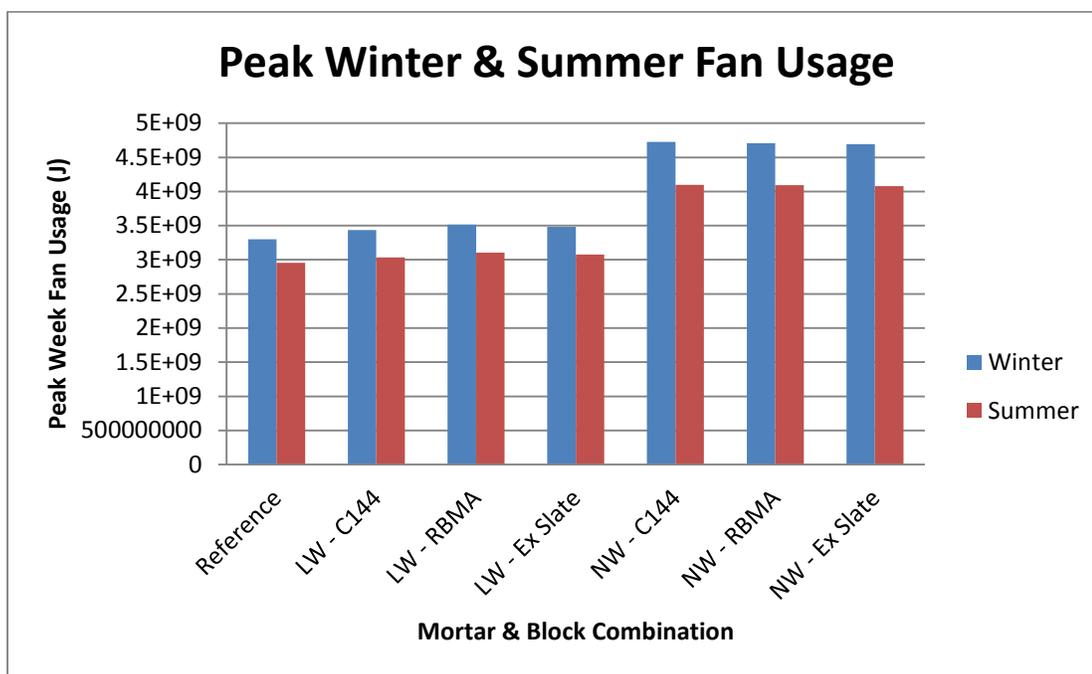
Figure 30: Boulder, CO strip mall concrete masonry model fan usage for peak summer and winter times
