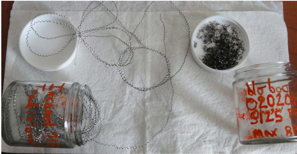
Figure 20: Inconel® 718 chip samples from traditional turning (left) and “Fine MTP” process (right).
