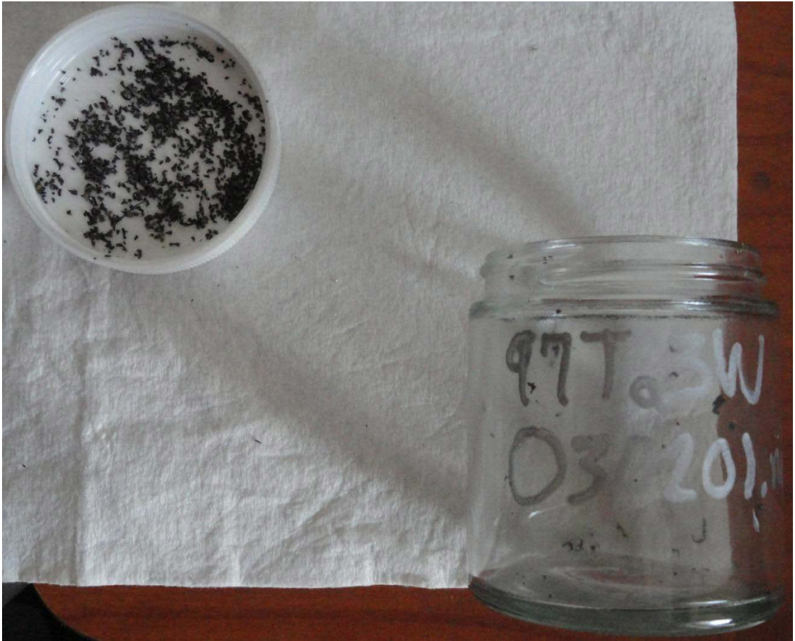
Figure 17: Chips from fine MTP process yielded very fine chips (CNC code O30201.nc).
