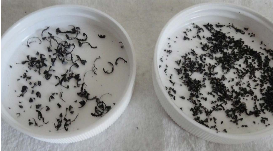
Figure 18: Tantalum chip samples from traditional turning (left) and “Fine MTP” process (right).
