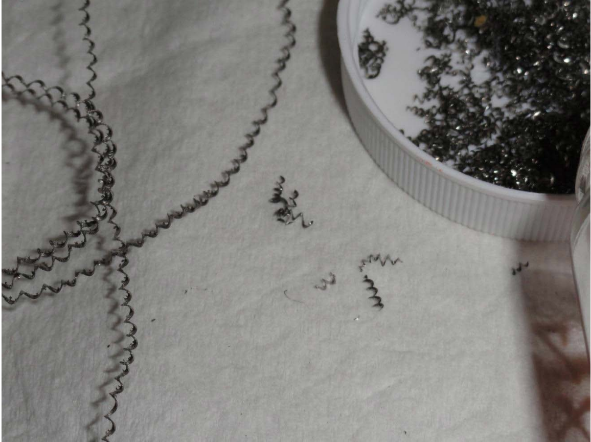
Figure 21: Closer examination of the Inconel® 718 chips comparing the continuous, coil-like chips from traditional turning (left) to the short segments of chips resulting from the use of the “Fine MTP” process (right).
