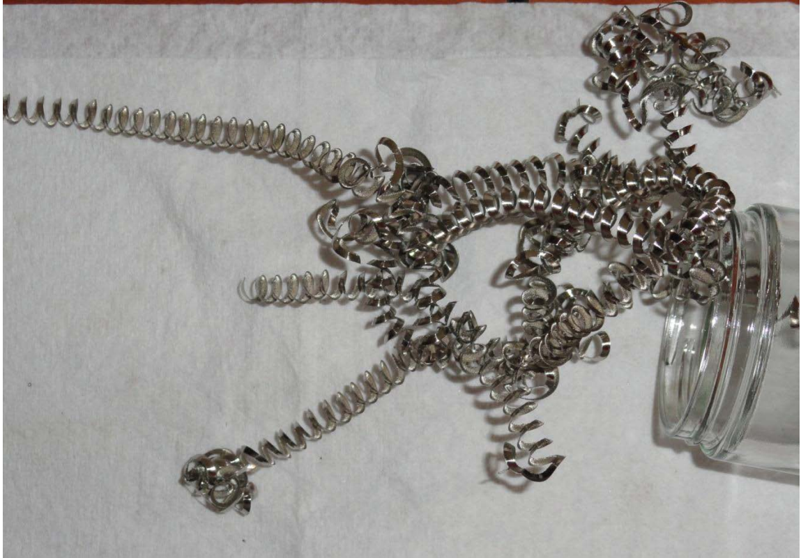
Figure 14: Tool steel M-42 coil-like chips resulting from traditional turning process.
