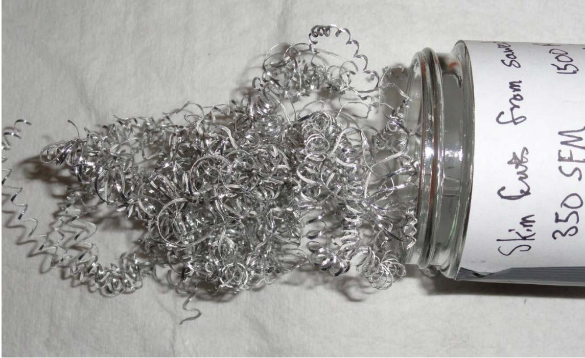
Figure 13: Entangled coil-like chips as a result of traditional turning process used on aluminum sample.
