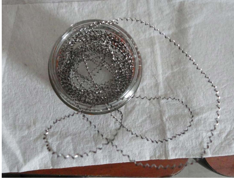
Figure 15: Image showing continuous coil-like chips of Inconel® 718 wound into glass container for storage (from tradition turning).
