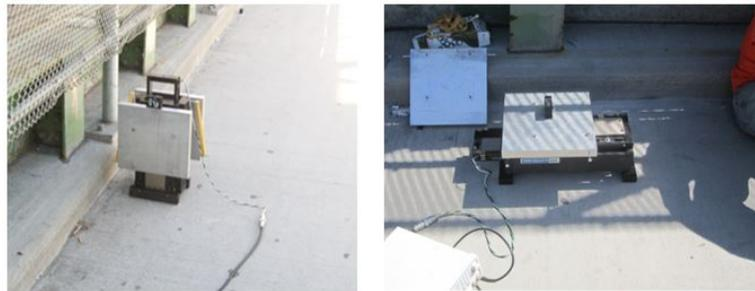
FIGURE 3.8: Mechanical shaker oriented to provide excitation in the vertical direction (left) and in the longitudinal direction (right)
