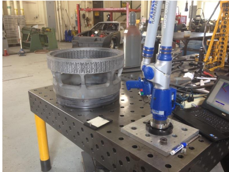
FIGURE 52: Exhaust measurement using an AACMM.
