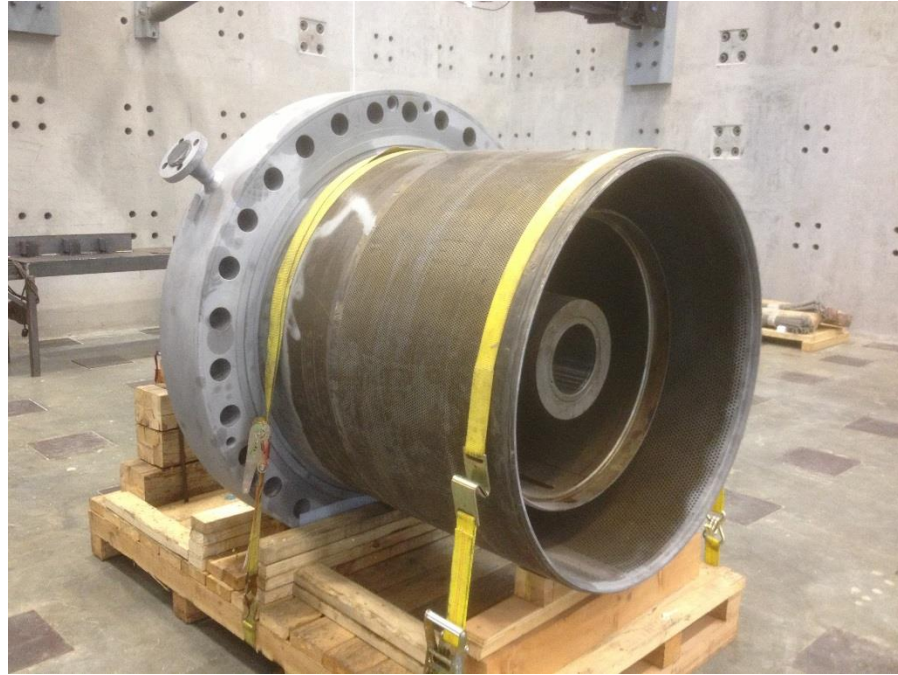
FIGURE 2: Steam turbine throttle valve.
