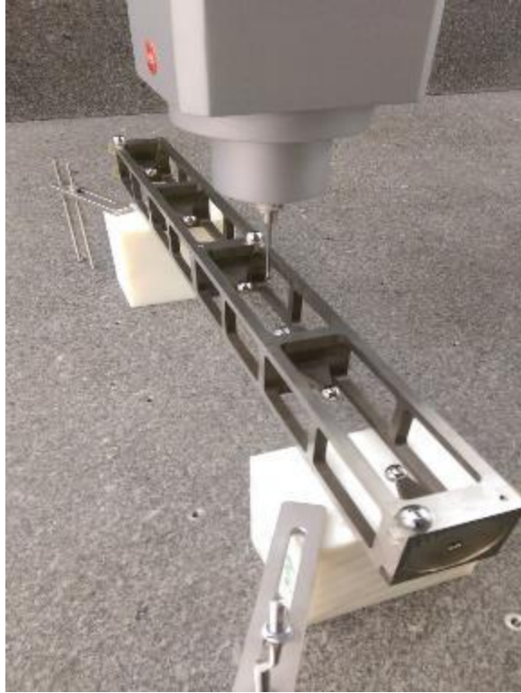
FIGURE 21: Invar ball-bar length gauge.
