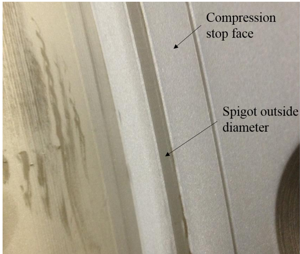
FIGURE 86: Spigot OD on throttle valve.
