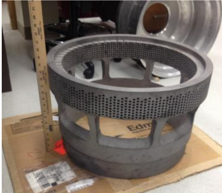
FIGURE 20: Steam turbine exhaust muffler.
