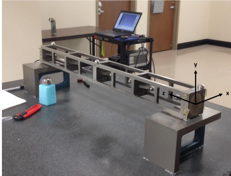
FIGURE 55: Ball-bar measurement setup.
