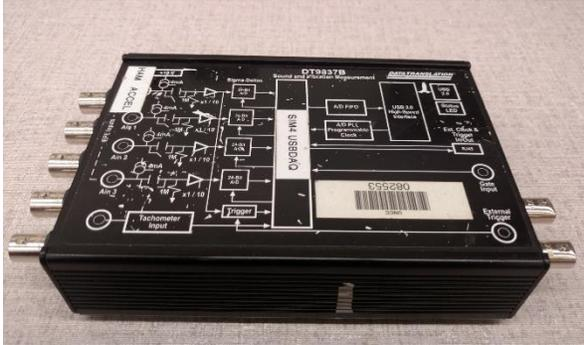
Figure 2-8 DT9837B DAQ module
