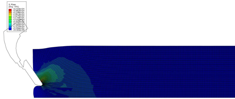
Figure 5.8: Soil deformation when the tool has traveled approximately 10 cm along the length of the soil block.
