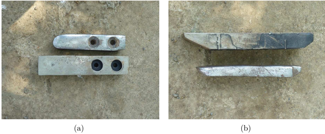
Figure 1.5: A comparison of an unworn tillage tool with a worn tillage tool, (a). top view, and (b). side view.
