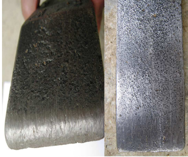
Figure 2.5: Two different views of a worn tillage tool surface from field tests.
