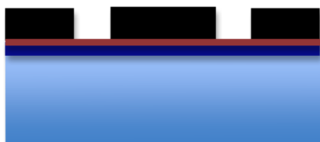
Step 3. Apply pattern and expose to UV Light
