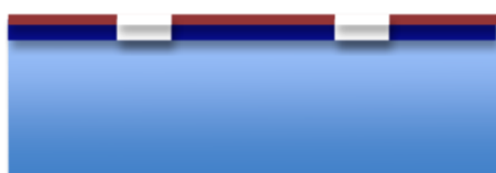
Step 5. Remove the SiO 2
