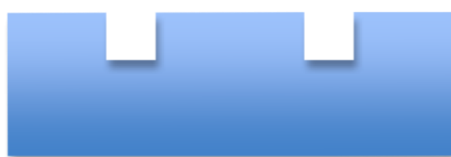
Step 7. Strip photo-resist and SiO 2
