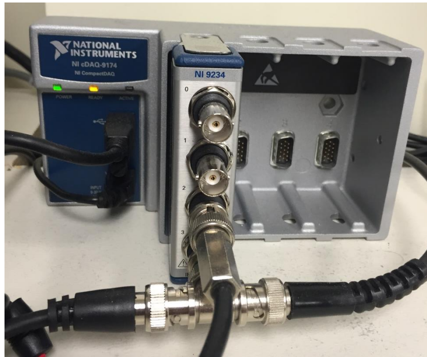
Figure 6: cDAQ and 4 channel module
