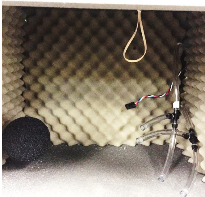
Figure 11: Foam test chamber
