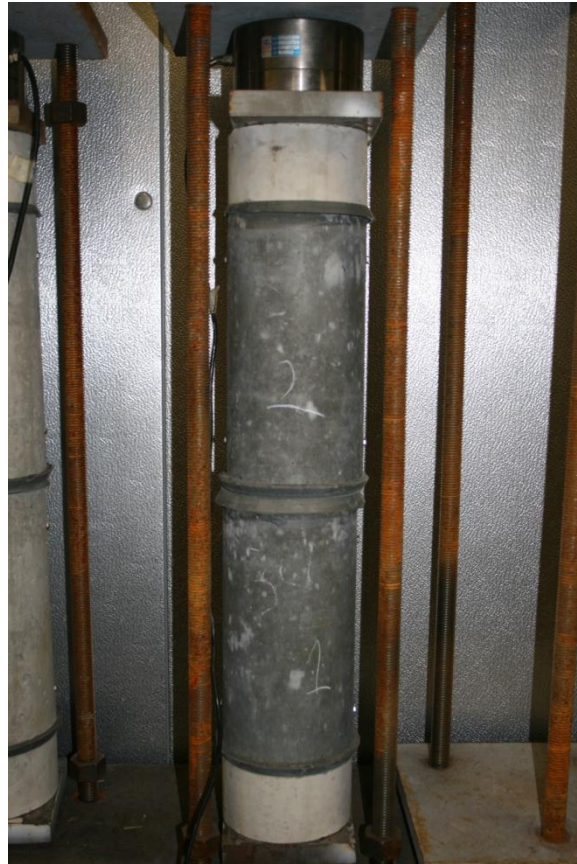
FIGURE 2-26: Creep specimen loading apparatus.
