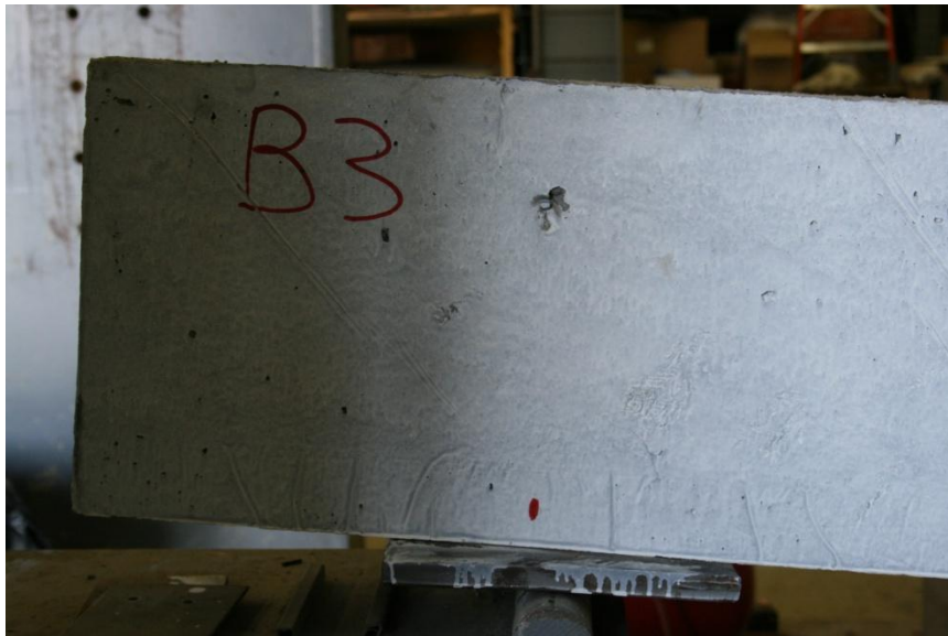
FIGURE 4-7: Support conditions for mild steel reinforced beams.
