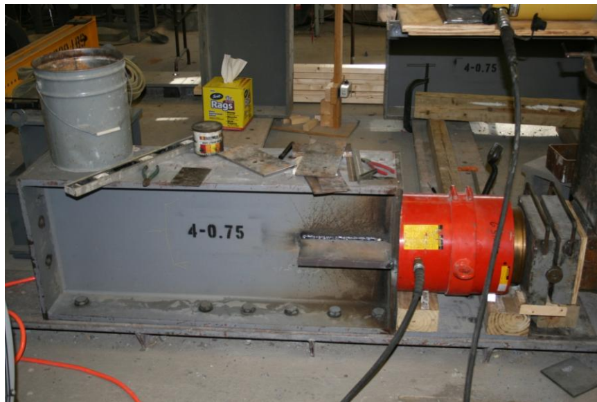
FIGURE 5-12: 4' abutment, primary axial load application piston and end roller.
