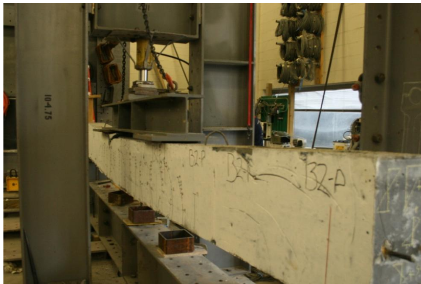
FIGURE 4-25: Prestressed beam loaded in the test frame.
