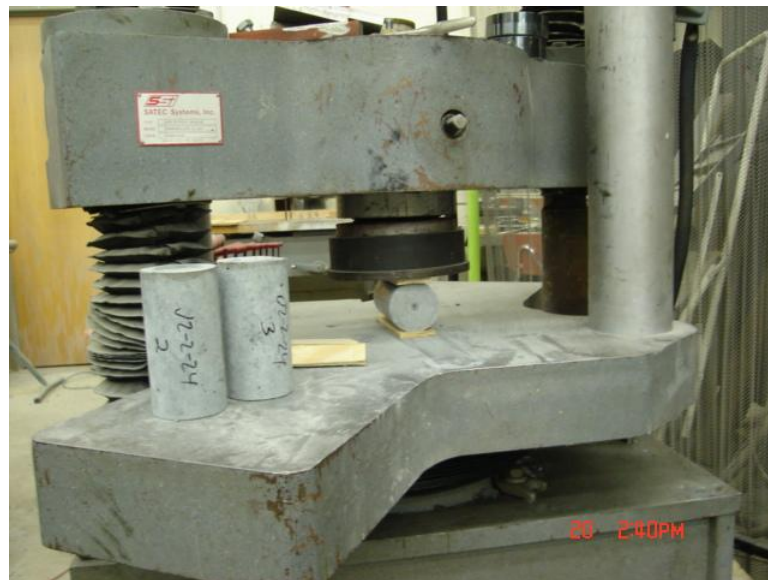
FIGURE 2-16: Splitting tensile test set-up.
