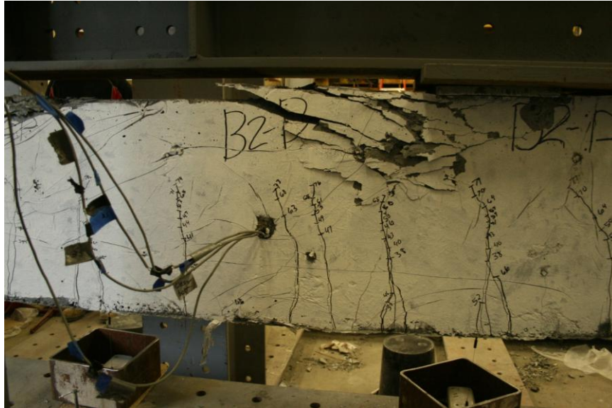
FIGURE 4-30: GCC-2-P1 beam failure by concrete crushing.
