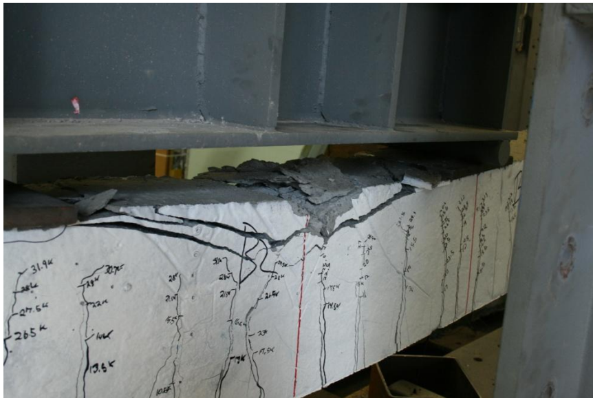
FIGURE 4-16: Crushing failure in GCC-2-B2.
