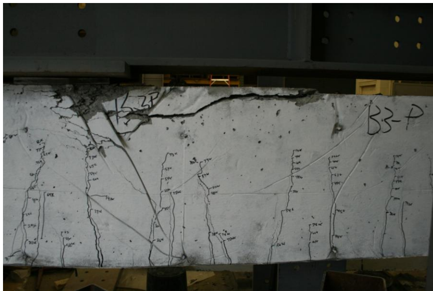
FIGURE 4-31: PCC-1-P2 beam failure by concrete crushing.
