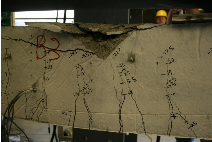
FIGURE 4-17: Crushing failure in PCC-1-B3.
