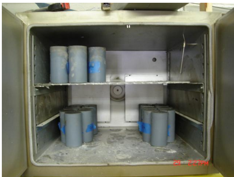
FIGURE 2-15: Oven for curing geopolymer concrete specimens.
