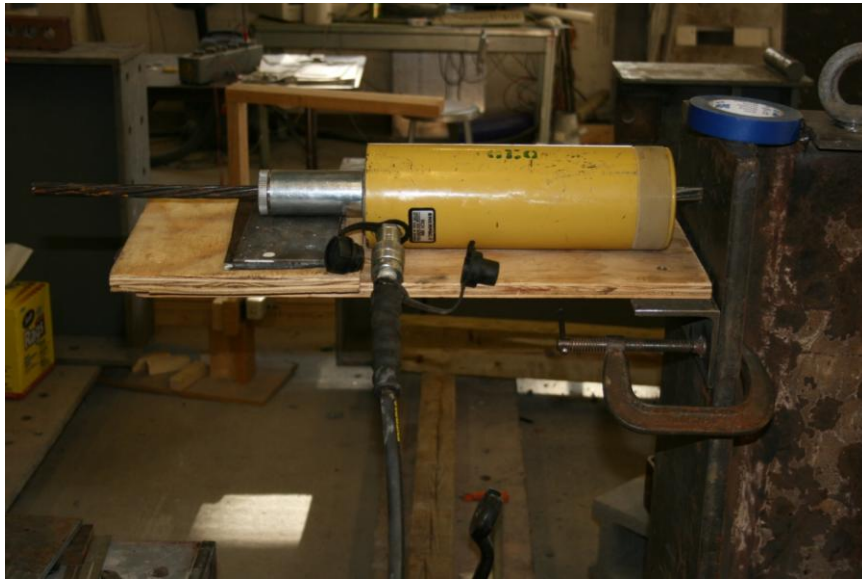
FIGURE 5-13: Application of P_2 with a 30 ton jack and prestressing strand.
