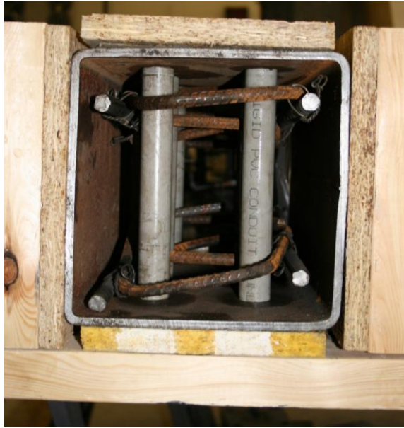
FIGURE 5-10: Reinforcing at the ends of the beam-columns.
