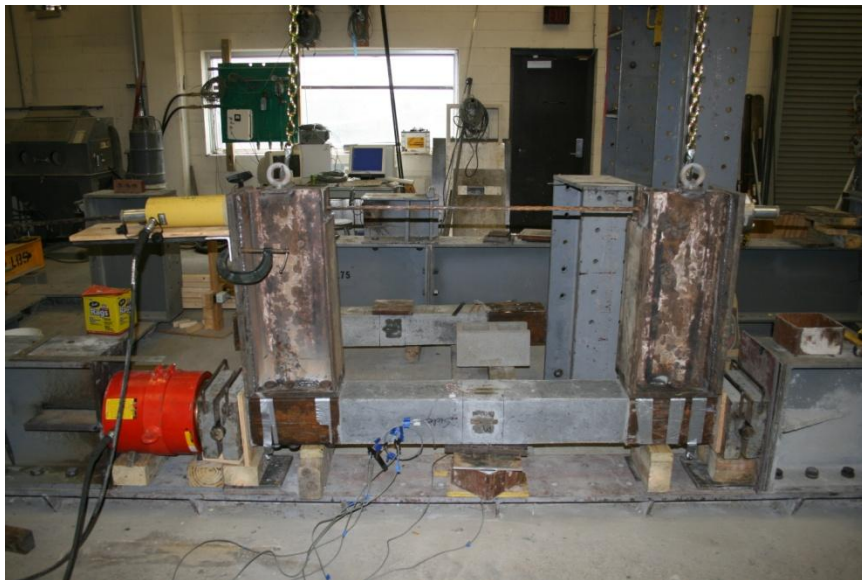
FIGURE 5-14: Full test set-up for flexural beam columns.
