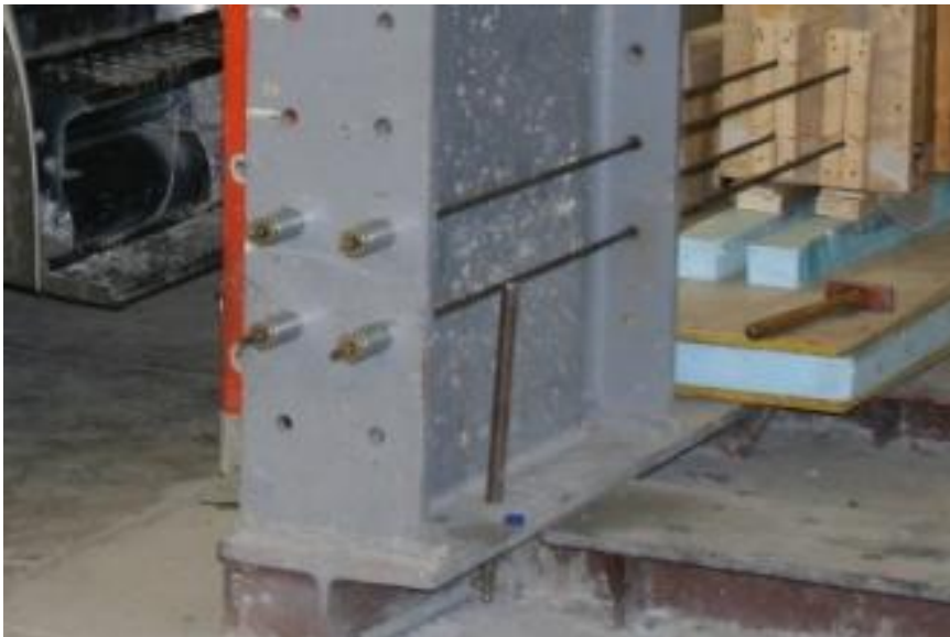
FIGURE 4-23: Prestressing tendons passing through the abutment.
