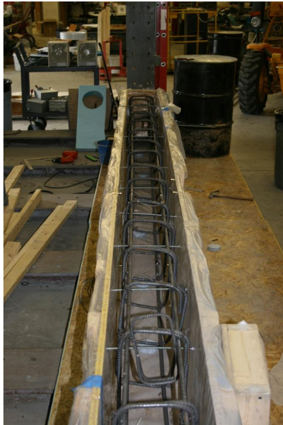
FIGURE 4-19: Reinforcing cage and prestressing tendons in formwork.
