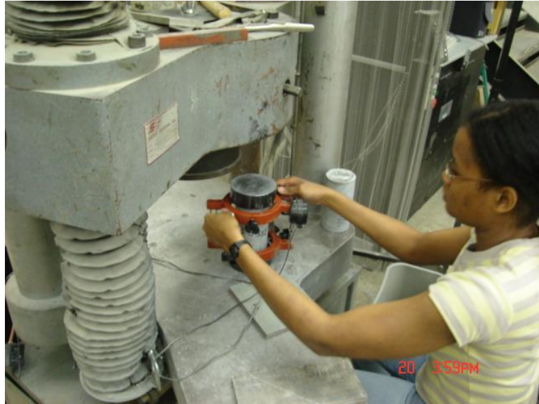
FIGURE 2-17: Static modulus of elasticity test set-up.
