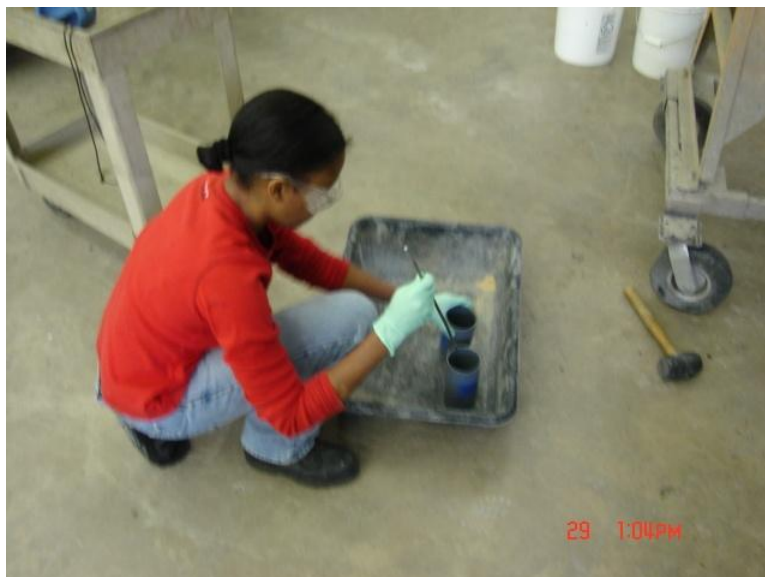
FIGURE 2-14: Consolidating geopolymer concrete in 3X6" cylinders.
