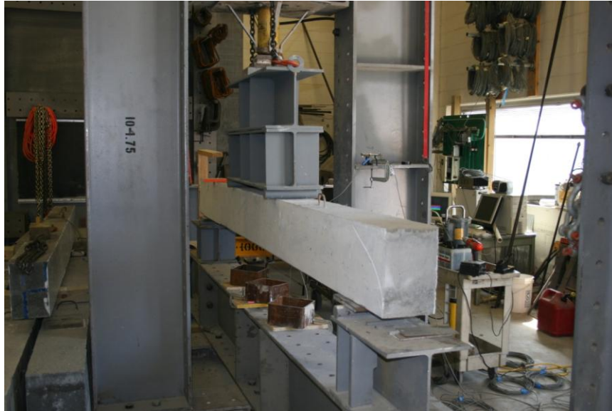
FIGURE 4-6: Mild steel reinforced beam loaded in the test frame.
