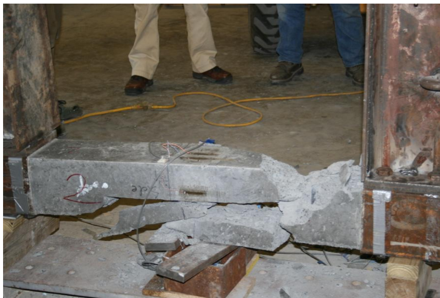
FIGURE 5-26: Failure of GCC-3-BC2.
