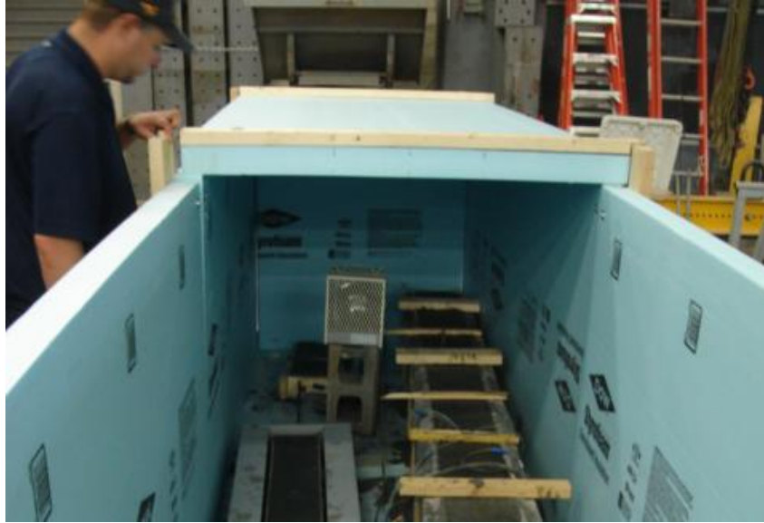
FIGURE 4-2: Beam and heater inside curing oven.
