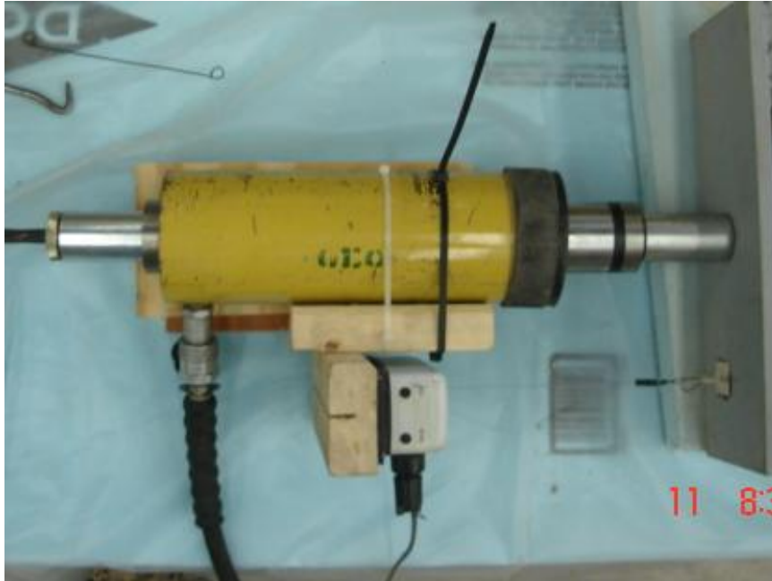
FIGURE 4-22: Jacking configuration used to tension prestressing tendons.
