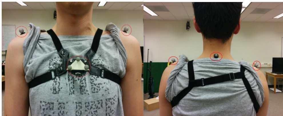
Figure 5.1 IMU placed on the sternum with triad attached to it and other markers on the upper body
