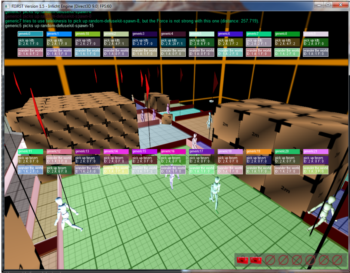
Figure 4.1: FI3RST contains multiple overlays to assist with AI debugging. Agent controllers are visualized as boxes, with color changes to indicate active layers. Flags in the world show agent waypoints. The navigation mesh is overlaid on the world terrain.
