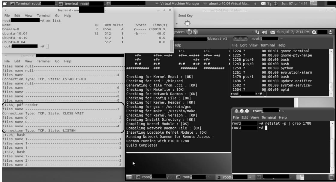
Figure 12: The detection of KBeast in Xen through cross-verification.
