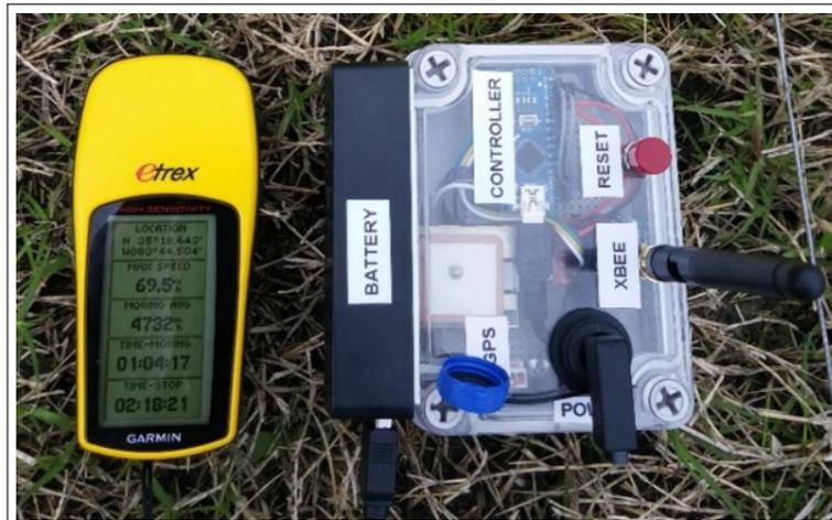
Figure 5.25: RSU Accuracy Check with Garmin GPS
