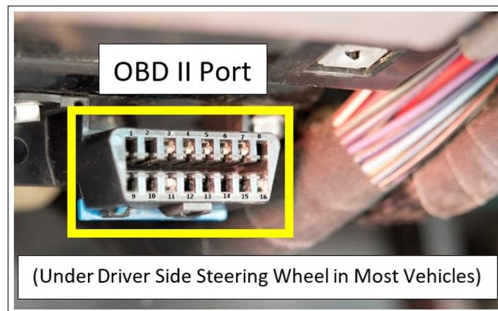
Figure 3.20: OBDII Port (On All Vehicles Produced after 1996) [82]
