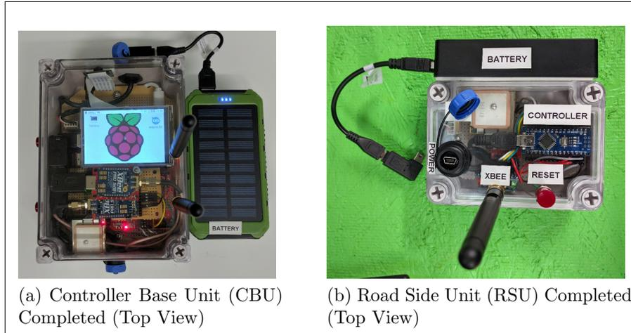
Figure 5.23: CBU and RSU Completed (Top View)
