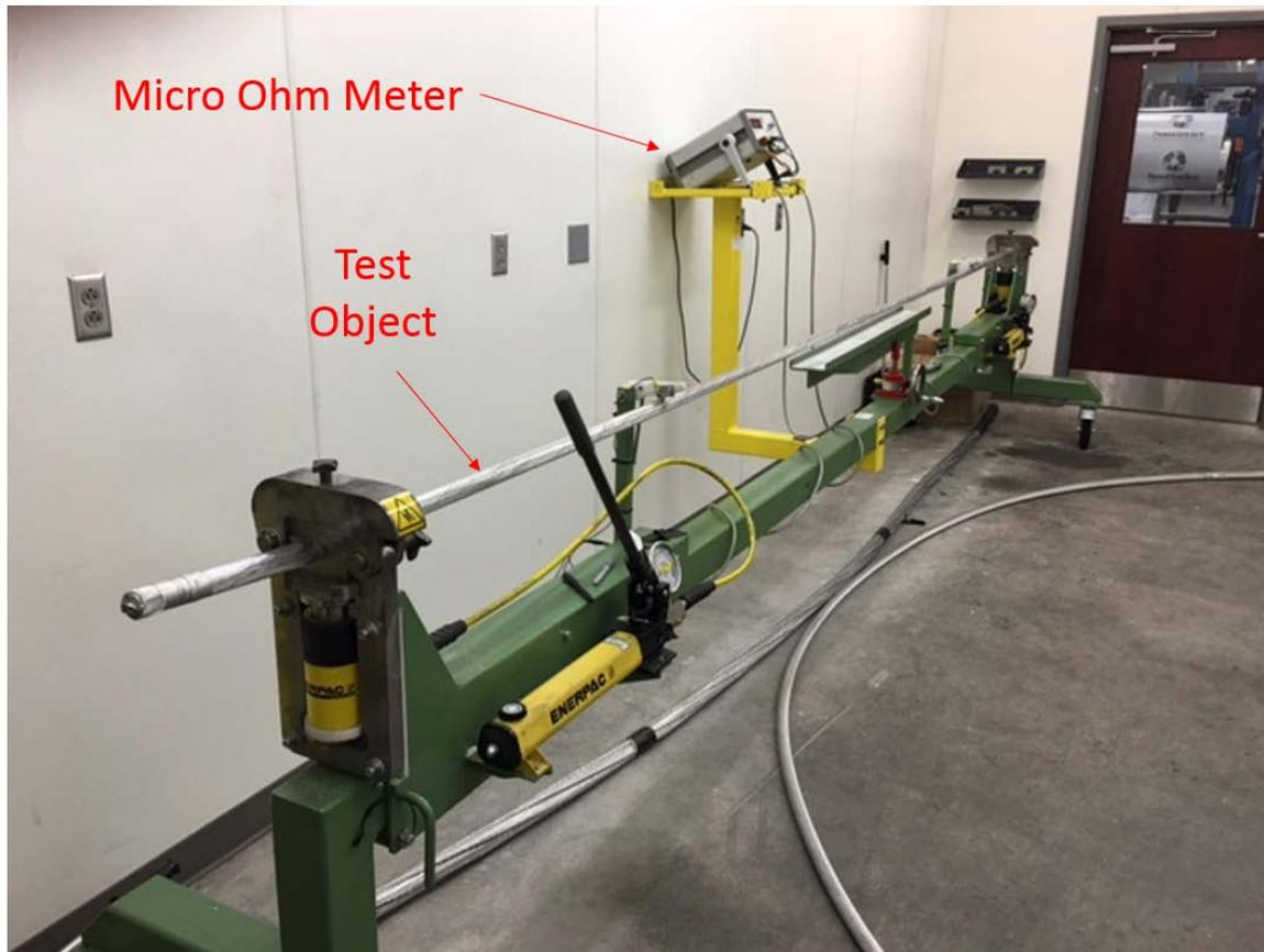
FIGURE 5-12: Picture of post-stranding DC resistance measurement setup
