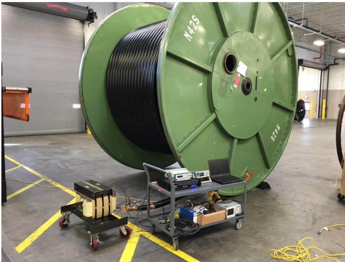
FIGURE 5-22: Equipment test setup of 2570 mm<sup>2</sup> conductor (steel reel)
