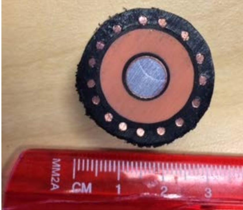
FIGURE 5-7: Picture of CCA test sample
