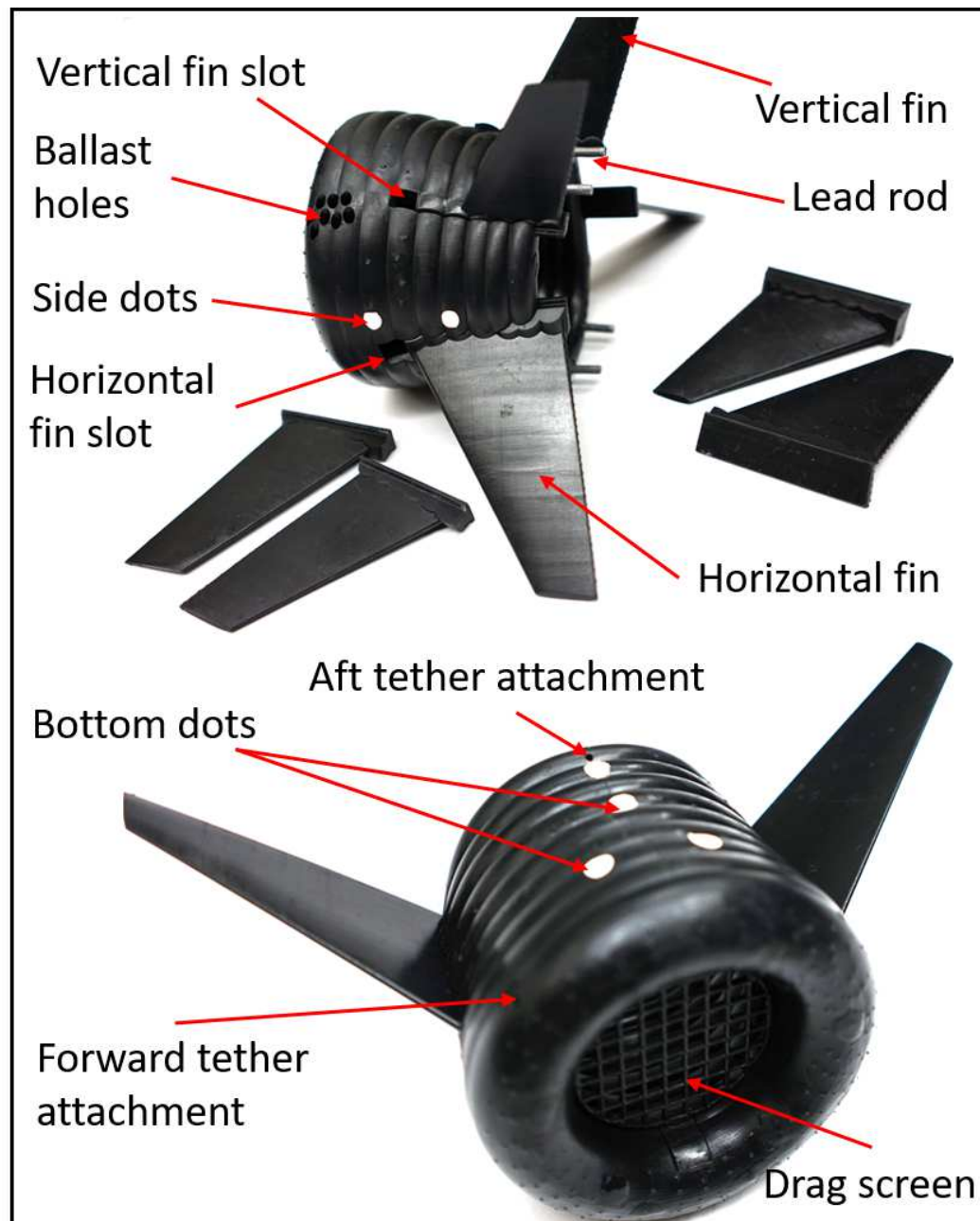
Figure 25: 3D printed representation of the BAT showing removable fin design, enabling rapid reconfiguration of plant geometry.
