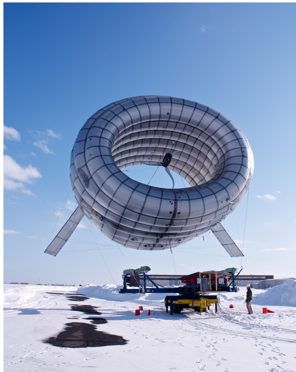
Figure 5: Full-scale prototype of Buoyant Airborne Turbine (BAT) during 2012 flight testing at Loring Air Force Base. (altaerosenergies.com)
