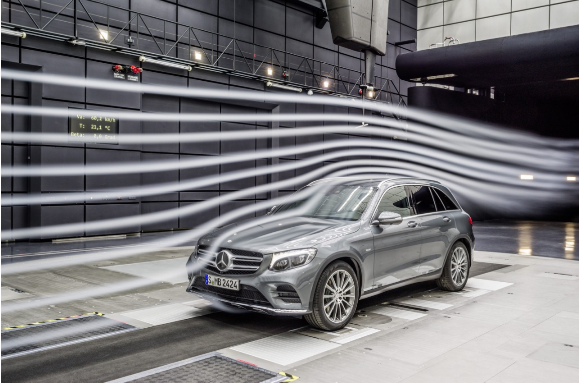
Figure 1.1: Smoke visualization in a wind tunnel testing [1].
