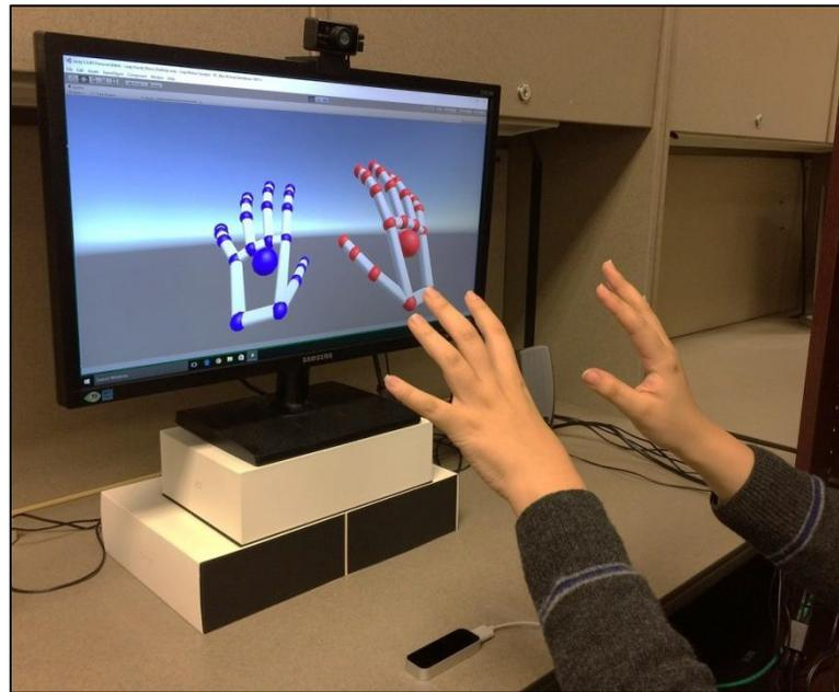
Figure 1.1: Hand and finger tracking using Leap Motion controller.
