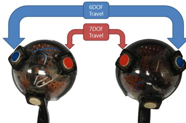
Figure 5.4: The buttonball devices with Fastrak trackers fixed inside.
