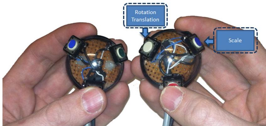
Figure 4.2: A pair of the buttonball devices. Each buttonball has three buttons on its surface and a Fastrak receiver inside of the ball to track the user's hand position.
