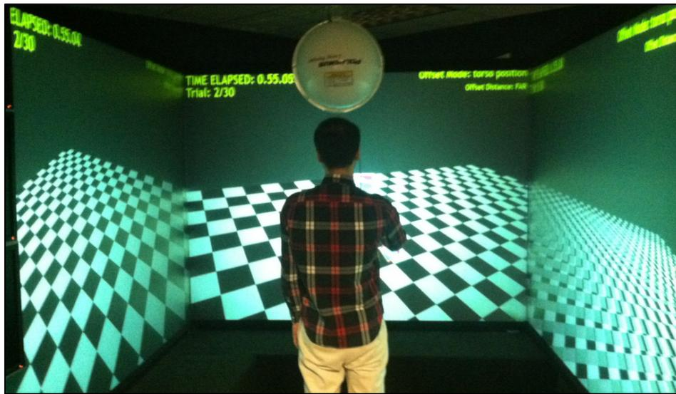
Figure 4.1: Our three-side CAVE system. Polhemus Fastrak tracks the position and orientation of the user's head and 3D input.
