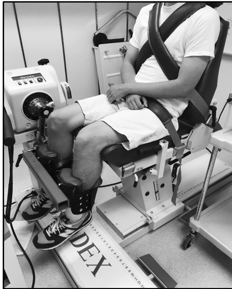
Figure 3: Depicting the modified single limb knee extension/flexion attachment for bilateral knee IET.
