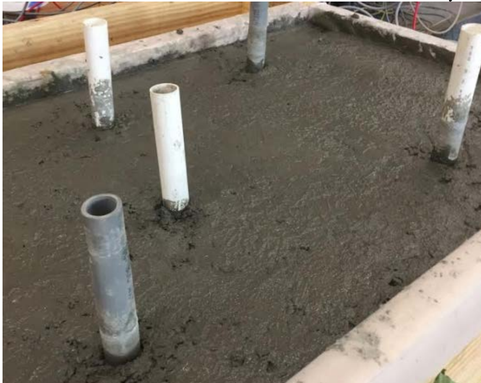
Figure 6.6: Laboratory test slab with PVC tubes after placement
