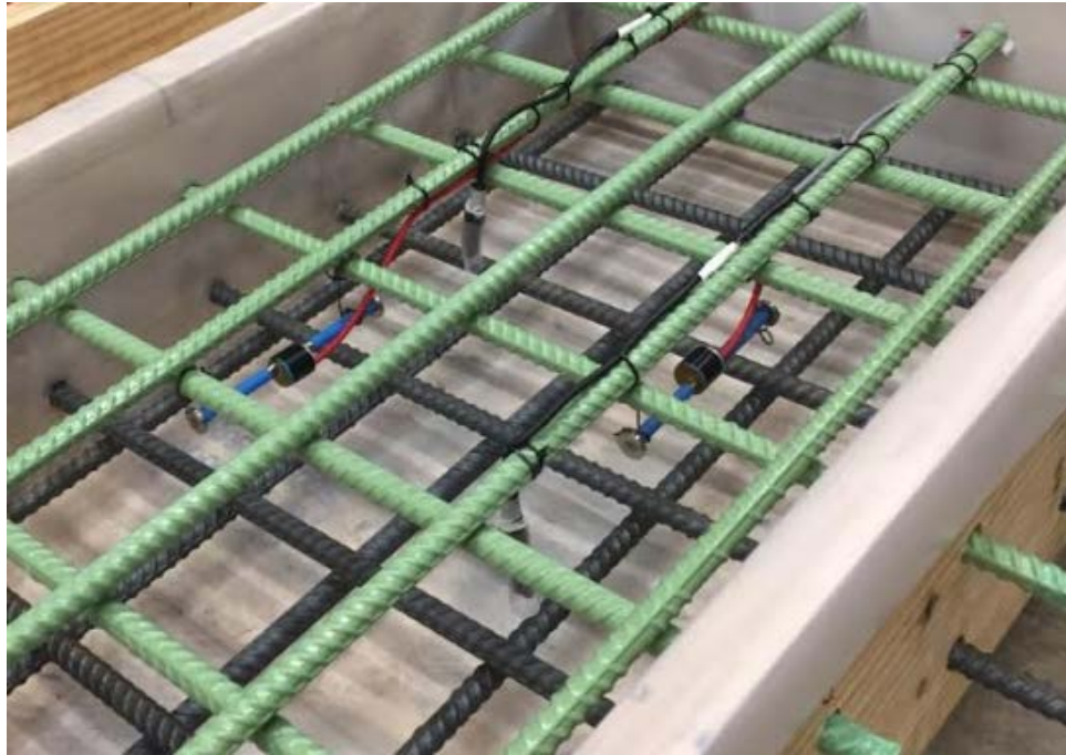
Figure 6.5: Formwork, rebar and embedded instrumentation for laboratory test slab
