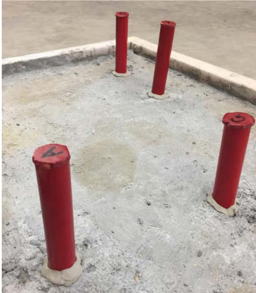
Figure 6.7: Wooden Dowels Placed Within Laboratory Test Slab
