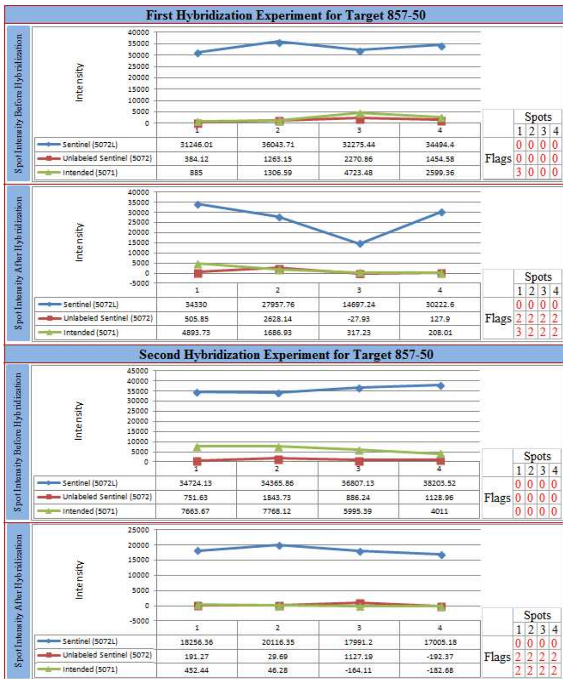
FIGURE 16: This figure summarizes the result of two hybridization experiments for target 857-50 and contains 1) plots of spot intensities before and after hybridization, 2) the intensity values for each spot located in a table at the bottom of each graph, and 3) spot quality flags which are located in a table at the bottom right corner of each graph. In the spot quality table, flag 0 means the spot has good quality, flag 2 means empty spots and flag 3 means poor quality spots.
