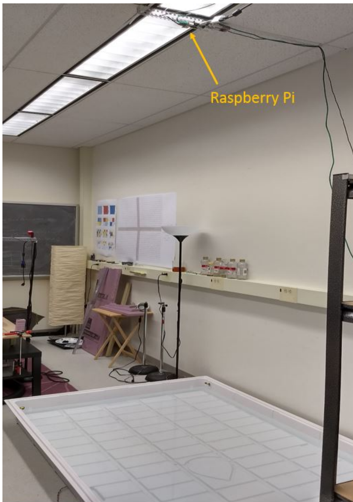
Figure 4.5: Pool test section with the Raspberry Pi mounted over it.
