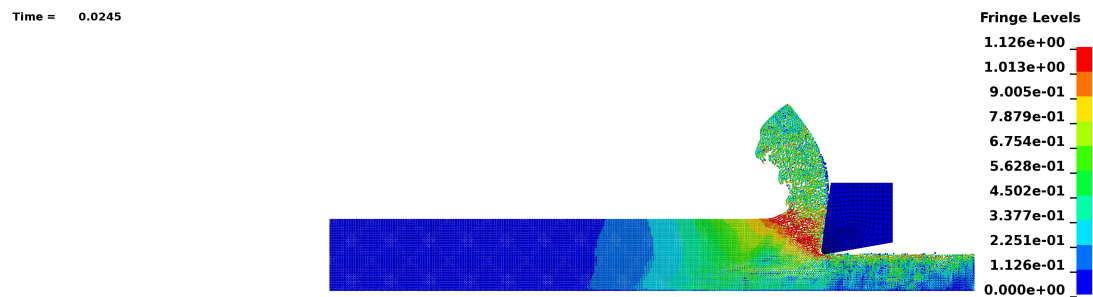
Figure 5.13: Contour plot of von Mises stress (GPa) for various depths of cut at time t = 0.0245 ms.
