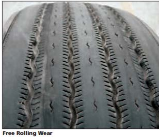
Figure 2.23 Free rolling wear [22]
