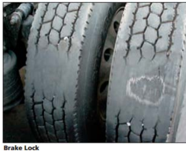
Figure 2.26 Flat spot wear [22]
