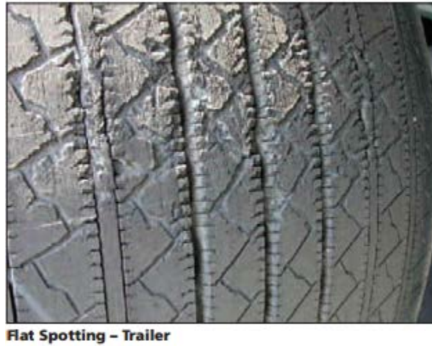
Figure 2.27 Flat spot wear [22]
