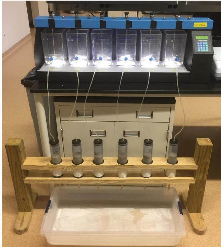
Figure 3.2. Jar test instrument with filtration apparatus.
