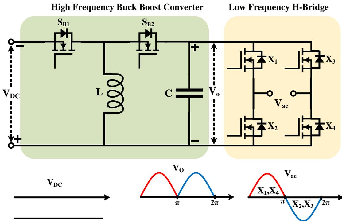
Figure 3.2: Microinverter schematic and operating principle
