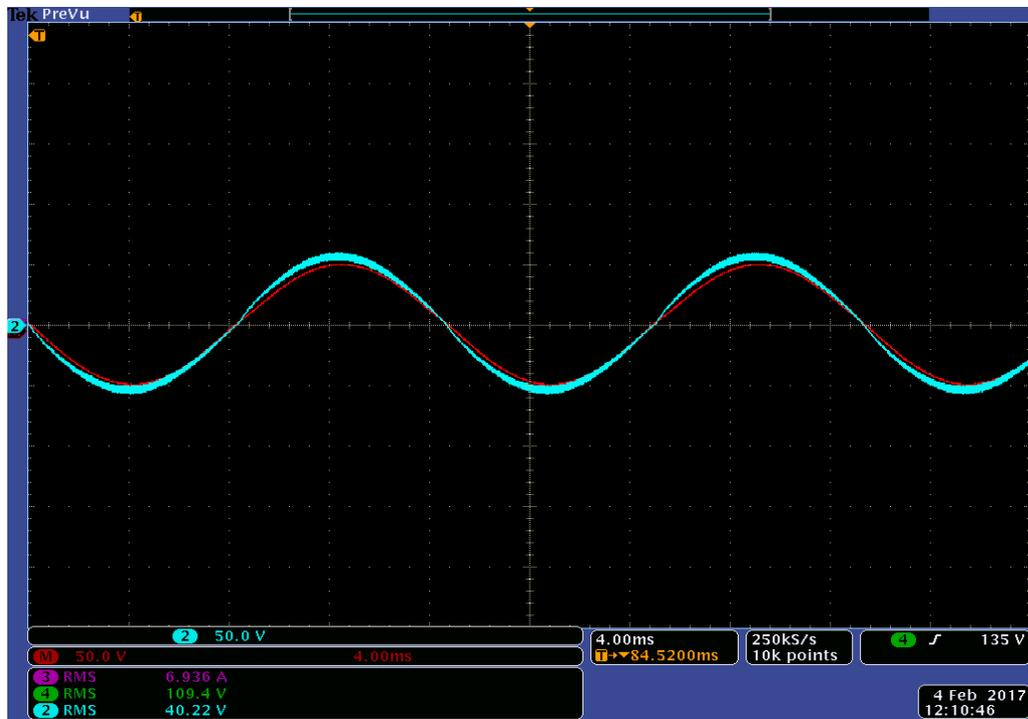
Figure 7.72: Experimental results of AC-DVR voltage  $V_{AC-DVR}$  (Blue) and DVR reference voltage  $V_{Ref-DVR}$  (Red) for experiment scenario XI
