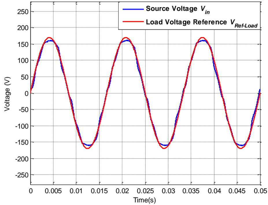
Figure 6.50: Source voltage  $V_{in}$  and load reference voltage  $V_{Ref-Load}$  for operating scenario XIII
