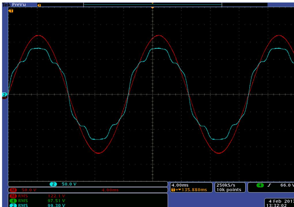
Figure 7.76: Experimental results of Source voltage  $V_{in}$  (Blue) and load reference voltage  $V_{Ref-Load}$  (Red) for experiment scenario XII
