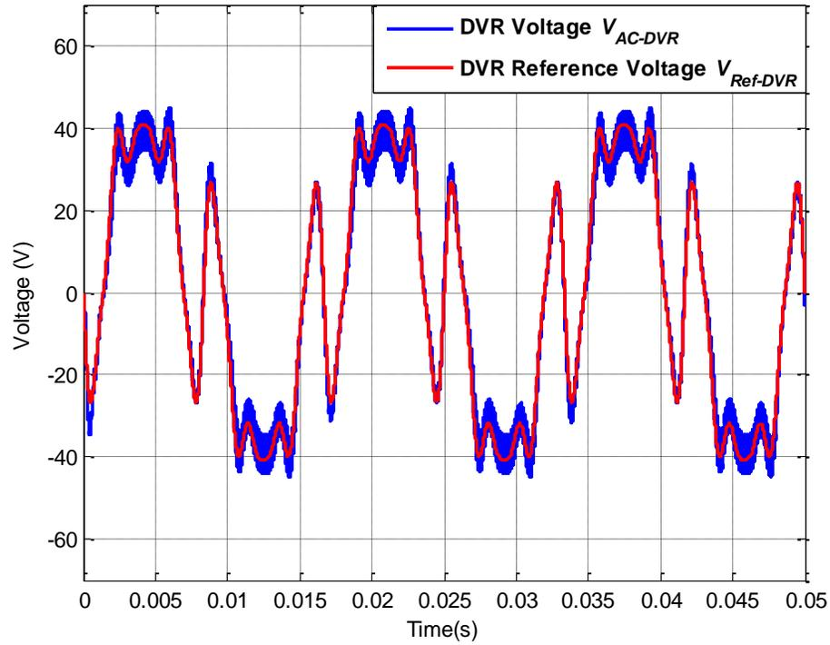
Figure 6.48: AC-DVR voltage  $V_{AC-DVR}$  and DVR reference voltage  $V_{Ref-DVR}$  for operating scenario XII
