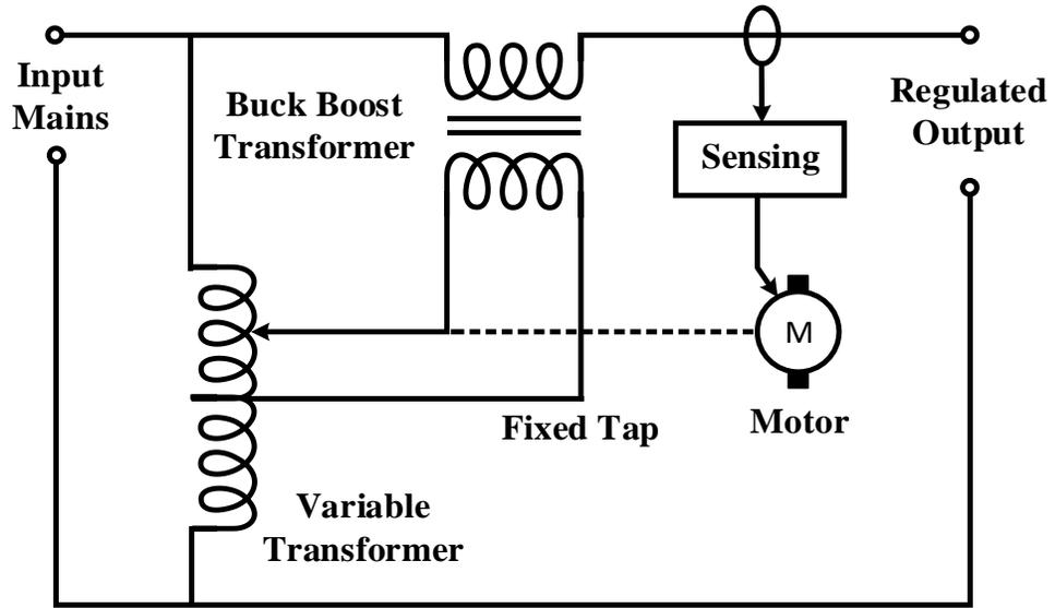
Figure 2.12: Servo Voltage Regulator
