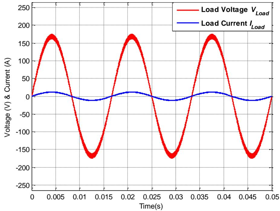
Figure 6.41: Load voltage  $V_{Load}$  and load current  $I_{Load}$  for operating scenario X
