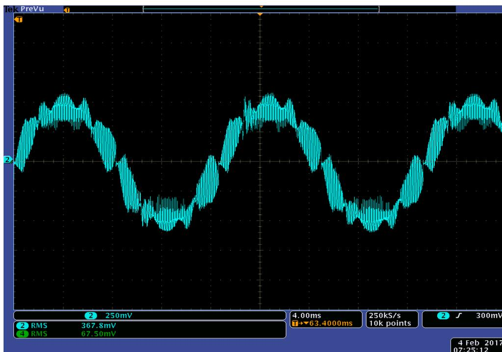
Figure 7.50: Experimental Results of Actual inductor current  $I_L$  for experiment scenario VIII
