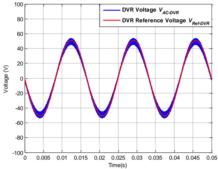
Figure 6.44: AC-DVR voltage  $V_{AC-DVR}$  and DVR reference voltage  $V_{Ref-DVR}$  for operating scenario XI
