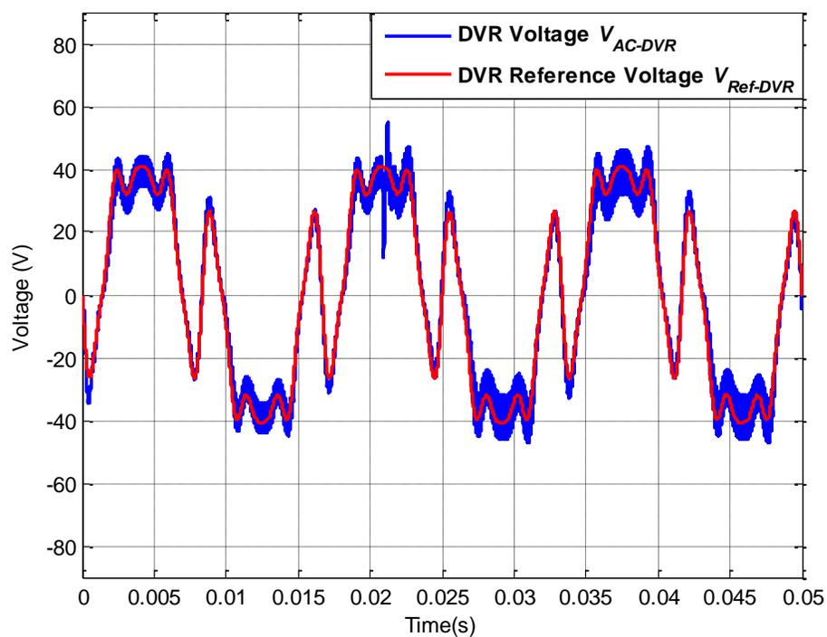
Figure 6.66: AC-DVR voltage  $V_{AC-DVR}$  and DVR reference voltage  $V_{Ref-DVR}$  for operating scenario XV
