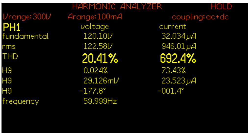
Figure 7.103: THD-5<sup>th</sup> of source voltage  $V_{in}$  for experiment scenario XVII
