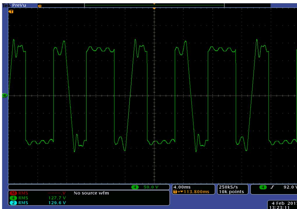
Figure 7.55: Experimental results of Bridge output voltage  $V_o$  for experiment scenario IX
