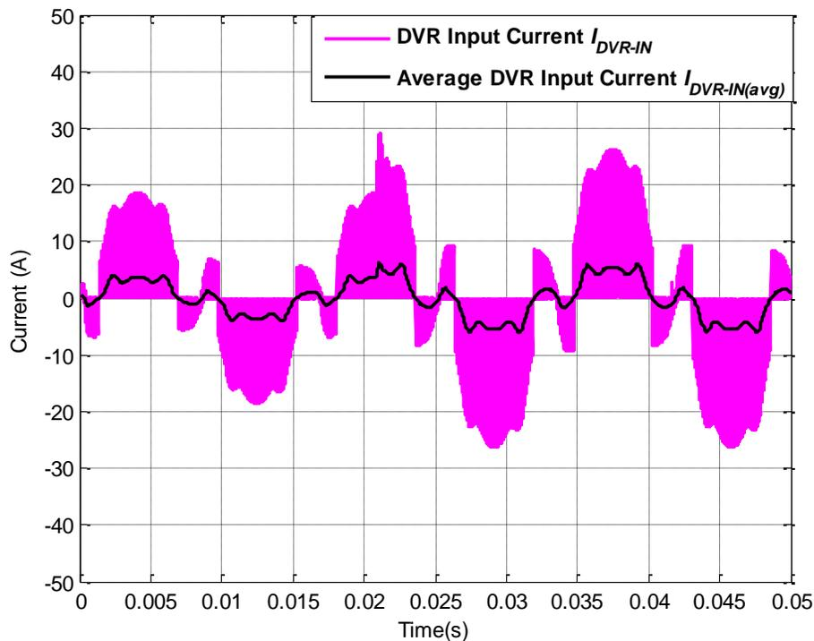
Figure 6.69: Actual DVR current  $I_{DVR-IN}$  and average DVR current  $I_{DVR-IN(avg)}$  for operating scenario XV
