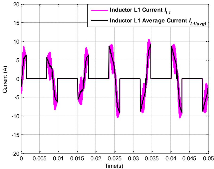
Figure A.61: Actual inductor current  $I_L$  and average inductor current  $I_{L(avg)}$  for operating scenario xv
