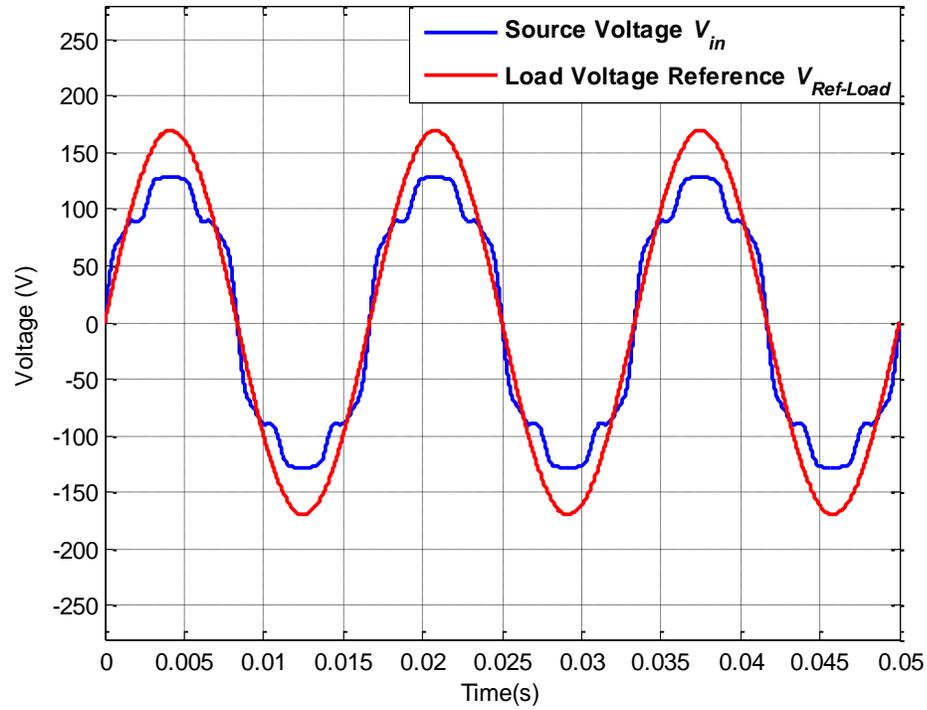
Figure 6.46: Source voltage  $V_{in}$  and load reference voltage  $V_{Ref-Load}$  for operating scenario XII
