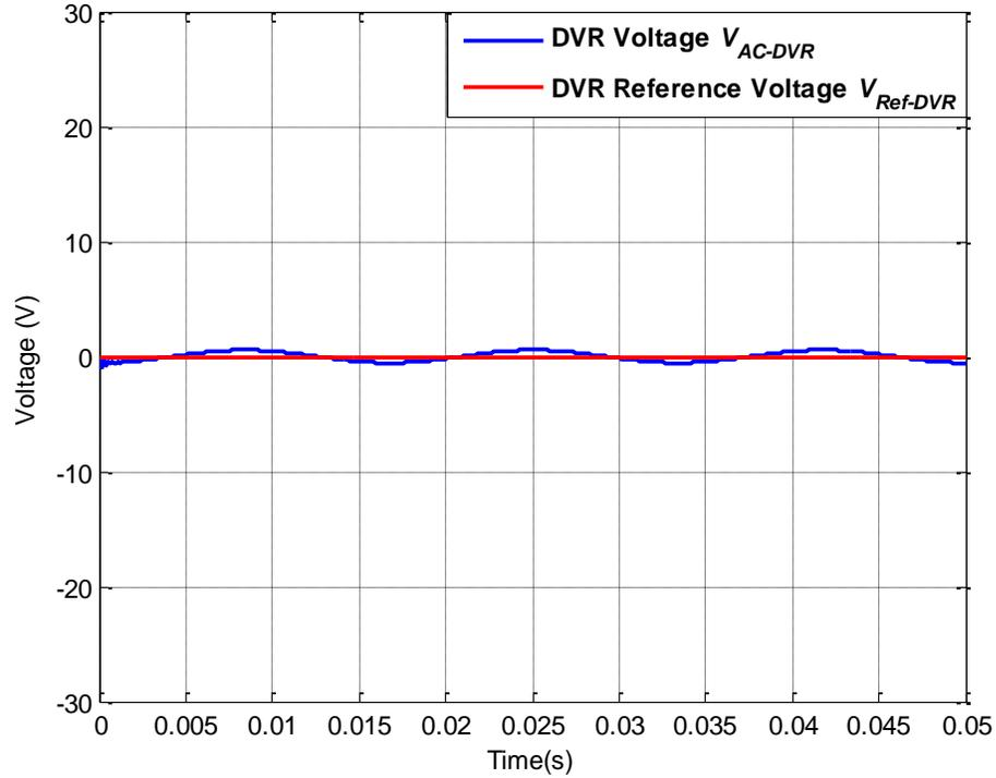
Figure A.3: AC-DVR voltage  $V_{AC-DVR}$  and DVR reference voltage  $V_{Ref-DVR}$  for operating scenario i
