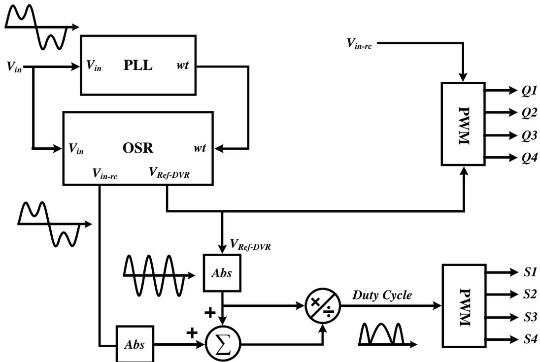
Figure 4.2 Control block diagram for proposed AC-AC DVR
