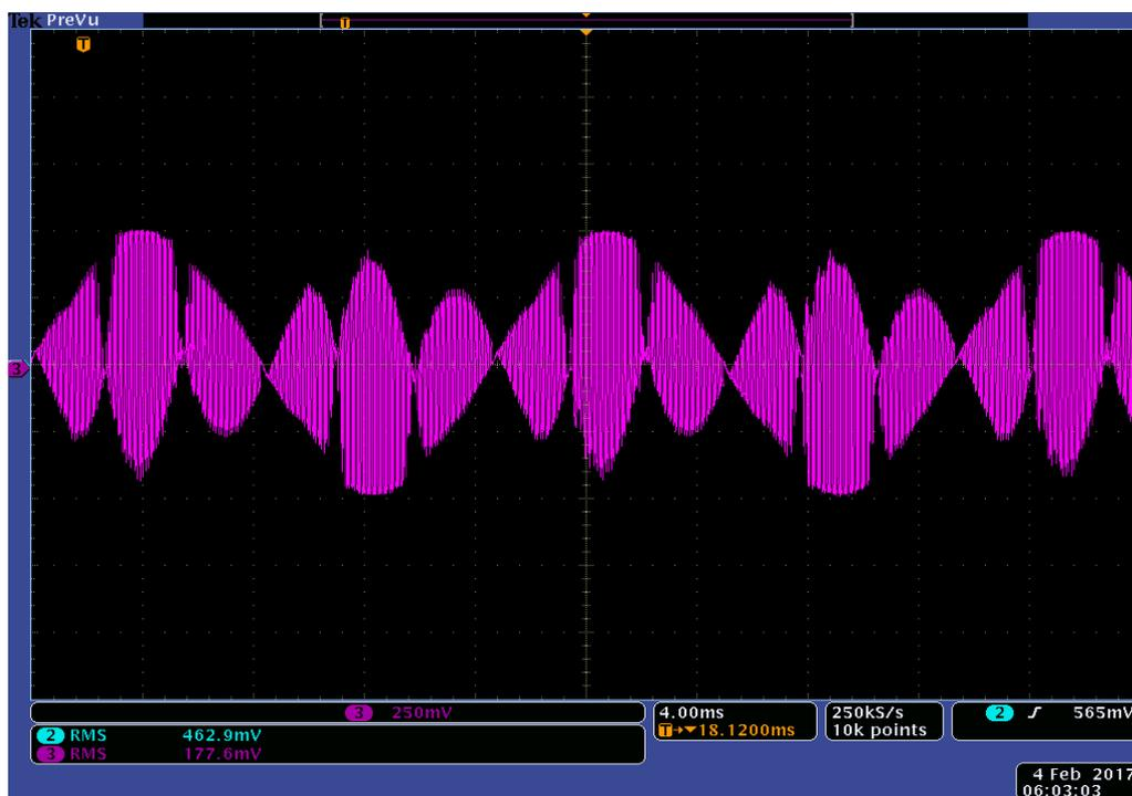
Figure 7.23: Experimental Results of Actual capacitor current  $I_C$  for operating scenario II
