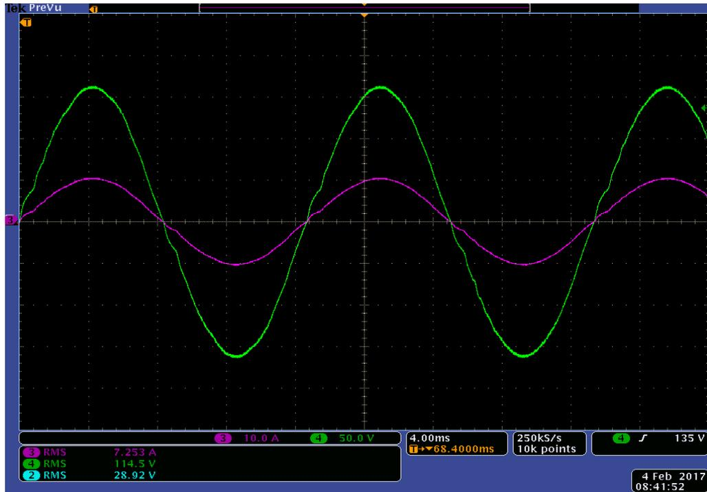
Figure 7.81: Experimental Results of Load voltage  $V_{Load}$  (Green) and load current  $I_{Load}$  (Pink) for experiment scenario XII
