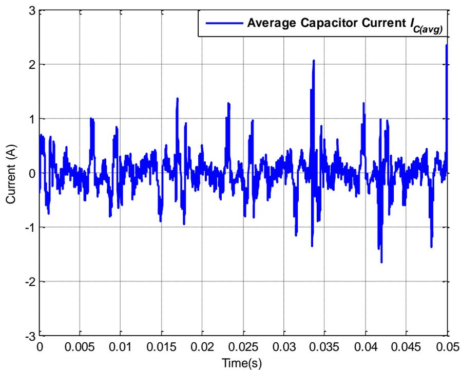
Figure A.51: Average capacitor current  $I_{C(avg)}$  for operating scenario xiii
