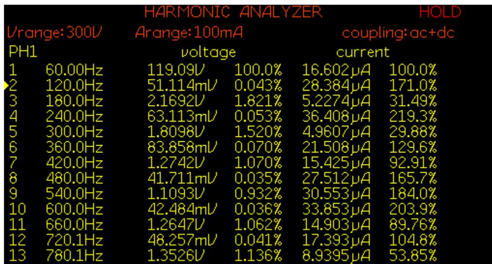
Figure 7.91: FFT of load voltage  $V_{Load}$  for experiment scenario XIII
