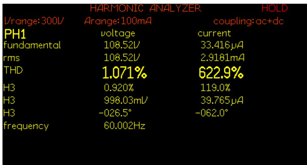
Figure 7.74: THD of load voltage  $V_{Load}$  for experiment scenario XI
