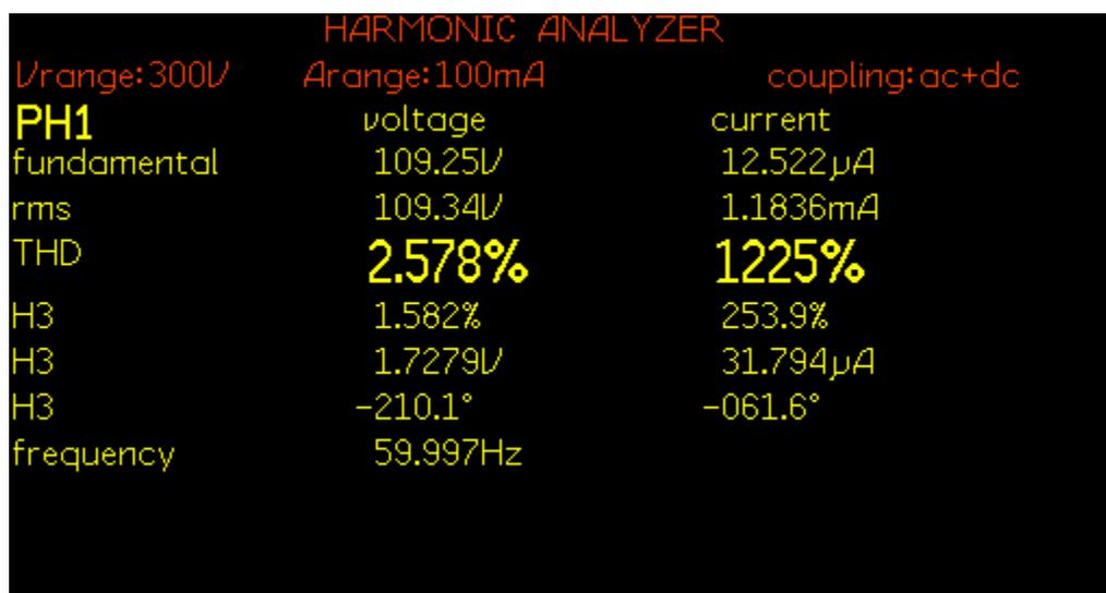
Figure 7.18: THD of load voltage  $V_{Load}$  for experiment scenario II
