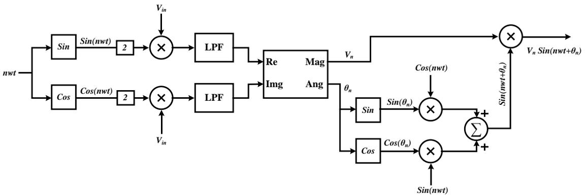
Figure 4.4: Block diagram of Fourier blocks
