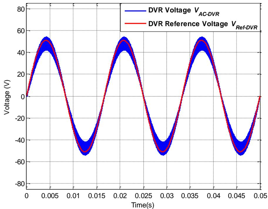
Figure A.35: AC-DVR voltage  $V_{AC-DVR}$  and DVR reference voltage  $V_{Ref-DVR}$  for operating scenario x
