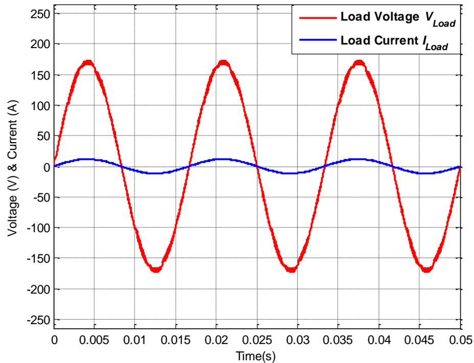
Figure 6.19: Load voltage  $V_{Load}$  and load current  $I_{Load}$  for operating scenario III
