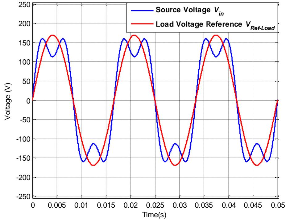
Figure A.5: Source voltage  $V_{in}$  and load reference voltage  $V_{Ref-Load}$  for operating scenario ii
