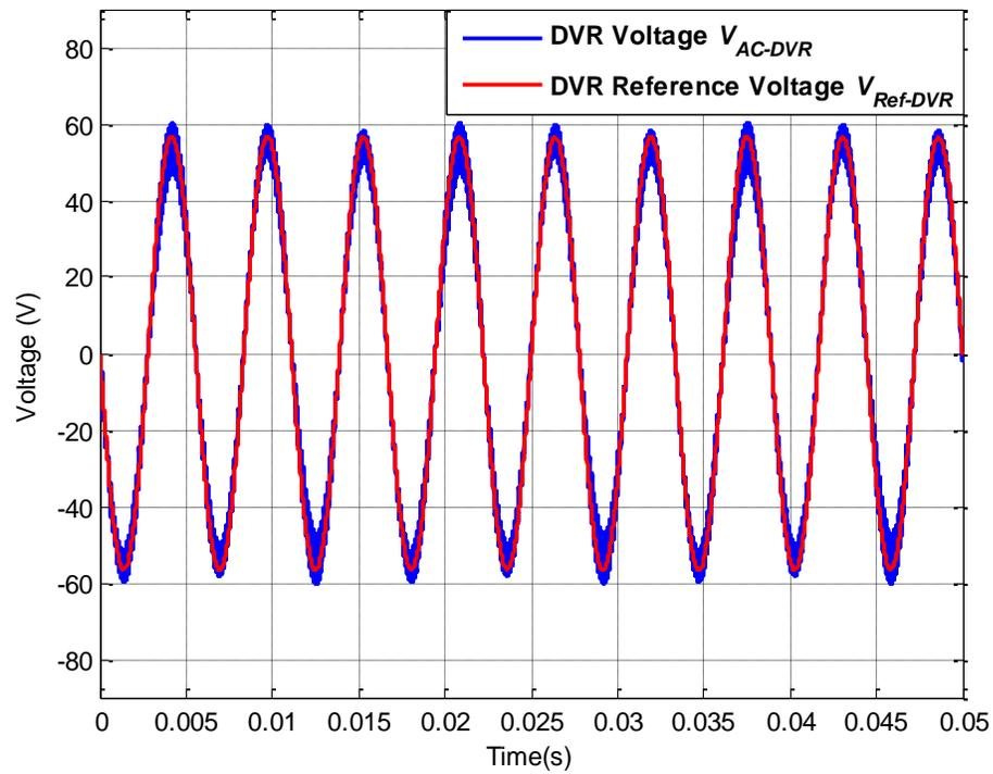
Figure A.6: AC-DVR voltage  $V_{AC-DVR}$  and DVR reference voltage  $V_{Ref-DVR}$  for operating scenario ii
