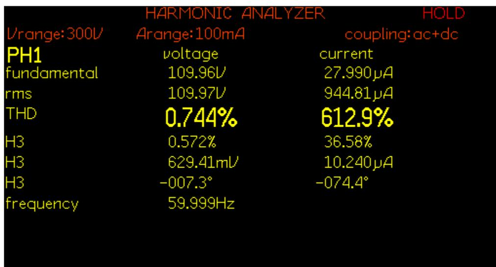
Figure 7.98: THD of load voltage  $V_{Load}$  for experiment scenario XIV
