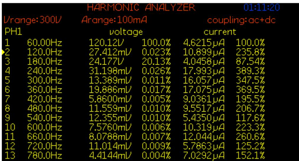
Figure 7.102: FFT-3<sup>rd</sup> of source voltage  $V_{in}$  for experiment scenario XVII
