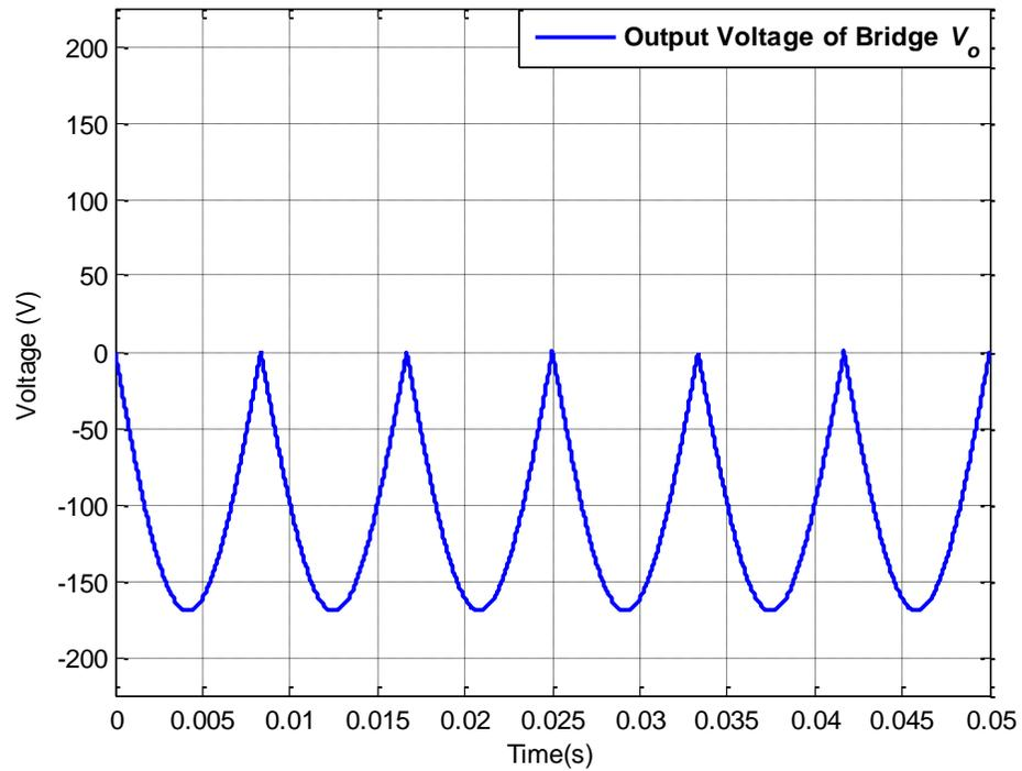
Figure 6.2 Bridge output voltage  $V_o$  for operating scenario I
