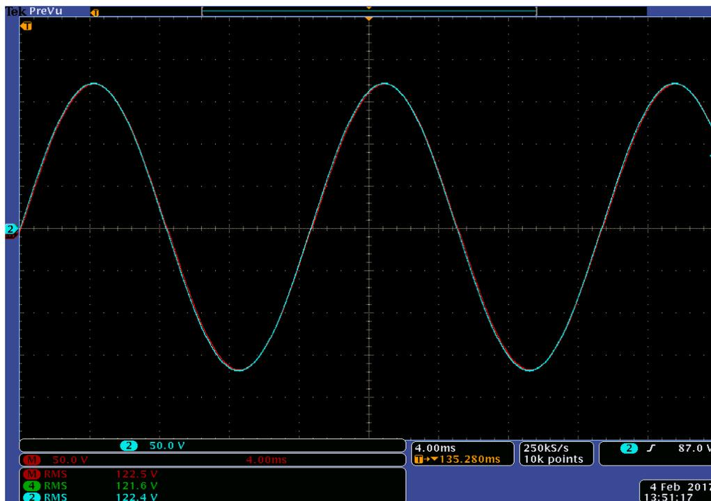
Figure 7.92: Experimental results of Source voltage  $V_{in}$  (Blue) and load reference voltage  $V_{Ref-Load}$  (Red) for experiment scenario XIV
