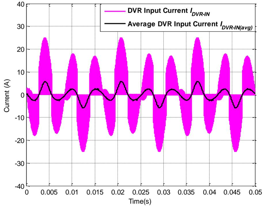
Figure A.9: Actual DVR current  $I_{DVR-IN}$  and average DVR current  $I_{DVR-IN(avg)}$  for operating scenario ii
