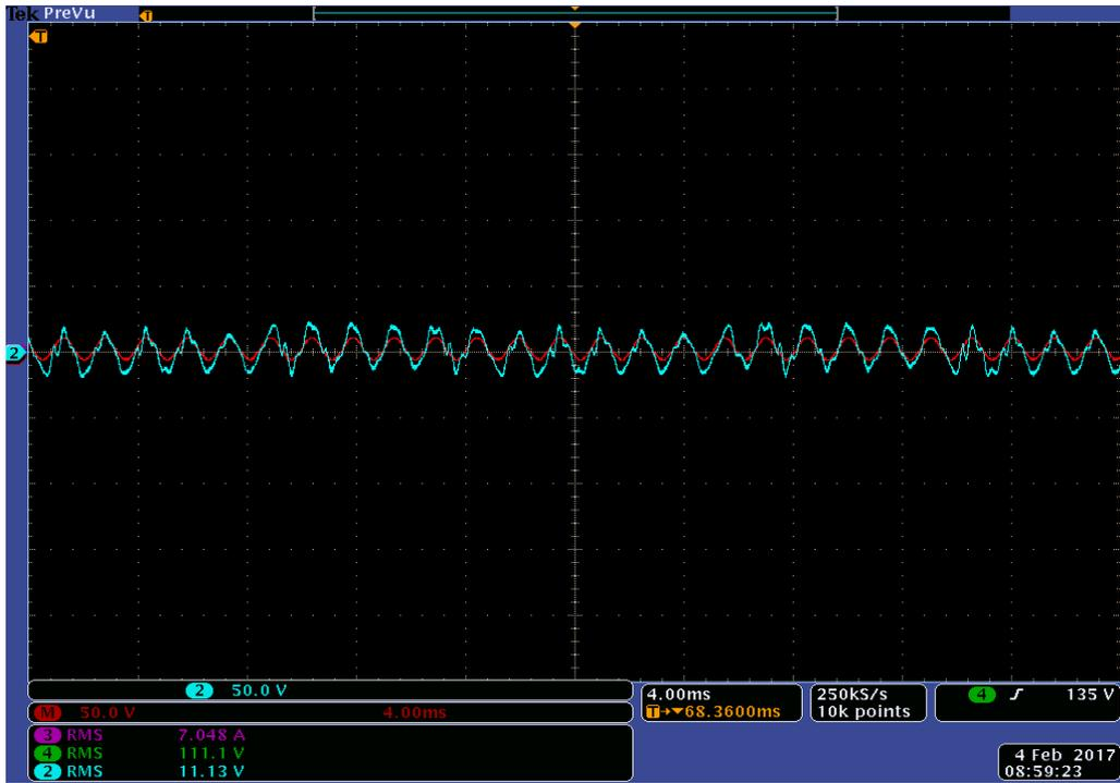
Figure 7.36: Experimental results of AC-DVR voltage  $V_{AC-DVR}$  (Blue) and DVR reference voltage  $V_{Ref-DVR}$  (Red) for experiment scenario IV
