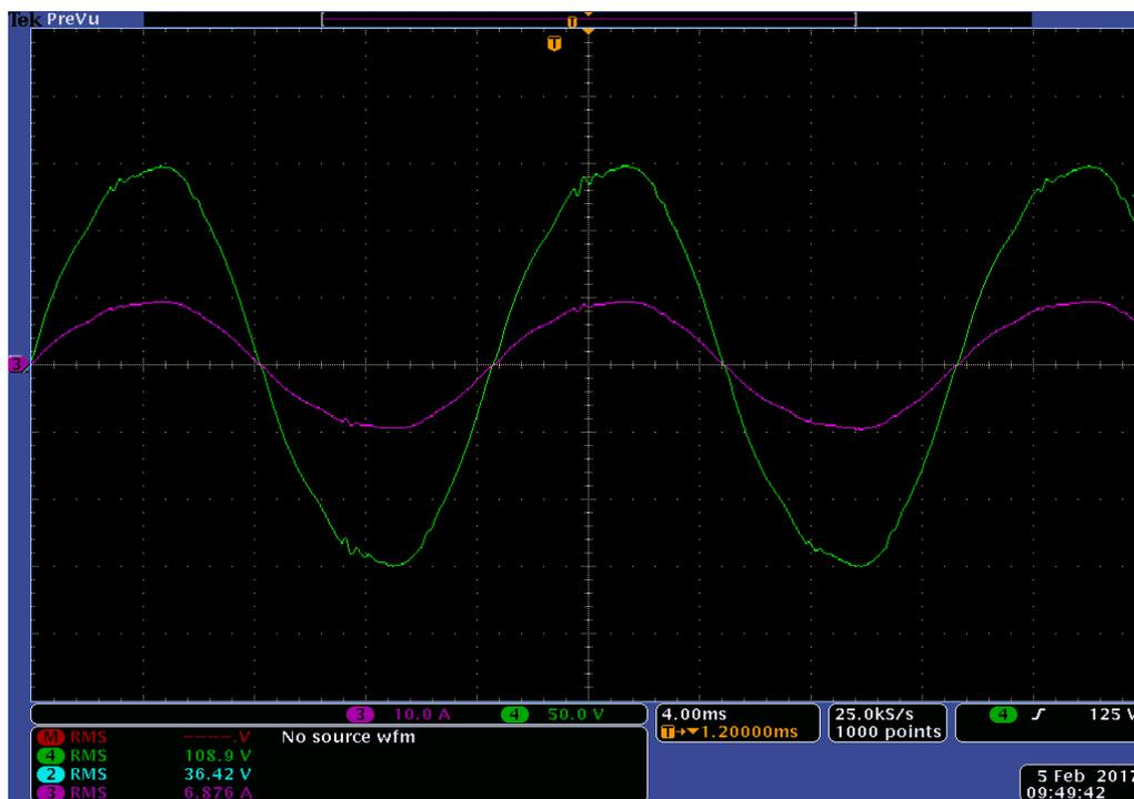
Figure 7.17: Experimental Results of Load voltage  $V_{Load}$  (Green) and load current  $I_{Load}$  (Pink) for experiment scenario II
