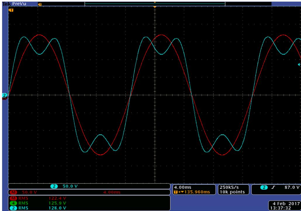
Figure 7.12: Experimental results of Source voltage  $V_{in}$  (Blue) and load reference voltage  $V_{Ref-Load}$  (Red) for experiment scenario II
