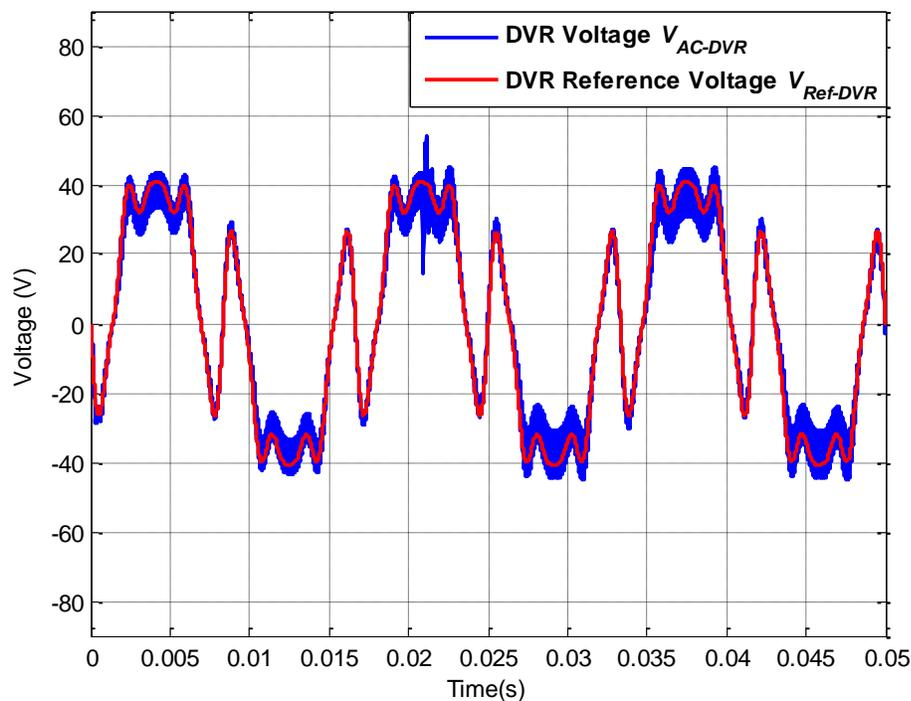
Figure A.57: AC-DVR voltage  $V_{AC-DVR}$  and DVR reference voltage  $V_{Ref-DVR}$  for operating scenario xv
