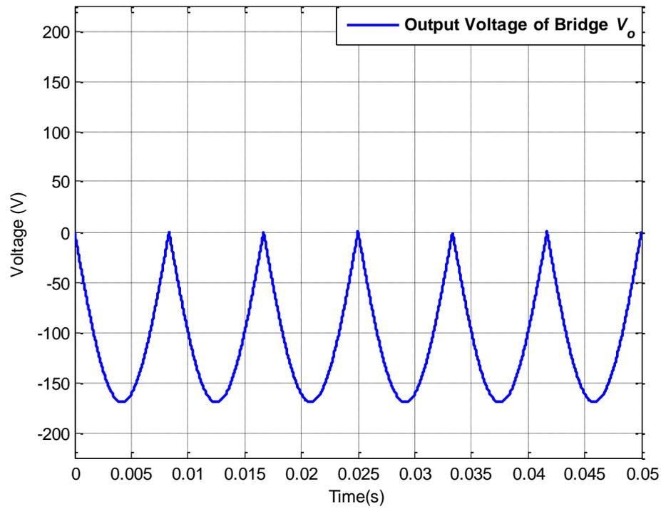
Figure 6.61: Bridge output voltage  $V_o$  for operating scenario XIV
