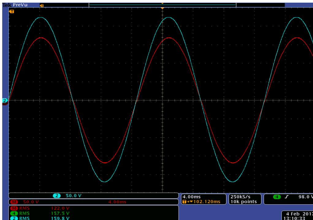
Figure 7.68: Experimental results of Source voltage  $V_{in}$  (Blue) and load reference voltage  $V_{Ref-Load}$  (Red) for experiment scenario XI
