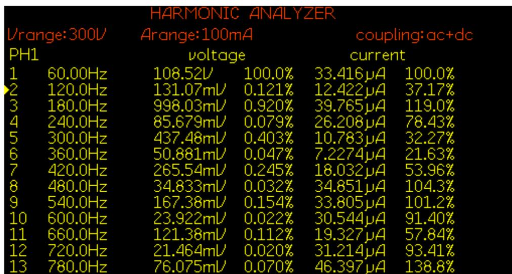
Figure 7.75: FFT of load voltage  $V_{Load}$  for experiment scenario XI
