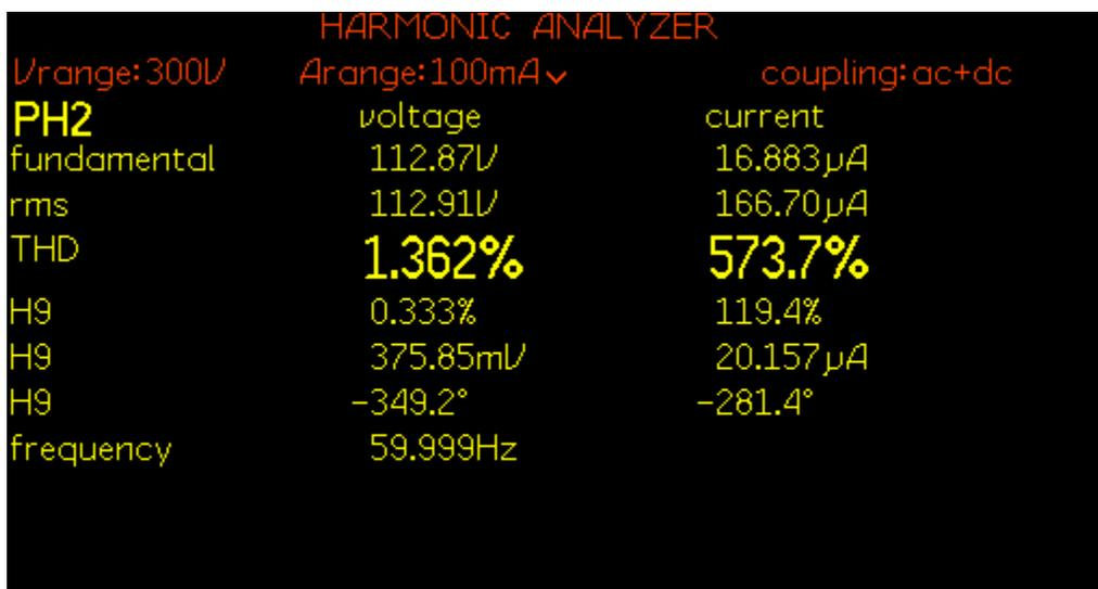
Figure 7.108: THD-3<sup>rd</sup> of load voltage  $V_{Load}$  for experiment scenario XVII
