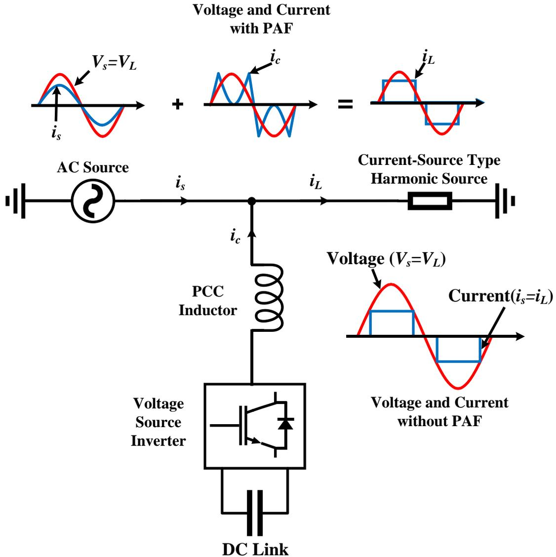
Figure 2.17: Parallel Active Filter (PAF) schematic and operation
