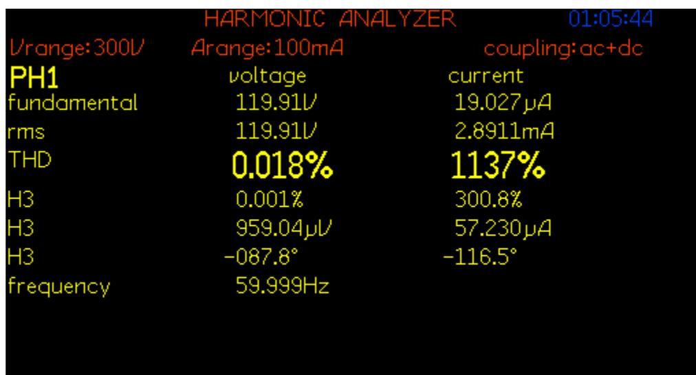
Figure 7.5: THD of source voltage  $V_{in}$  for experiment scenario I
