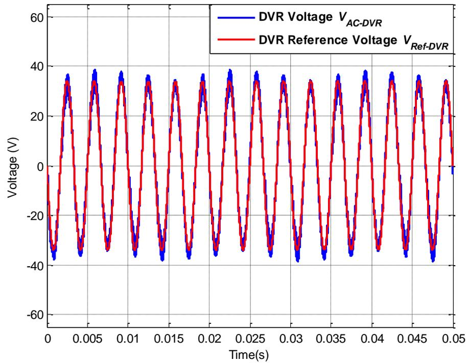
Figure 6.18: AC-DVR voltage  $V_{AC-DVR}$  and DVR reference voltage  $V_{Ref-DVR}$  for operating scenario III
