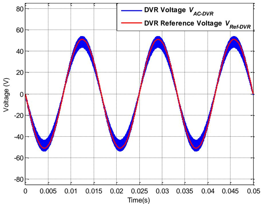
Figure A.38: AC-DVR voltage  $V_{AC-DVR}$  and DVR reference voltage  $V_{Ref-DVR}$  for operating scenario xi
