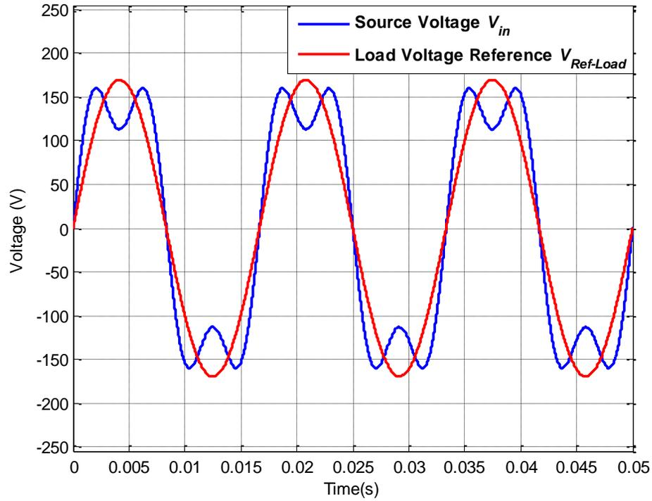
Figure 6.6: Source voltage  $V_{in}$  and load reference voltage  $V_{Ref-Load}$  for operating scenario II
