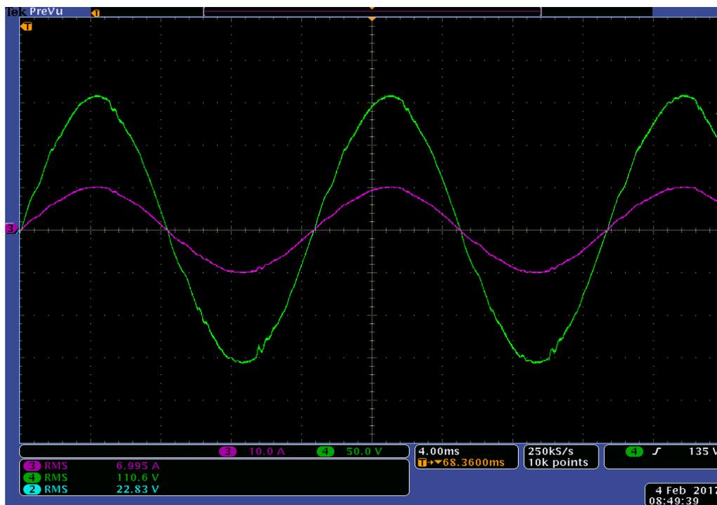
Figure 7.29: Experimental Results of Load voltage  $V_{Load}$  (Green) and load current  $I_{Load}$  (Pink) for experiment scenario III
