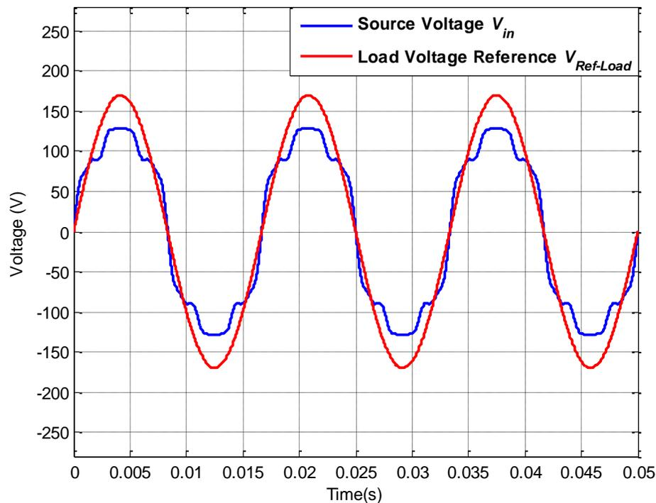
Figure A.56: Source voltage  $V_{in}$  and load reference voltage  $V_{Ref-Load}$  for operating scenario xv
