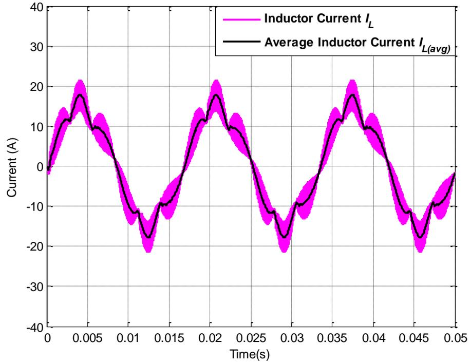
Figure 6.12: Actual inductor current  $I_L$  and average inductor current  $I_{L(avg)}$  for operating scenario II
