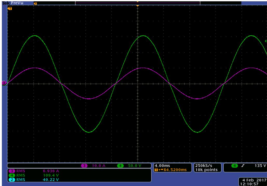
Figure 7.73: Experimental Results of Load voltage  $V_{Load}$  (Green) and load current  $I_{Load}$  (Pink) for experiment scenario XI
