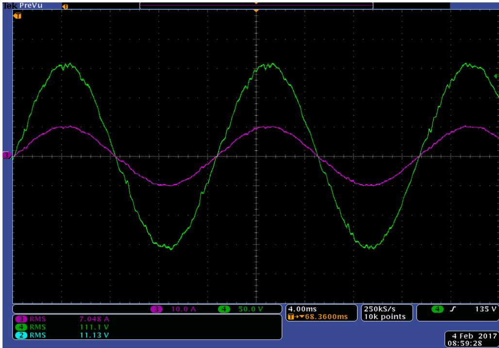
Figure 7.37: Experimental Results of Load voltage  $V_{Load}$  (Green) and load current  $I_{Load}$  (Pink) for experiment scenario IV
