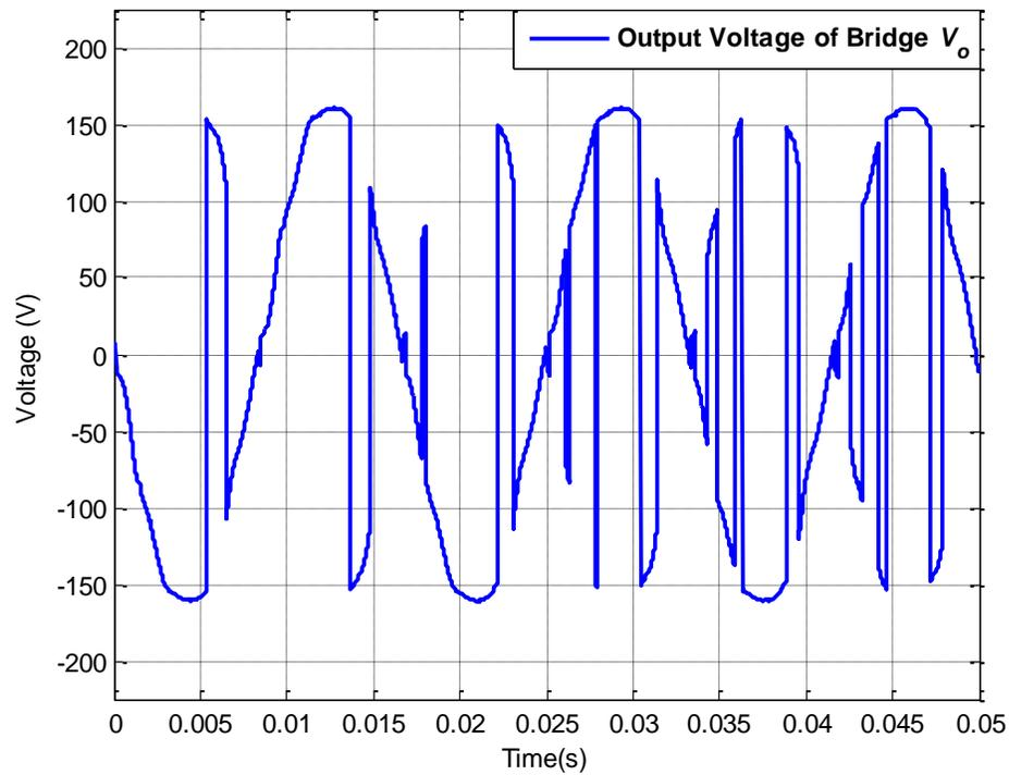
Figure 6.51: Bridge output voltage  $V_o$  for operating scenario XIII
