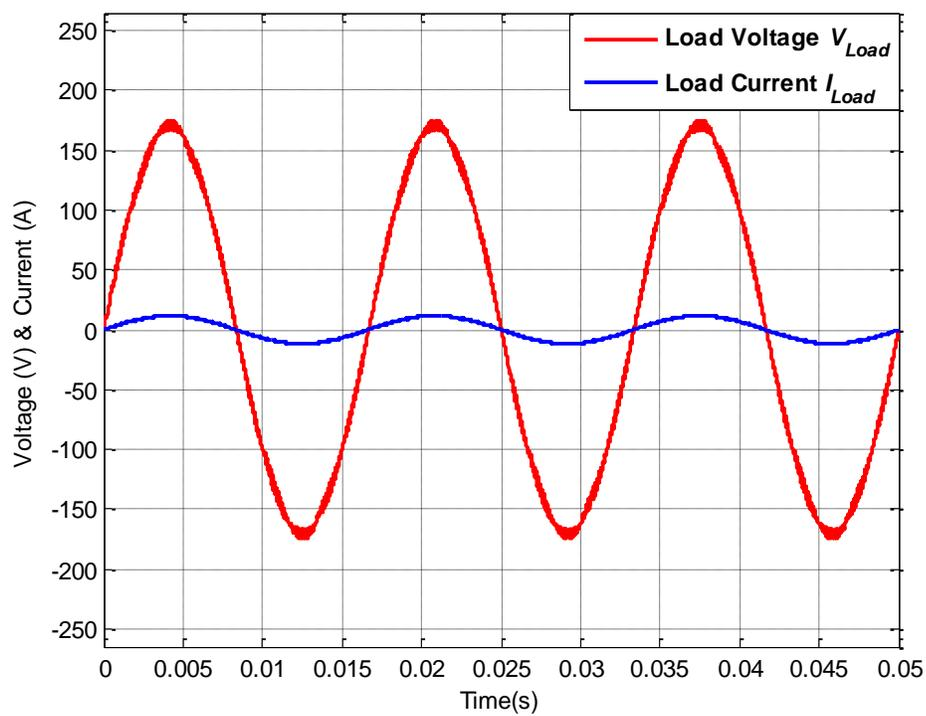
Figure A.17: Load voltage  $V_{Load}$  and load current  $I_{Load}$  for operating scenario iii
