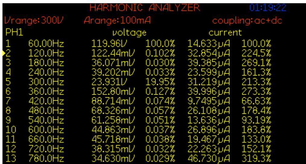
Figure 7.26: FFT of source voltage  $V_{in}$  for experiment scenario III
