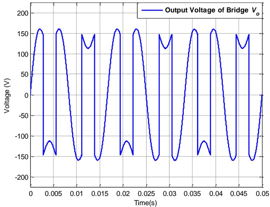
Figure 6.7: Bridge output voltage  $V_o$  for operating scenario II
