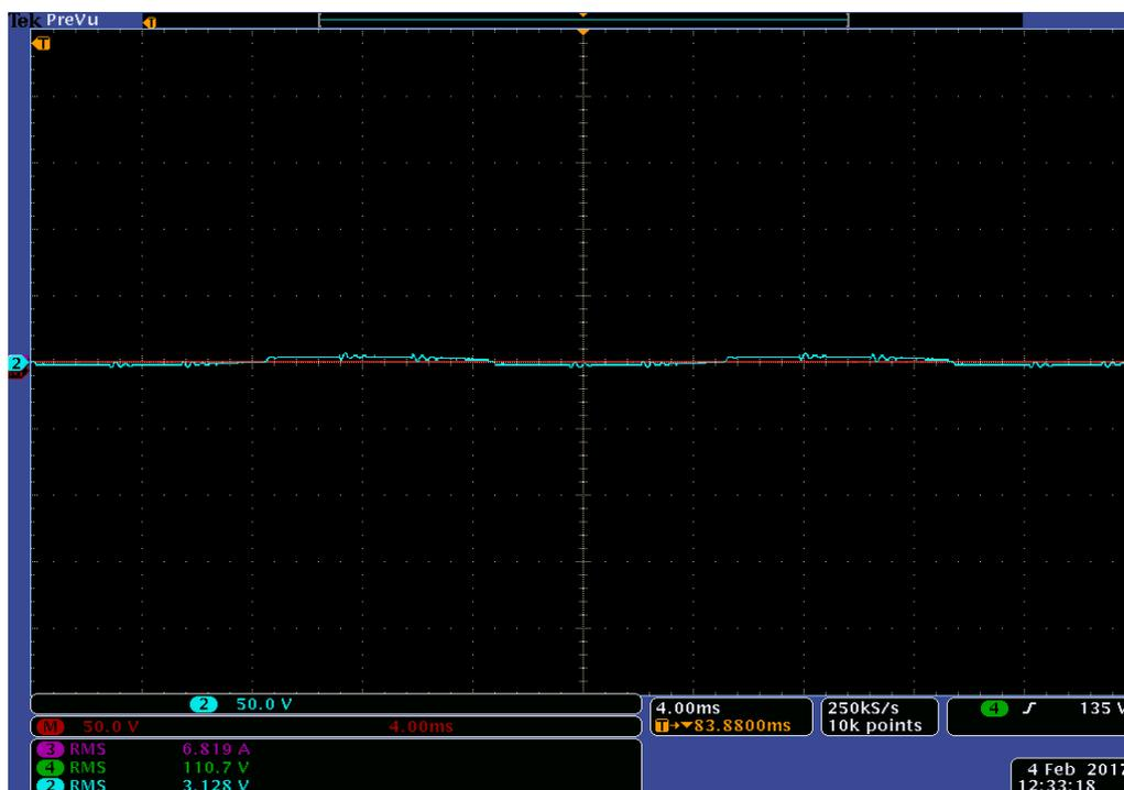
Figure 7.96: Experimental results of AC-DVR voltage  $V_{AC-DVR}$  (Blue) and DVR reference voltage  $V_{Ref-DVR}$  (Red) for experiment scenario XIV
