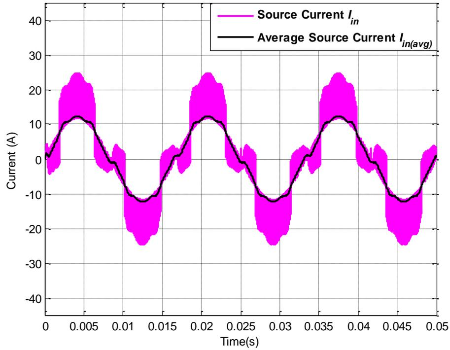
Figure 6.28: Actual source current  $I_{in}$  and average source current  $I_{in(avg)}$  for operating scenario VIII
