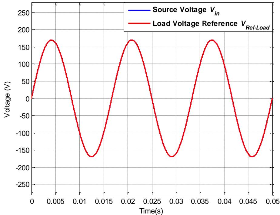
Figure 6.1: Source voltage  $V_{in}$  and load reference voltage  $V_{Ref-Load}$  for operating scenario I
