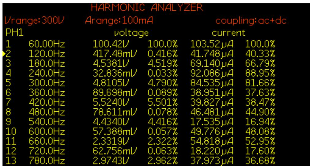
Figure 7.59: FFT of load voltage  $V_{Load}$  for experiment scenario IX
