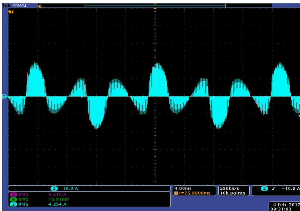
Figure 7.21: Experimental Results of Actual DVR current  $I_{DVR-IN}$  for experiment scenario II
