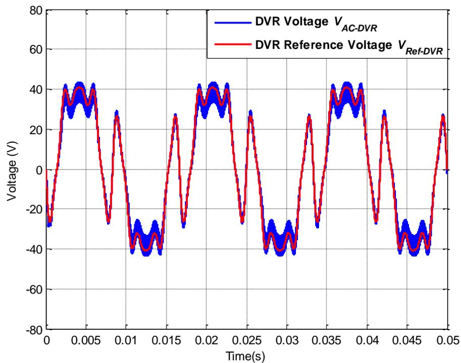
Figure A.41: AC-DVR voltage  $V_{AC-DVR}$  and DVR reference voltage  $V_{Ref-DVR}$  for operating scenario xii
