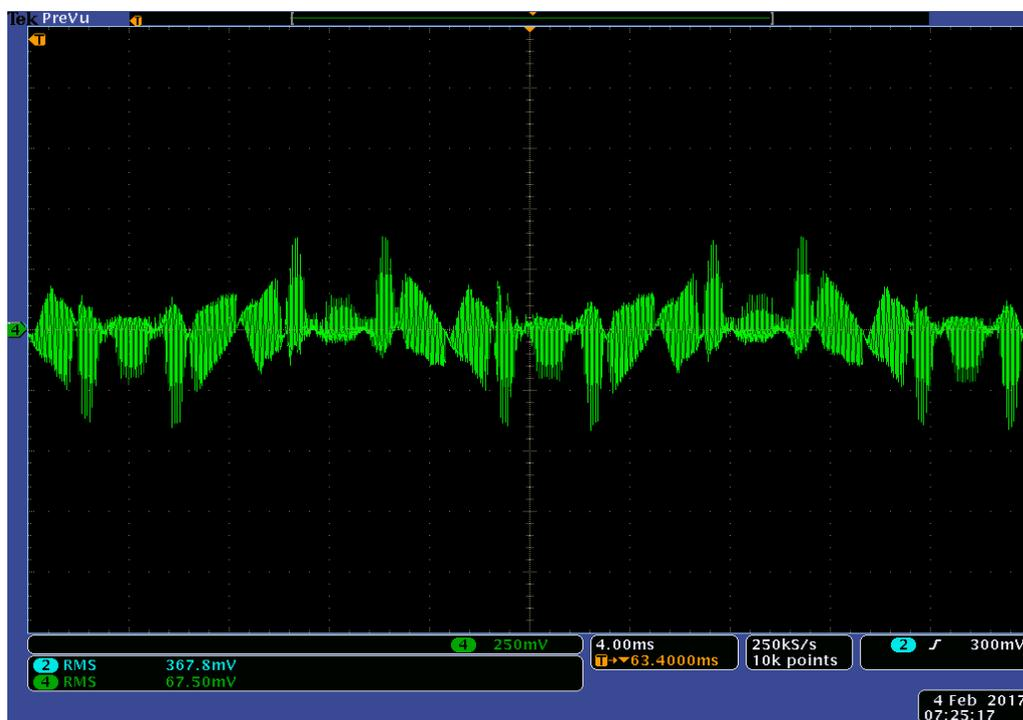
Figure 7.51: Experimental Results of Actual capacitor current  $I_C$  for operating scenario VIII
