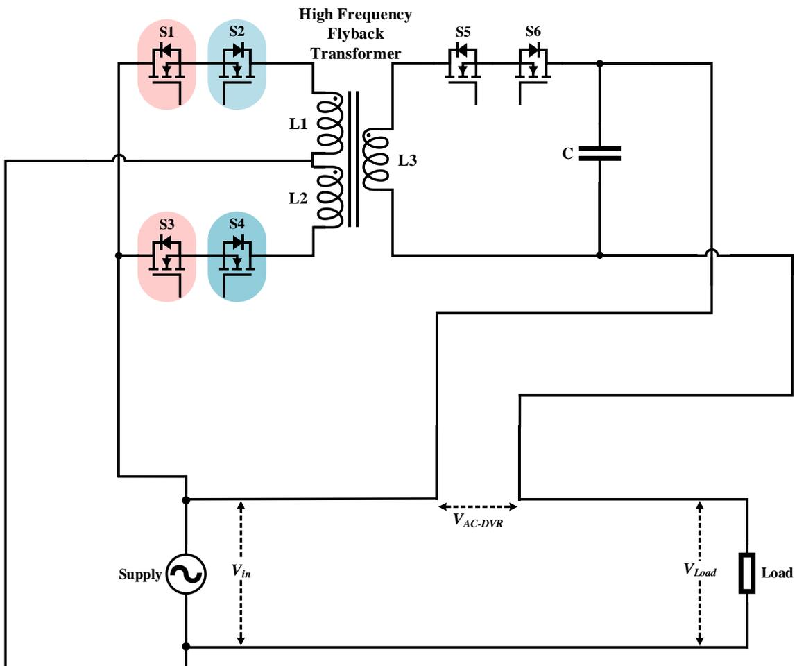
Figure A.1 Possible modifications in proposed AC-DVR
