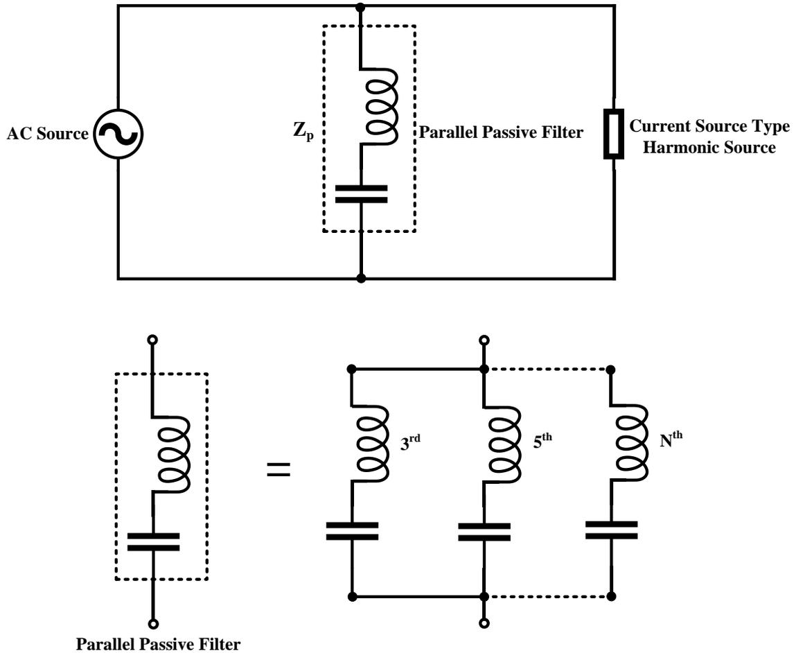
Figure 2.15: Parallel Passive Filter (PPF) schematic [24]
