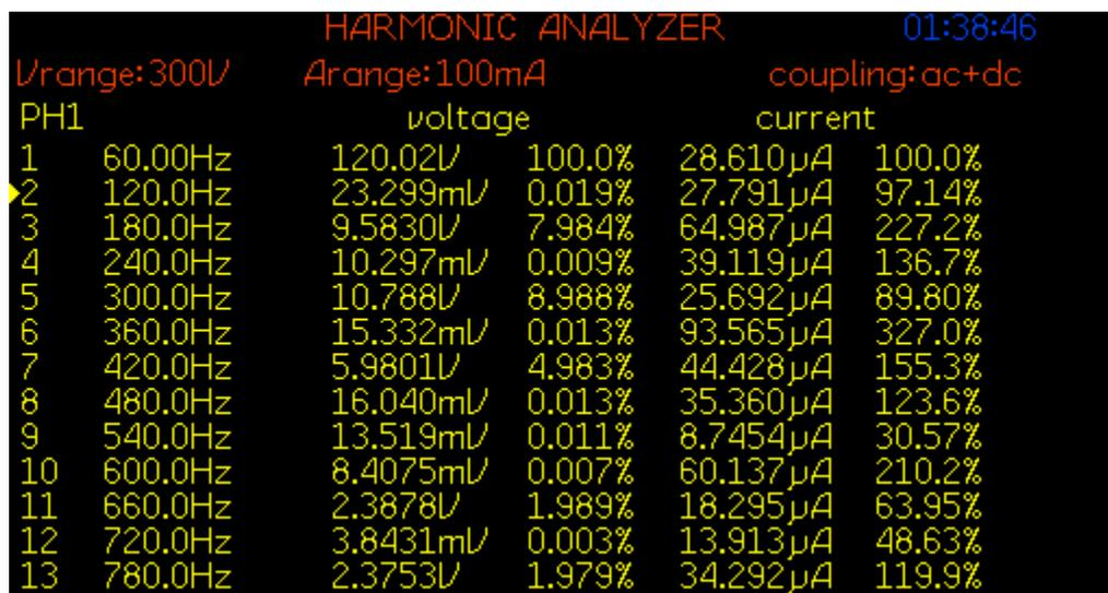
Figure 7.42: FFT of source voltage  $V_{in}$  for experiment scenario VIII
