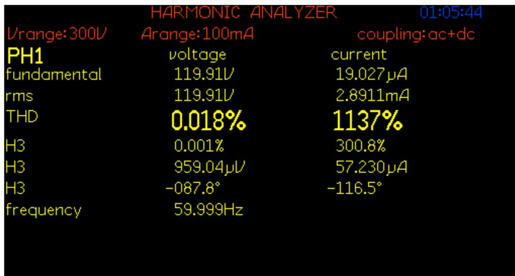
Figure 7.93: THD of source voltage  $V_{in}$  for experiment scenario XIV
