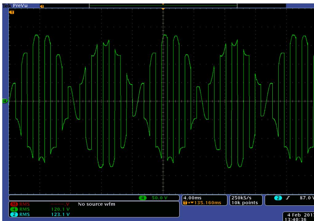
Figure 7.35: Experimental results of Bridge output voltage  $V_o$  for experiment scenario IV
