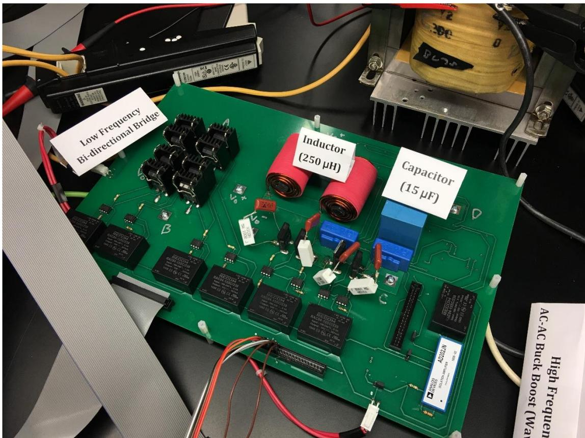
Figure 7.1: Experimental setup of AC-DVR
