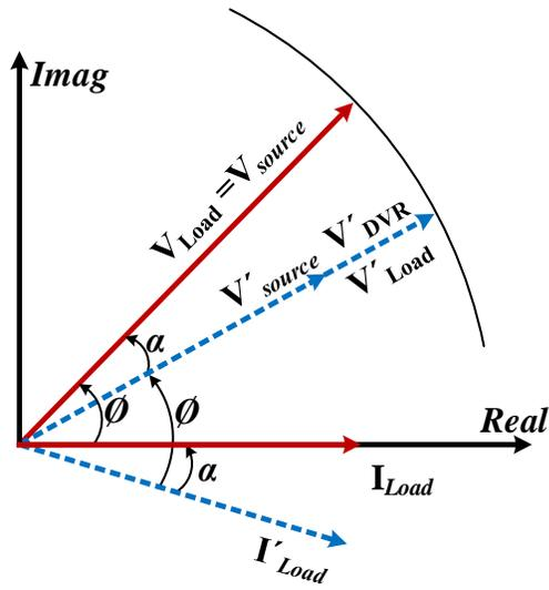
Figure 2.9: In-phase compensation phasor diagram
