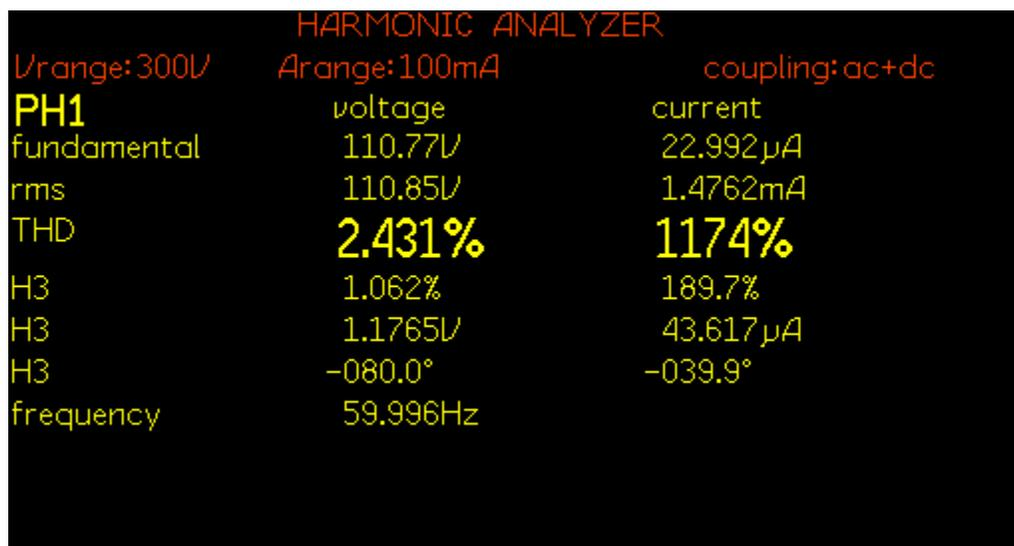
Figure 7.46: THD of load voltage  $V_{Load}$  for experiment scenario VIII
