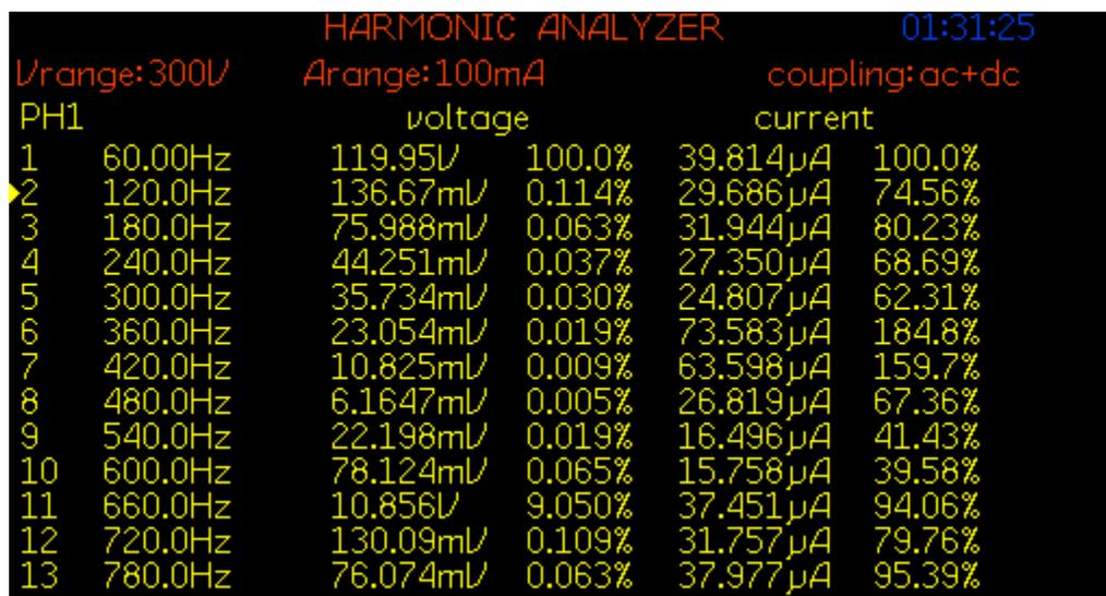
Figure 7.34: FFT of source voltage  $V_{in}$  for experiment scenario IV
