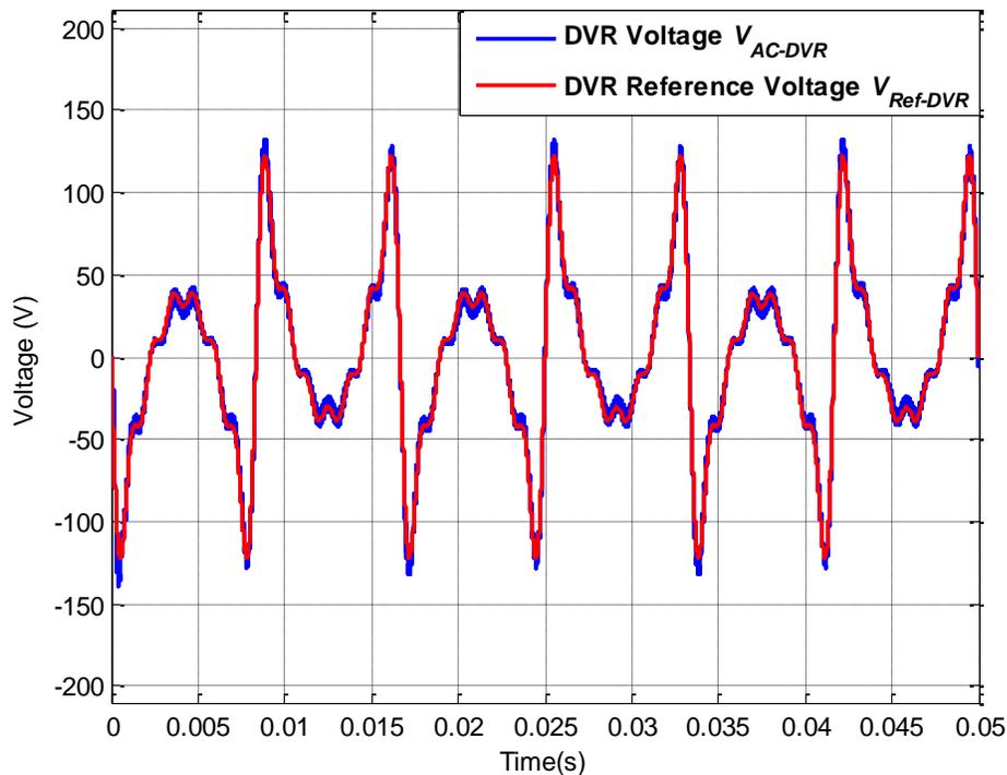
Figure A.32: AC-DVR voltage  $V_{AC-DVR}$  and DVR reference voltage  $V_{Ref-DVR}$  for operating scenario ix
