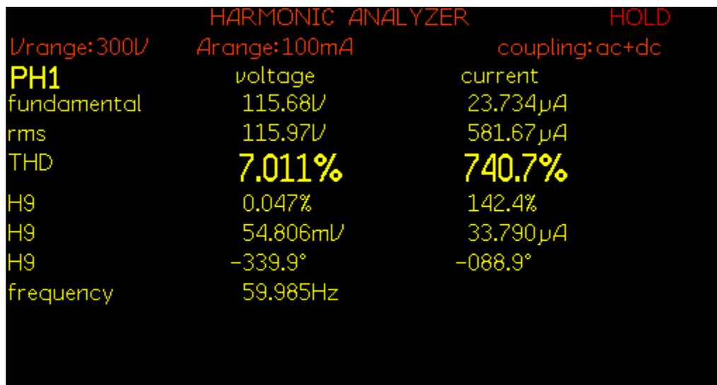
Figure 7.85: THD of source voltage  $V_{in}$  for experiment scenario XIII
