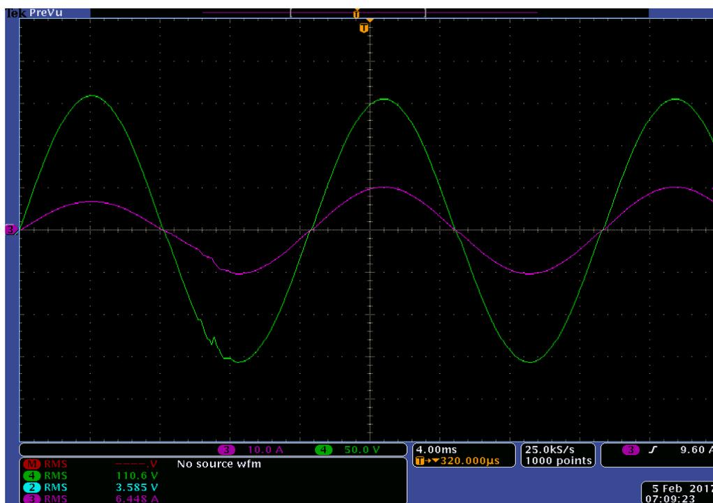
Figure 7.97: Experimental Results of Load voltage  $V_{Load}$  (Green) and load current  $I_{Load}$  (Pink) for experiment scenario XIV
