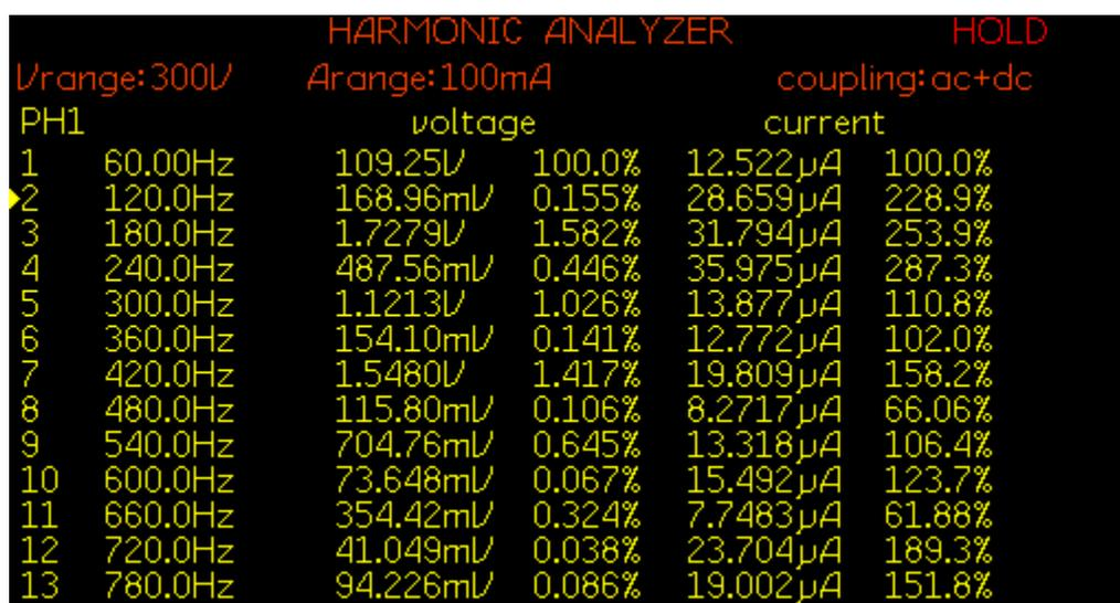
Figure 7.19: FFT of load voltage  $V_{Load}$  for experiment scenario II
