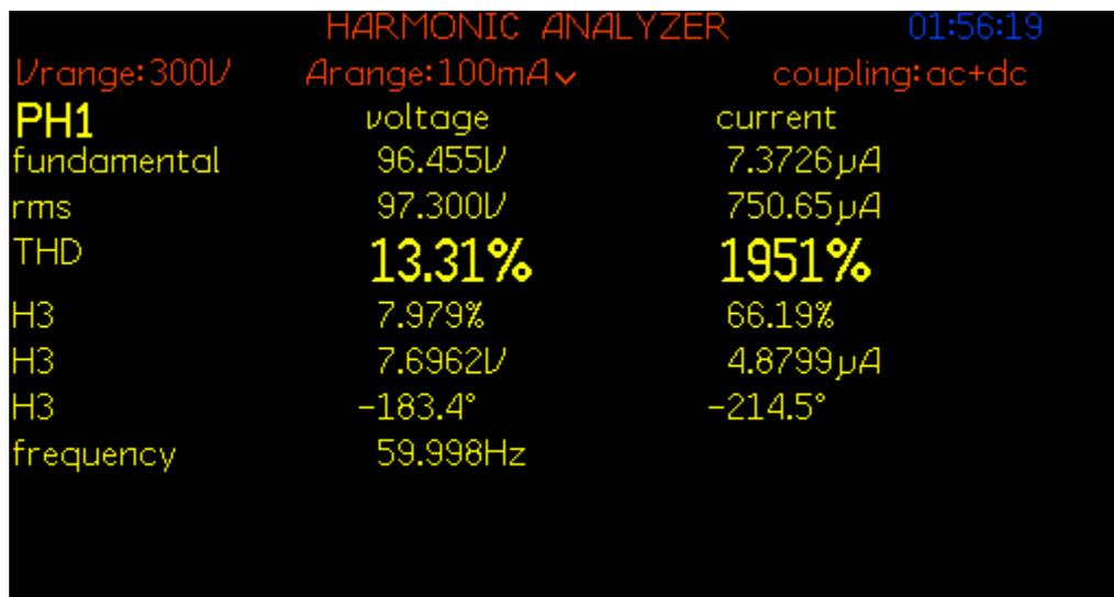
Figure 7.77: THD of source voltage  $V_{in}$  for experiment scenario XII
