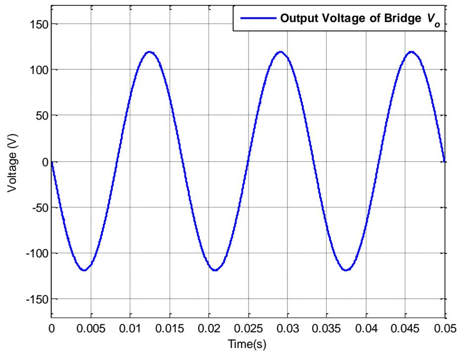
Figure 6.39: Bridge output voltage  $V_o$  for operating scenario X
