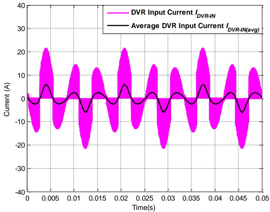
Figure 6.11: Actual DVR current  $I_{DVR-IN}$  and average DVR current  $I_{DVR-IN(avg)}$  for operating scenario II
