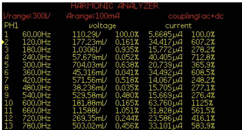
Figure 7.39: FFT of load voltage  $V_{Load}$  for experiment scenario IV
