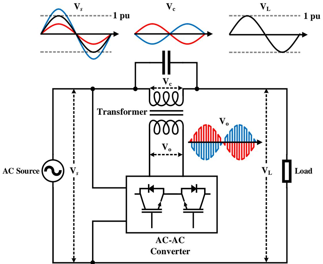
Figure 2.13: Static Voltage Regulator (SVR)
