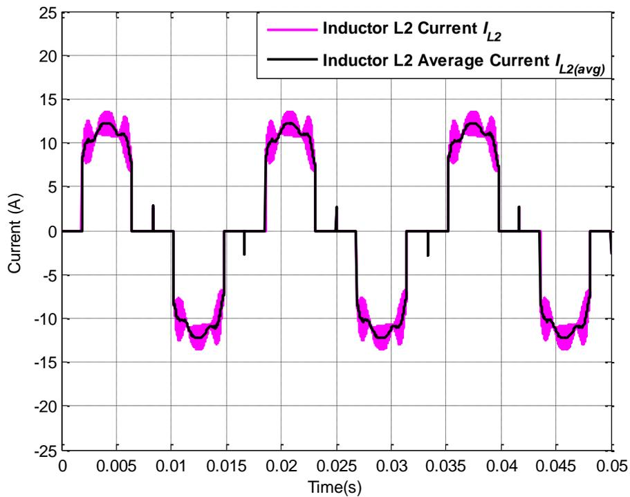
Figure A.27: Actual inductor current  $I_L$  and average inductor current  $I_{L(avg)}$  for operating scenario viii
