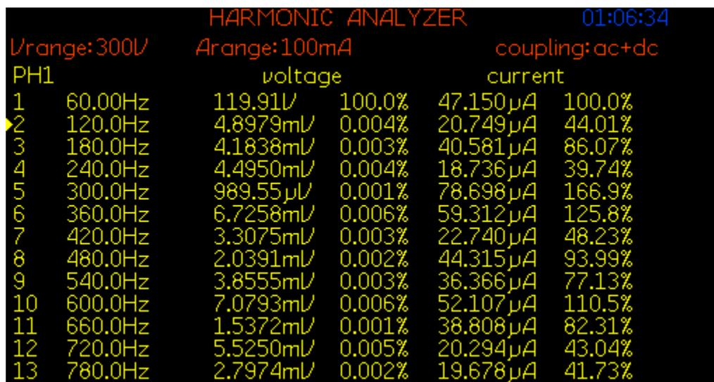
Figure 7.94: FFT of source voltage  $V_{in}$  for experiment scenario XIV
