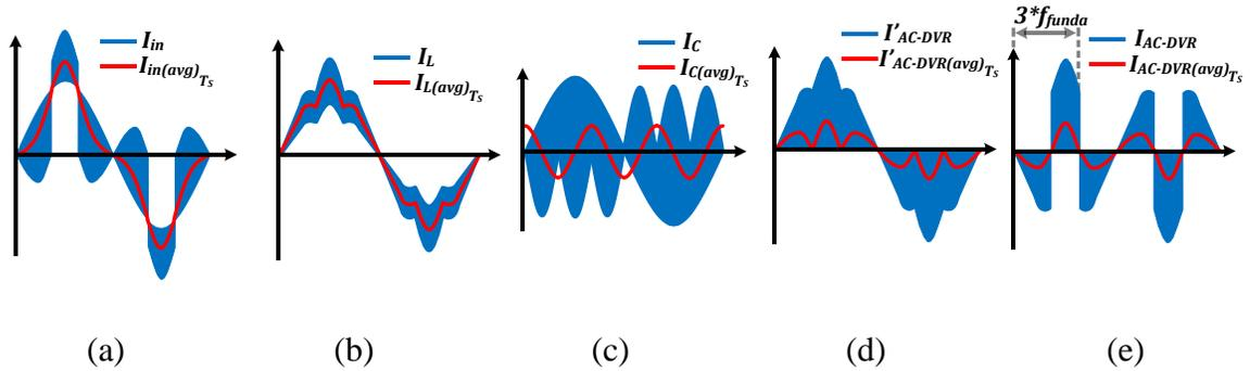
Figure 4.1: Actual (switched) and average current waveforms (a) Source current, (b) Inductor current, (c) capacitor current, (d) Wave shaper input current, (e) AC-DVR input current
