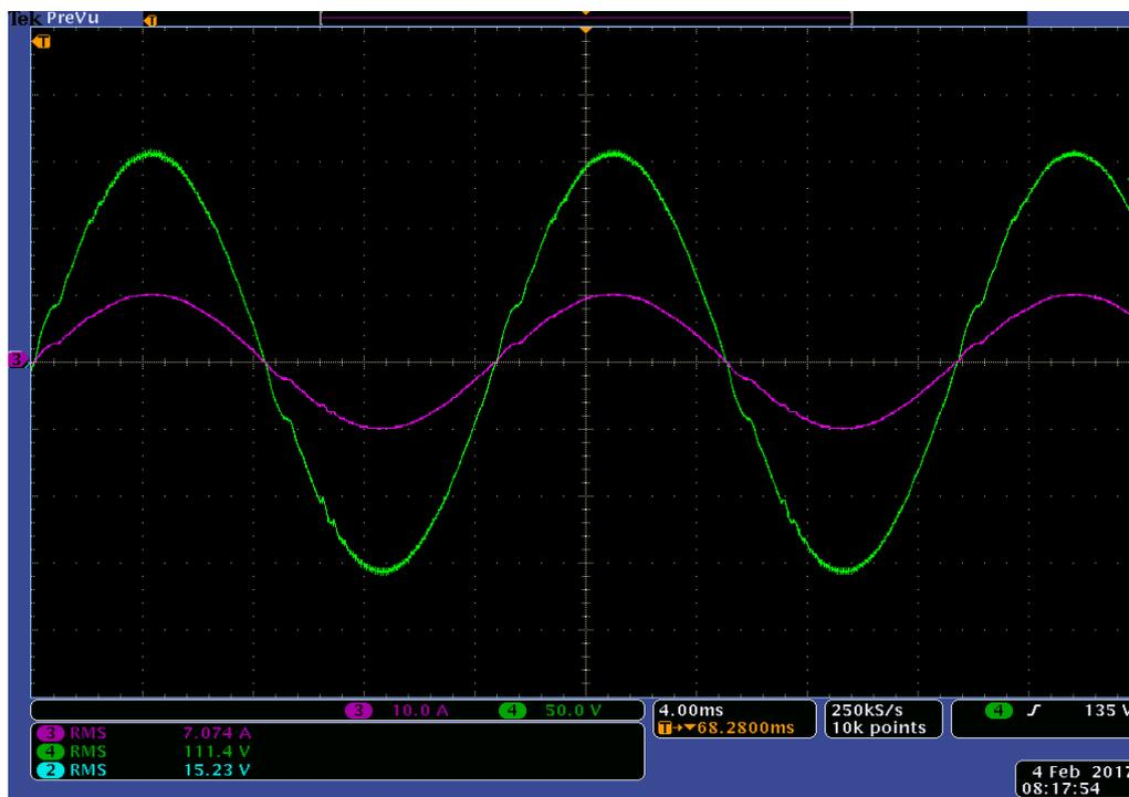
Figure 7.45: Experimental Results of Load voltage  $V_{Load}$  (Green) and load current  $I_{Load}$  (Pink) for experiment scenario VIII
