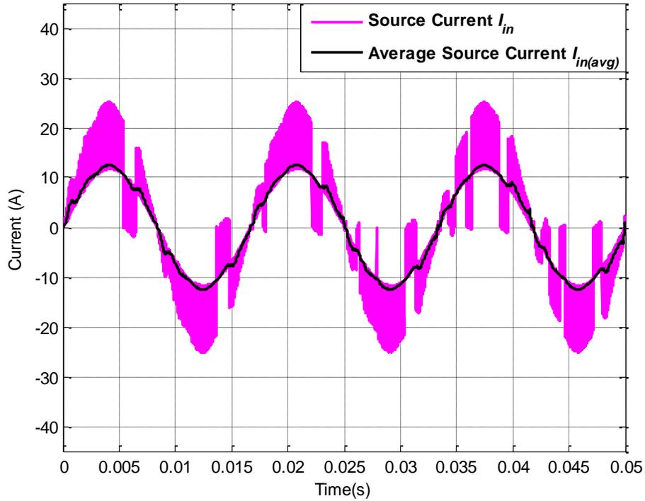
Figure 6.54: Actual source current  $I_{in}$  and average source current  $I_{in(avg)}$  for operating scenario XIII
