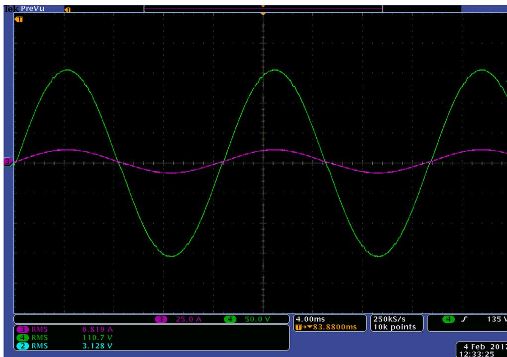
Figure 7.9: Experimental Results of Load voltage  $V_{Load}$  (Green) and load current  $I_{Load}$  (Pink) for experiment scenario I
