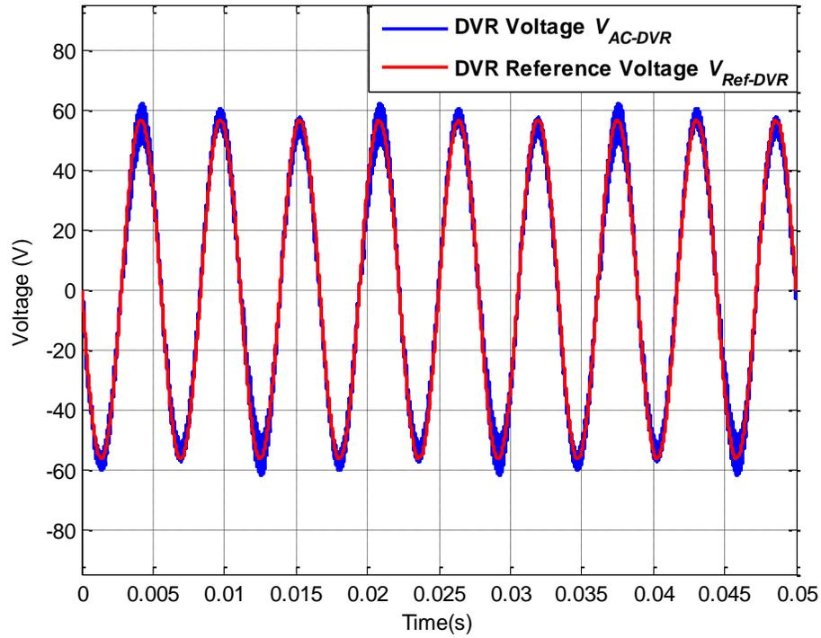
Figure 6.8: AC-DVR voltage  $V_{AC-DVR}$  and DVR reference voltage  $V_{Ref-DVR}$  for operating scenario II
