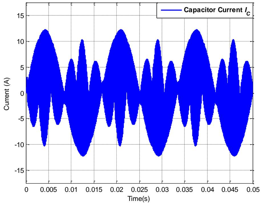
Figure 6.13: Actual capacitor current  $I_C$  for operating scenario II
