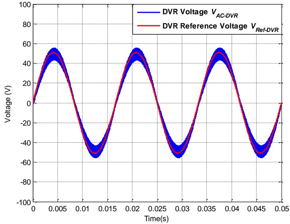
Figure 6.40: AC-DVR voltage  $V_{AC-DVR}$  and DVR reference voltage  $V_{Ref-DVR}$  for operating scenario X
