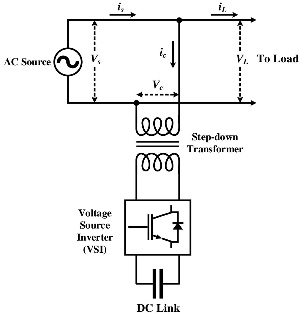
Figure 2.5: VSI (Voltage Source Inverter) based D-STATCOM
