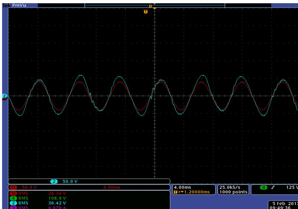
Figure 7.16: Experimental results of AC-DVR voltage  $V_{AC-DVR}$  (Blue) and DVR reference voltage  $V_{Ref-DVR}$  (Red) for experiment scenario II
