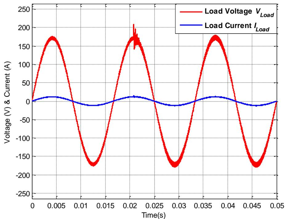
Figure A.68: Load voltage  $V_{Load}$  and load current  $I_{Load}$  for operating scenario xvi
