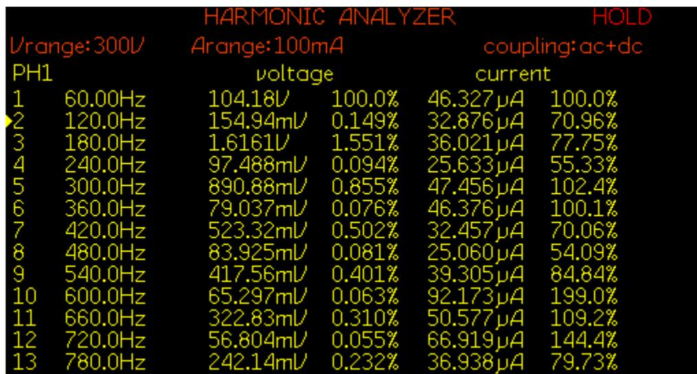
Figure 7.67: FFT of load voltage  $V_{Load}$  for experiment scenario X
