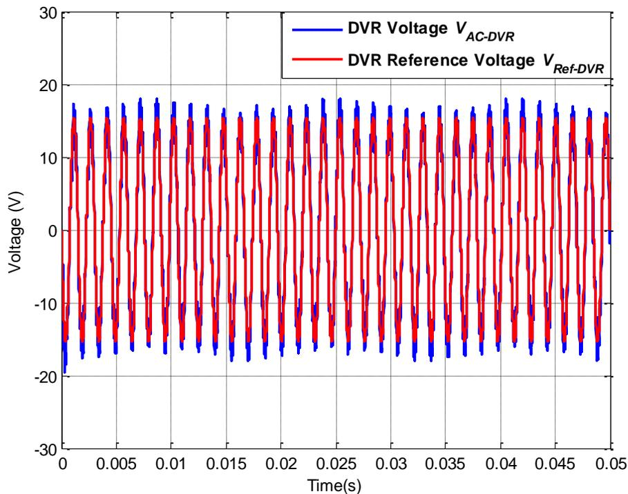
Figure A.19: AC-DVR voltage  $V_{AC-DVR}$  and DVR reference voltage  $V_{Ref-DVR}$  for operating scenario vi
