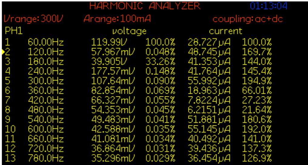
Figure 7.14: FFT of source voltage  $V_{in}$  for experiment scenario II
