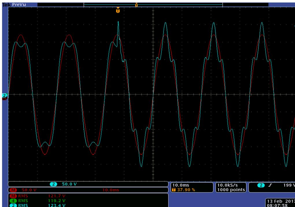
Figure 7.100: Experimental results of Source voltage  $V_{in}$  (Blue) and load reference voltage  $V_{Ref-Load}$  (Red) for experiment scenario XVII
