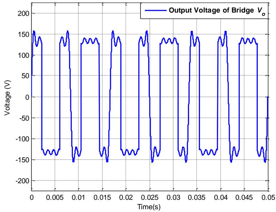
Figure 6.35: Bridge output voltage  $V_o$  for operating scenario IX
