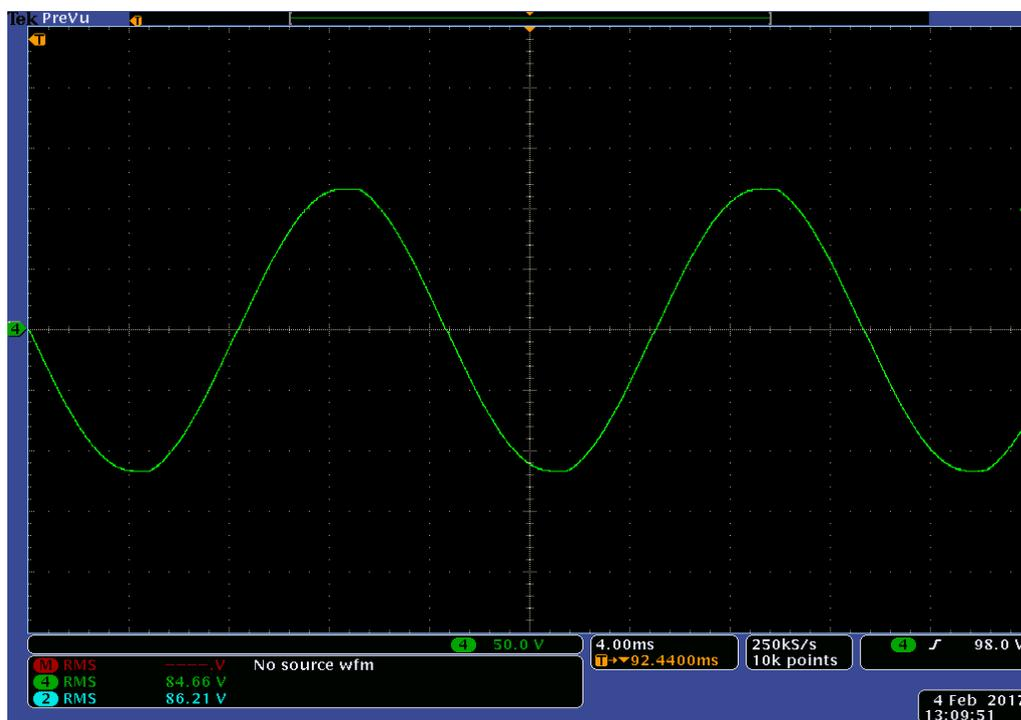
Figure 7.63: Experimental results of Bridge output voltage  $V_o$  for experiment scenario X
