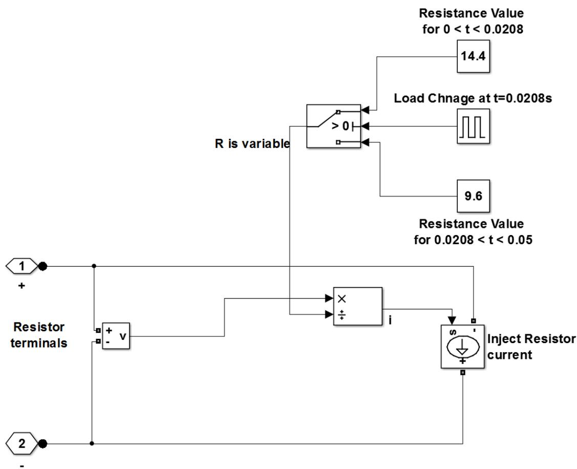
Figure 5.8: Model of variable resistive load
