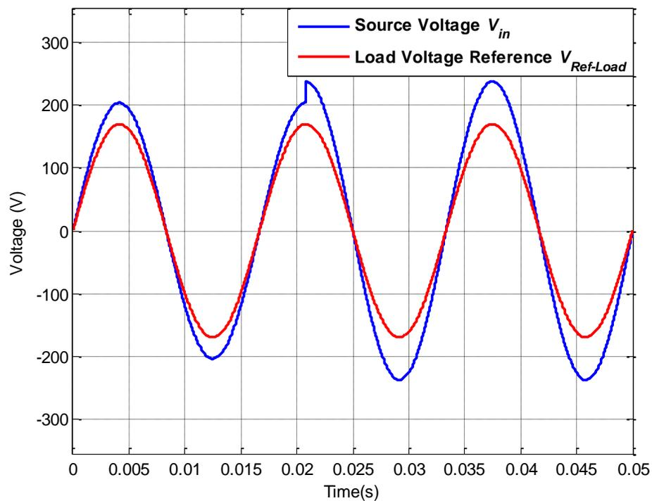
Figure 6.74: Source voltage  $V_{in}$  and load reference voltage  $V_{Ref-Load}$  for operating scenario XVI
