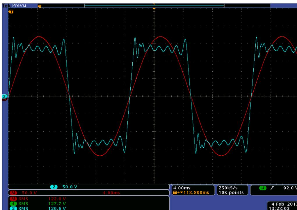
Figure 7.52: Experimental results of Source voltage  $V_{in}$  (Blue) and load reference voltage  $V_{Ref-Load}$  (Red) for experiment scenario IX
