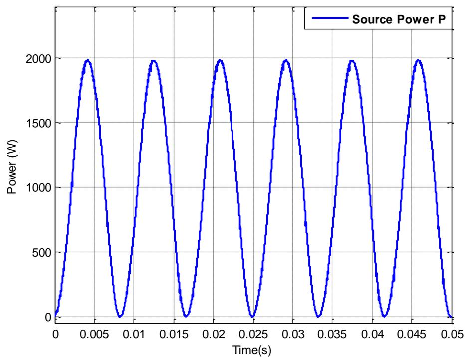
Figure A.14: Grid power for operating scenario ii
