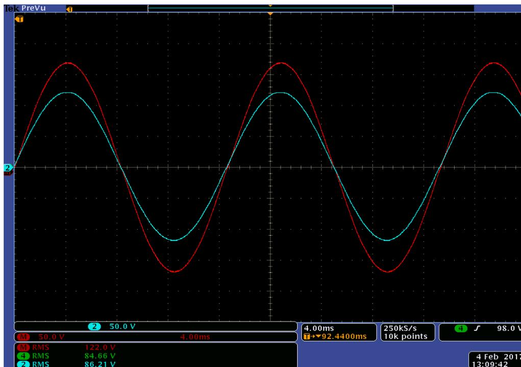
Figure 7.60: Experimental results of Source voltage  $V_{in}$  (Blue) and load reference voltage  $V_{Ref-Load}$  (Red) for experiment scenario X
