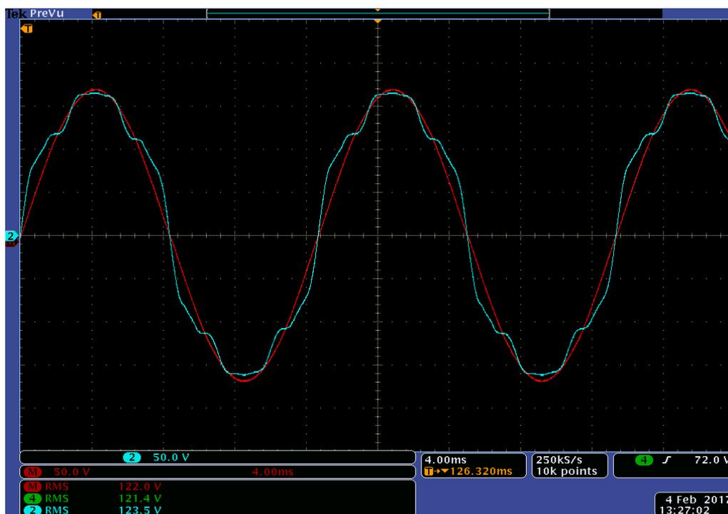
Figure 7.40: Experimental results of Source voltage  $V_{in}$  (Blue) and load reference voltage  $V_{Ref-Load}$  (Red) for experiment scenario VIII
