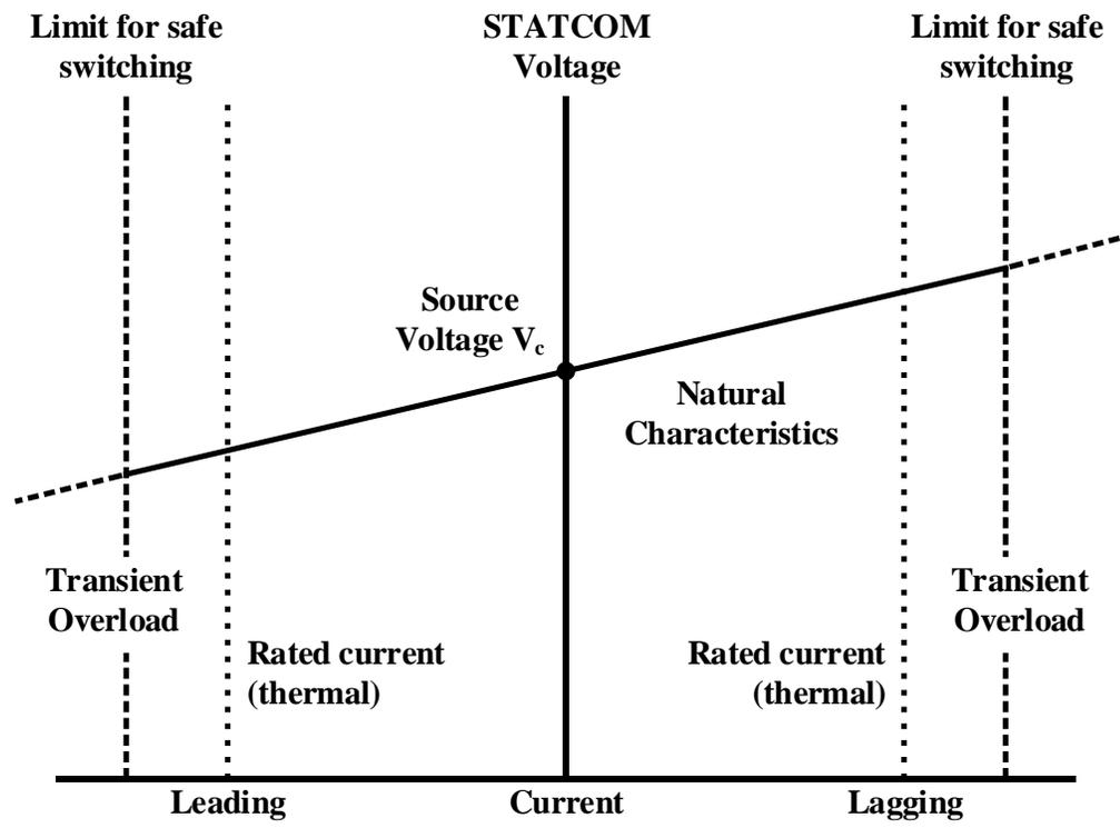
Figure 2.6: Natural characteristic of D-STATCOM
