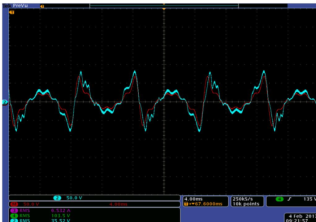
Figure 7.56: Experimental results of AC-DVR voltage  $V_{AC-DVR}$  (Blue) and DVR reference voltage  $V_{Ref-DVR}$  (Red) for experiment scenario IX
