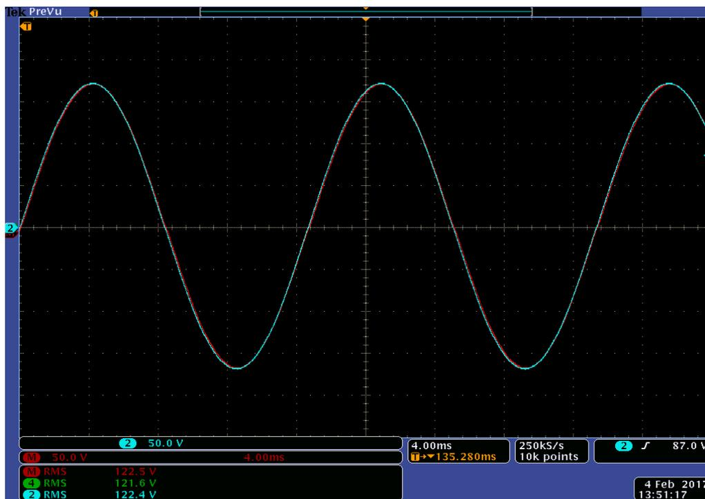
Figure 7.4: Experimental results of Source voltage  $V_{in}$  (Blue) and load reference voltage  $V_{Ref-Load}$  (Red) for experiment scenario I
