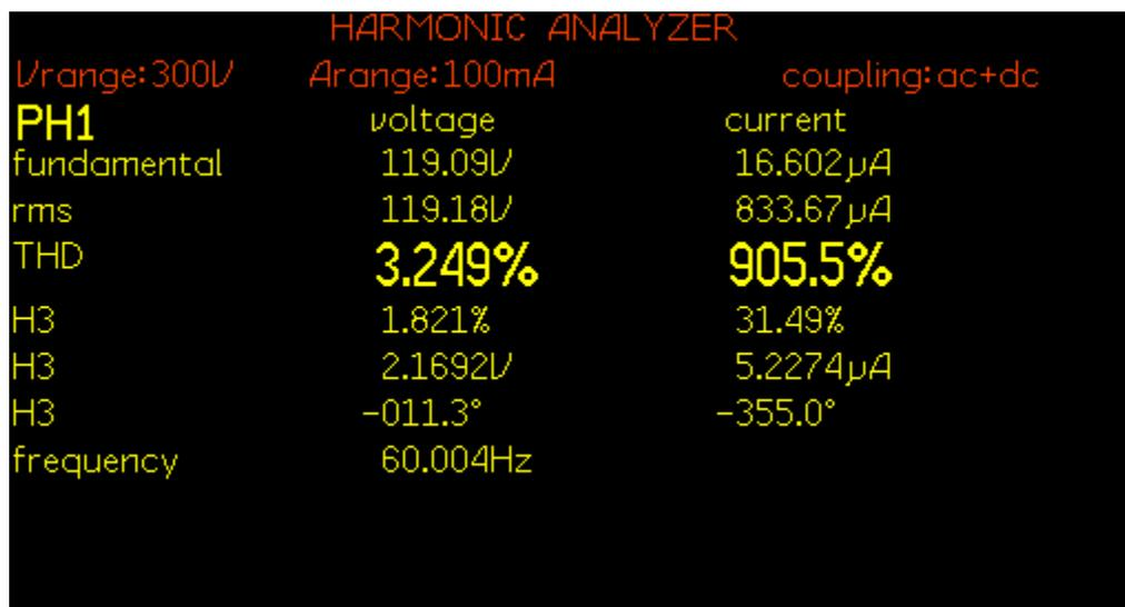
Figure 7.90: THD of load voltage  $V_{Load}$  for experiment scenario XIII
