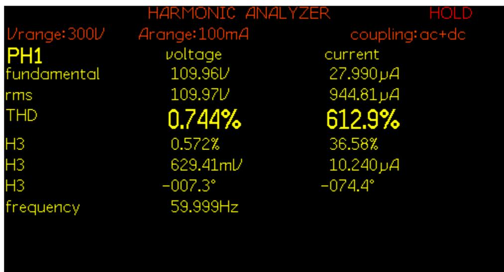
Figure 7.10: THD of load voltage  $V_{Load}$  for experiment scenario I
