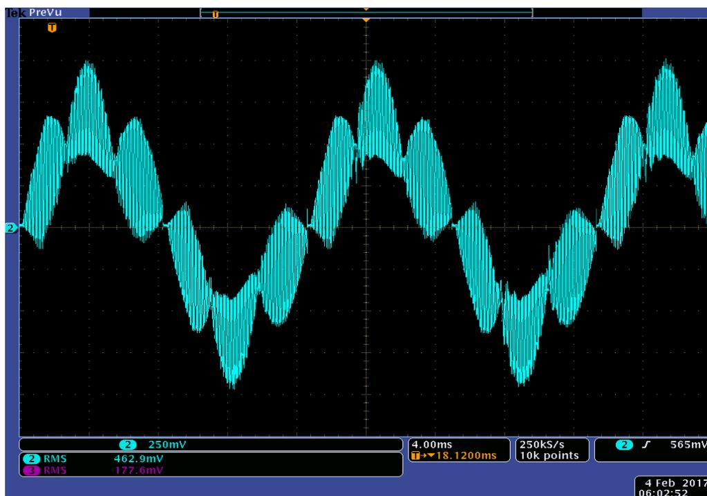
Figure 7.22: Experimental Results of Actual inductor current  $I_L$  for experiment scenario II
