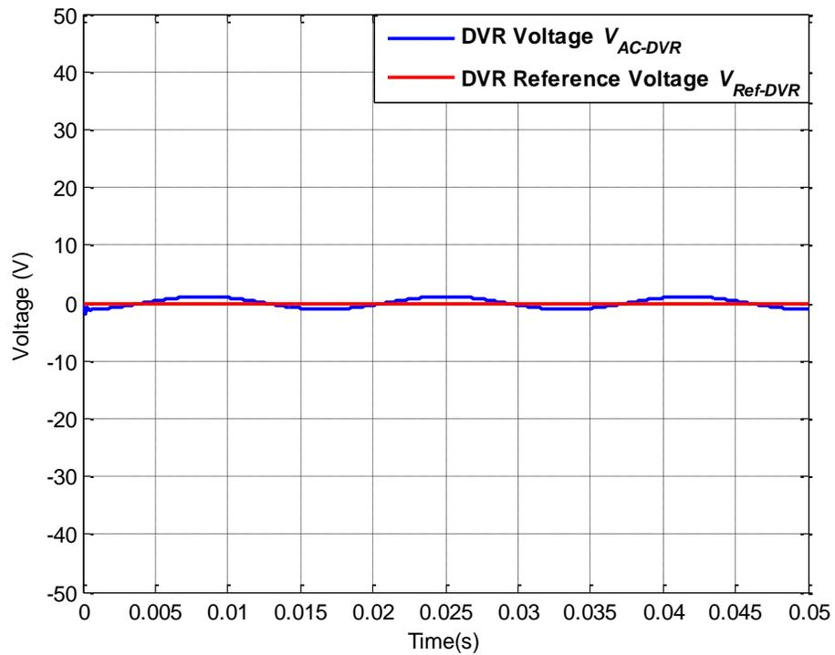
Figure 6.3 AC-DVR voltage  $V_{AC-DVR}$  and DVR reference voltage  $V_{Ref-DVR}$  for operating scenario I
