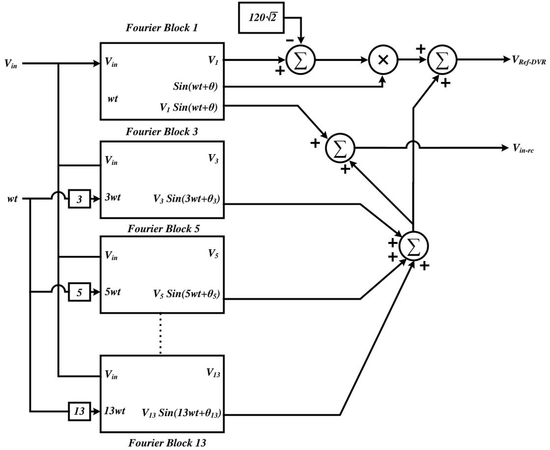
Figure 4.3: Block diagram of OSR (Original Signal Reconstruction) block
