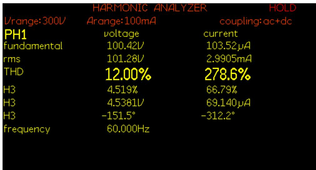
Figure 7.58: THD of load voltage  $V_{Load}$  for experiment scenario IX
