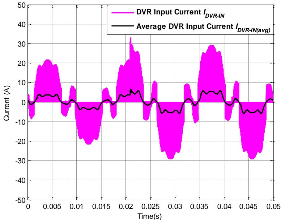
Figure A.60: Actual DVR current  $I_{DVR-IN}$  and average DVR current  $I_{DVR-IN(avg)}$  for operating scenario xv
