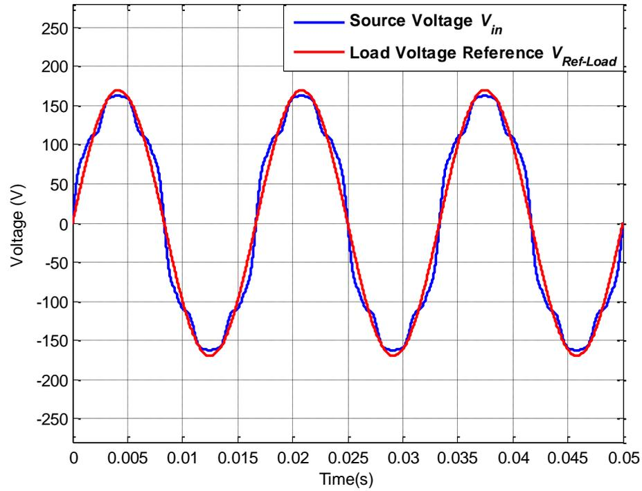
Figure 6.24: Source voltage  $V_{in}$  and load reference voltage  $V_{Ref-Load}$  for operating scenario VIII
