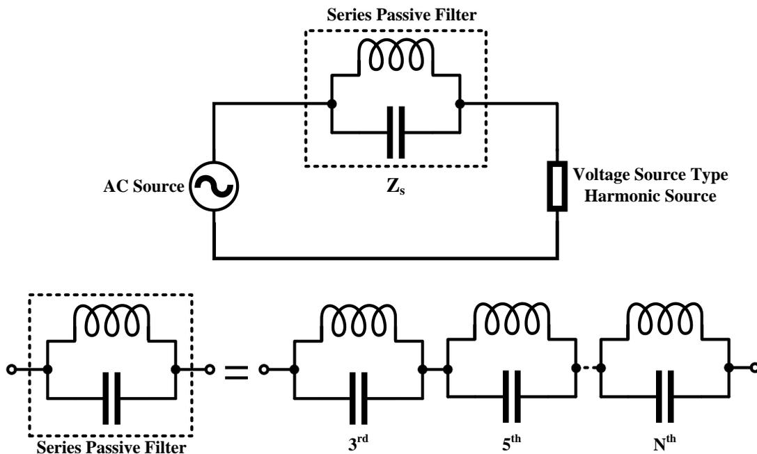
Figure 2.14: Series Passive Filter (SPF) schematic [44]
