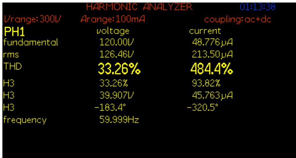
Figure 7.13: THD of source voltage  $V_{in}$  for experiment scenario II
