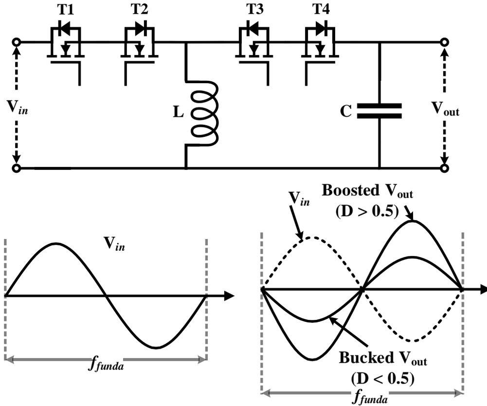
Figure 3.1: Schematic and operating principle of AC-AC buck boost converter
