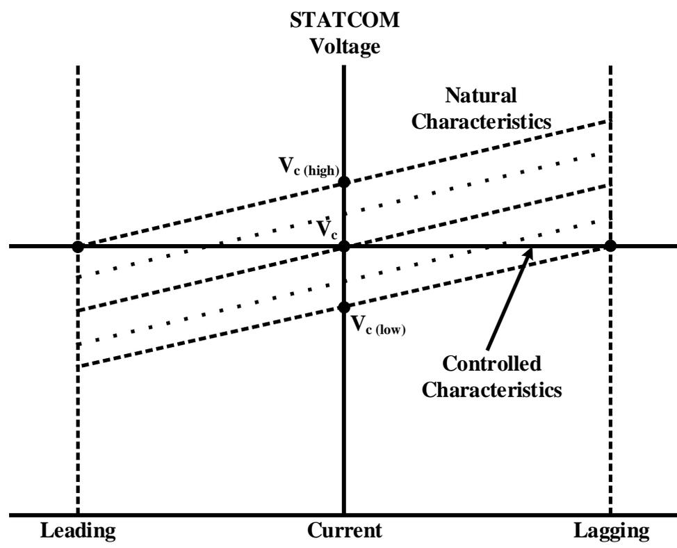
Figure 2.7: Controlled characteristic of D-STATCOM
