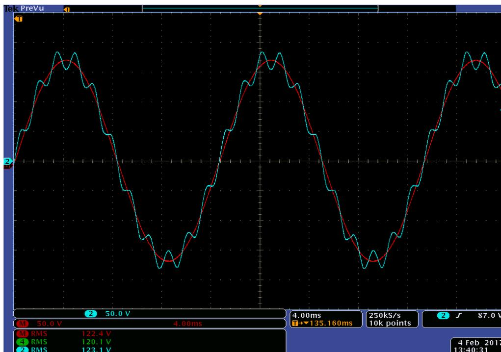
Figure 7.32: Experimental results of Source voltage  $V_{in}$  (Blue) and load reference voltage  $V_{Ref-Load}$  (Red) for experiment scenario VI
