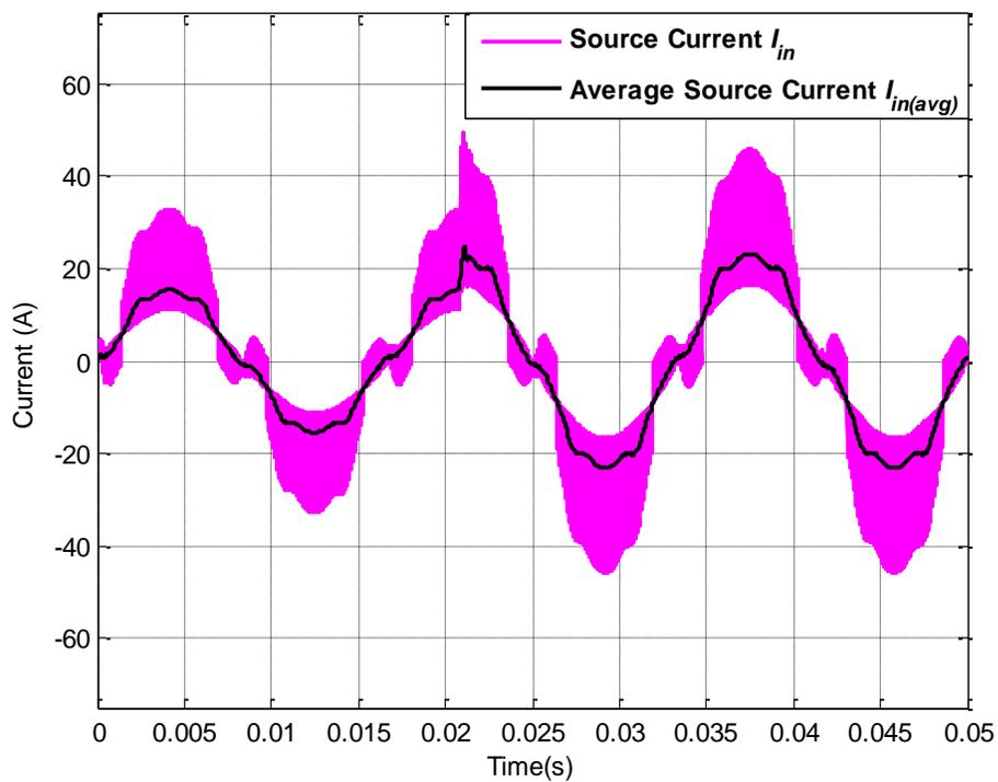
Figure A.59: Actual source current  $I_{in}$  and average source current  $I_{in(avg)}$  for operating scenario xv
