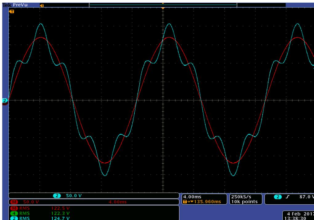
Figure 7.24: Experimental results of Source voltage  $V_{in}$  (Blue) and load reference voltage  $V_{Ref-Load}$  (Red) for experiment scenario III
