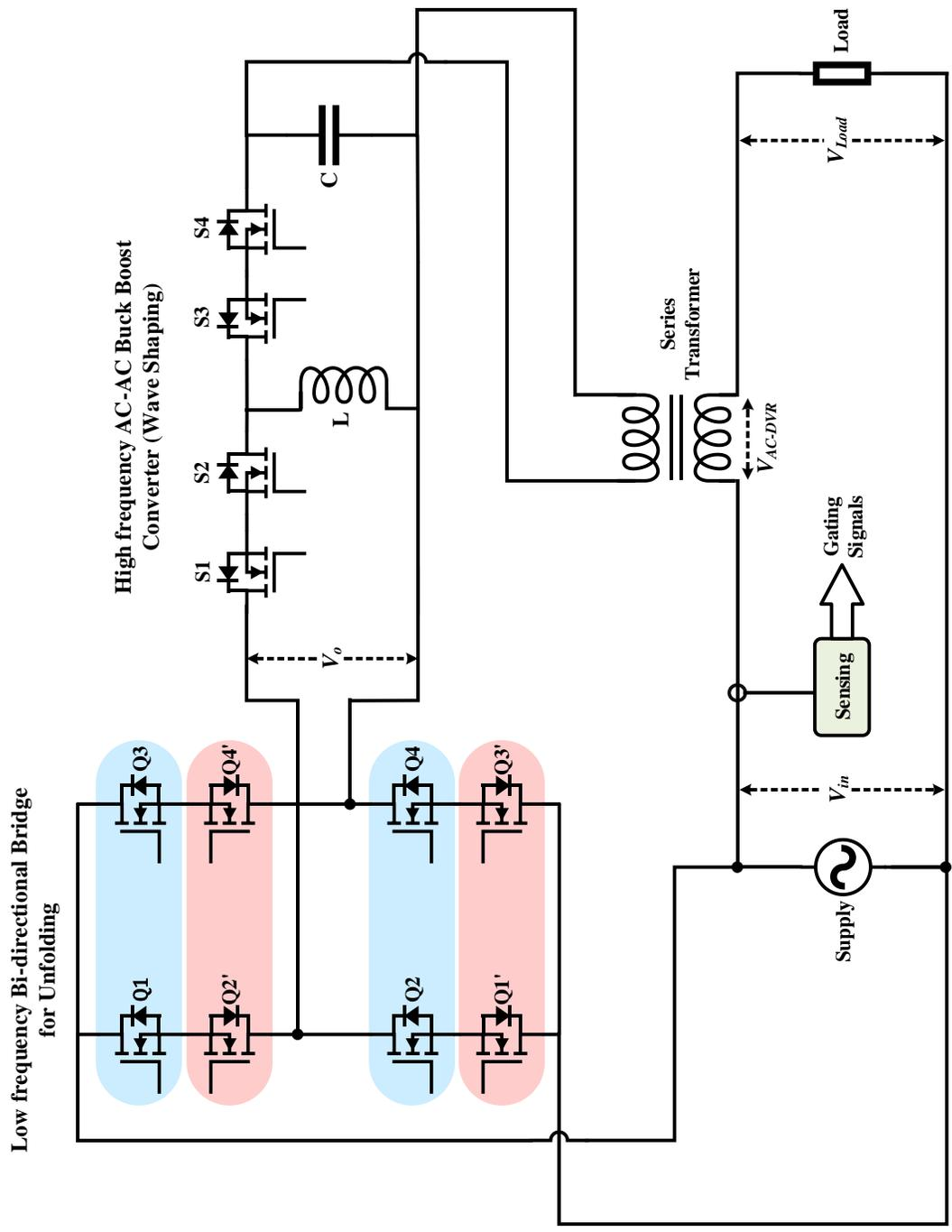
Figure 3.5 Detailed schematic of buck boost based AC-AC Dynamic Voltage Regulator (AC-DVR)
