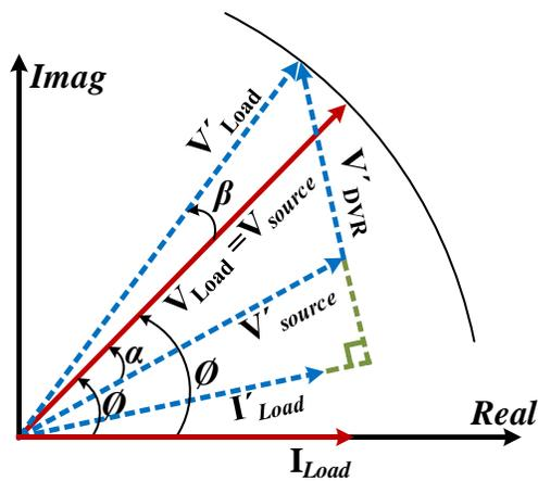
Figure 2.11: Energy minimized compensation phasor diagram
