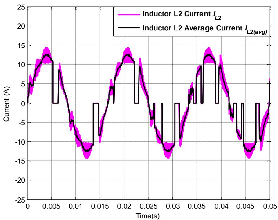
Figure A.49: Actual inductor current  $I_L$  and average inductor current  $I_{L(avg)}$  for operating scenario xiii
