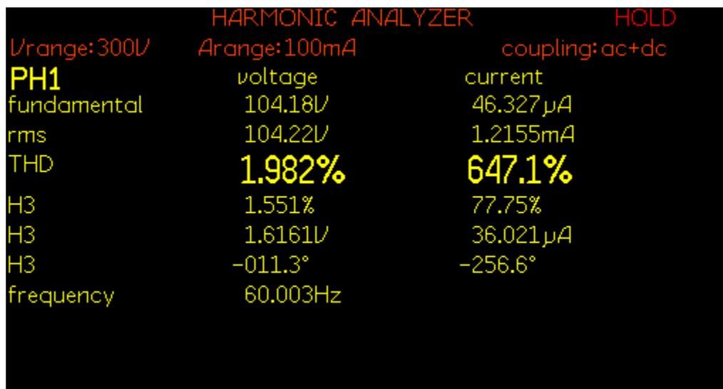
Figure 7.66: THD of load voltage  $V_{Load}$  for experiment scenario X
