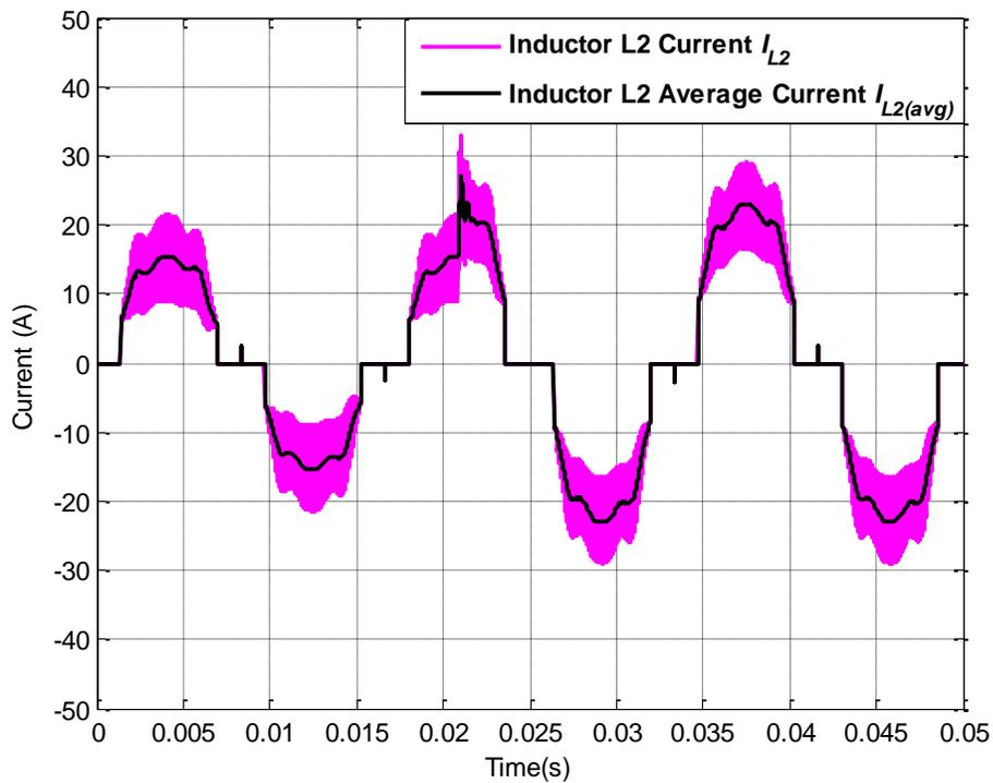
Figure A.62: Actual inductor current  $I_L$  and average inductor current  $I_{L(avg)}$  for operating scenario xv
