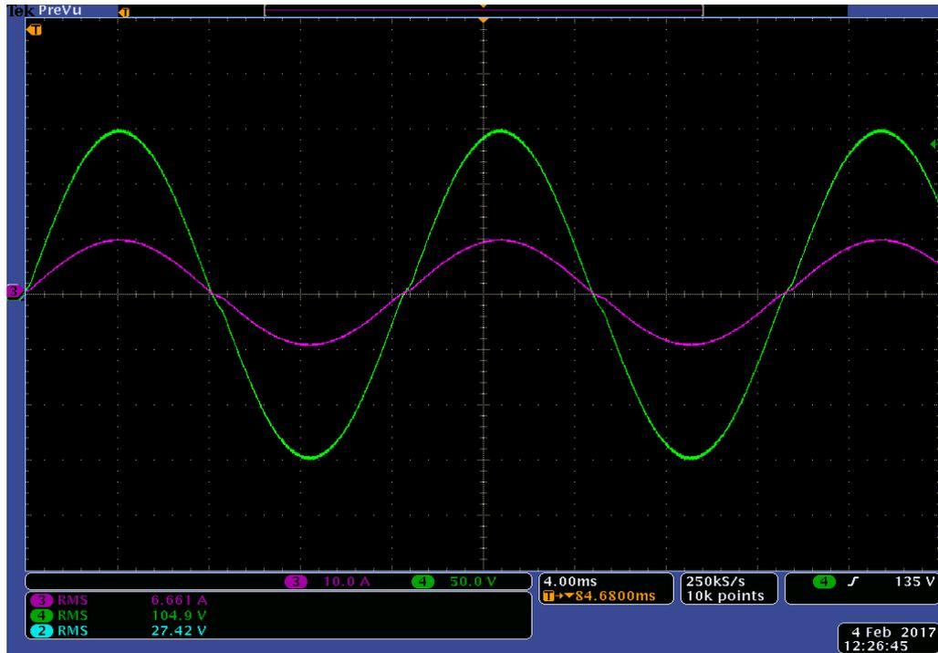
Figure 7.65: Experimental Results of Load voltage  $V_{Load}$  (Green) and load current  $I_{Load}$  (Pink) for experiment scenario X
