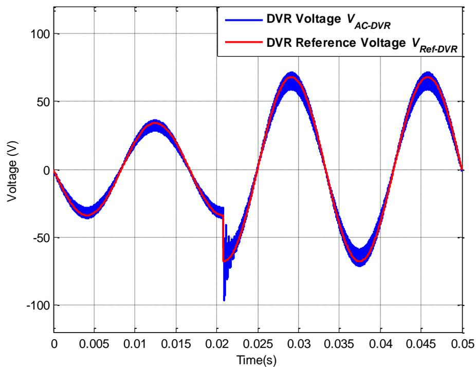
Figure A.67: AC-DVR voltage  $V_{AC-DVR}$  and DVR reference voltage  $V_{Ref-DVR}$  for operating scenario xvi
