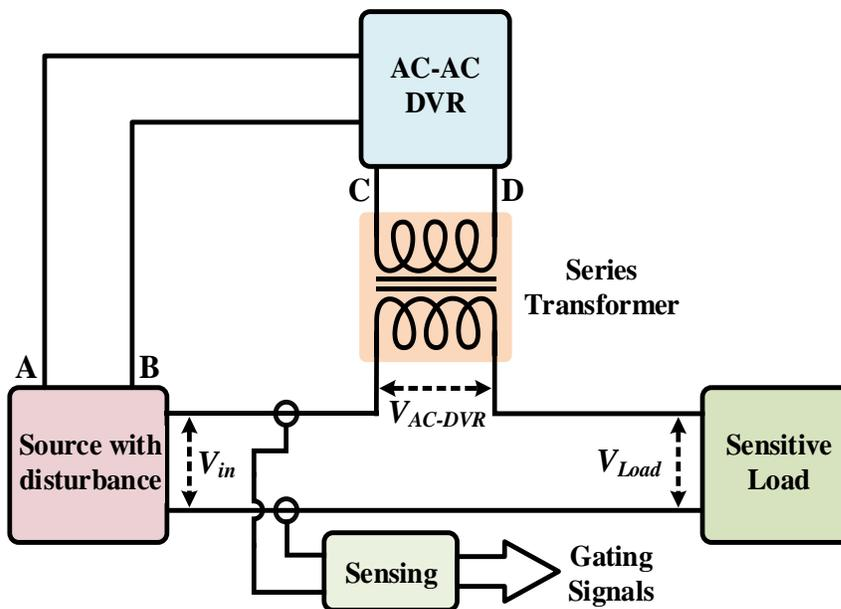
Figure 3.4: AC-DVR connection with source and load
