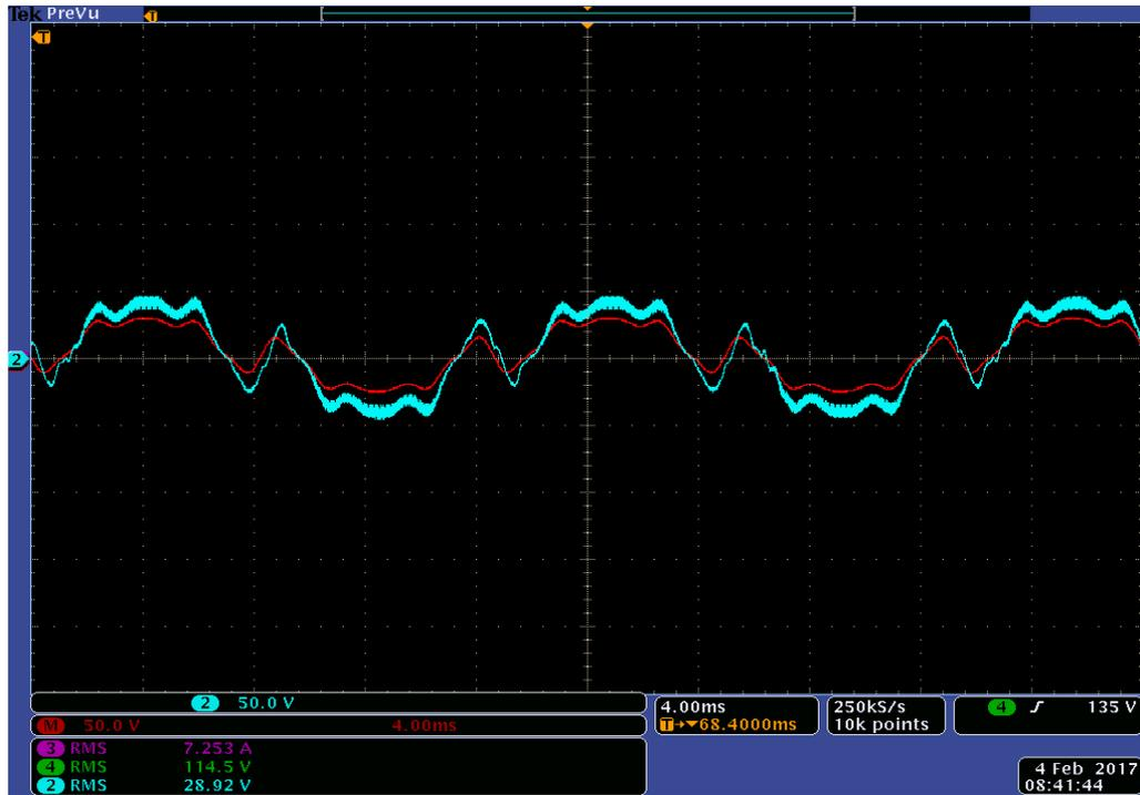
Figure 7.80: Experimental results of AC-DVR voltage  $V_{AC-DVR}$  (Blue) and DVR reference voltage  $V_{Ref-DVR}$  (Red) for experiment scenario XII
