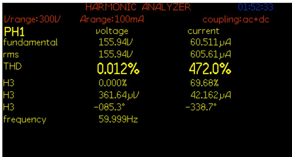
Figure 7.69: THD of source voltage  $V_{in}$  for experiment scenario XI
