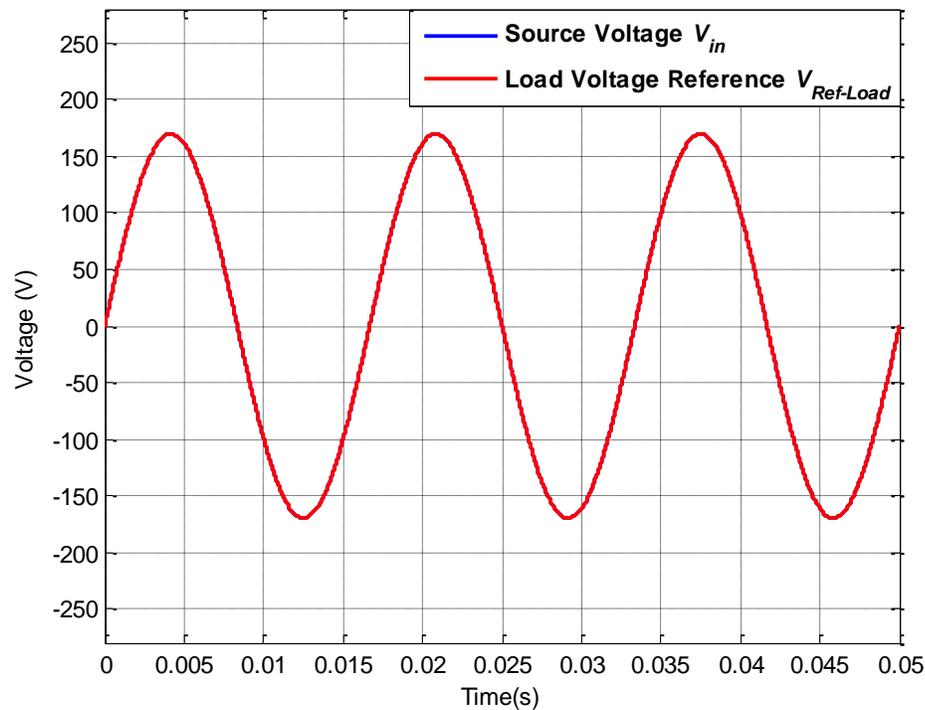
Figure A.2: Source voltage  $V_{in}$  and load reference voltage  $V_{Ref-Load}$  for operating scenario i
