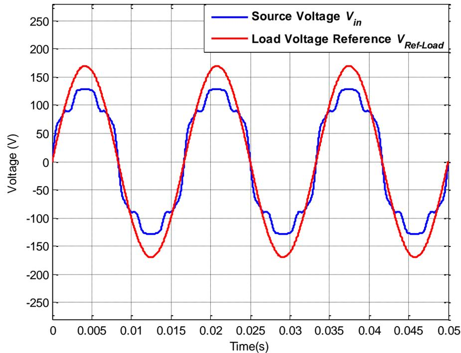
Figure 6.64: Source voltage  $V_{in}$  and load reference voltage  $V_{Ref-Load}$  for operating scenario XV
