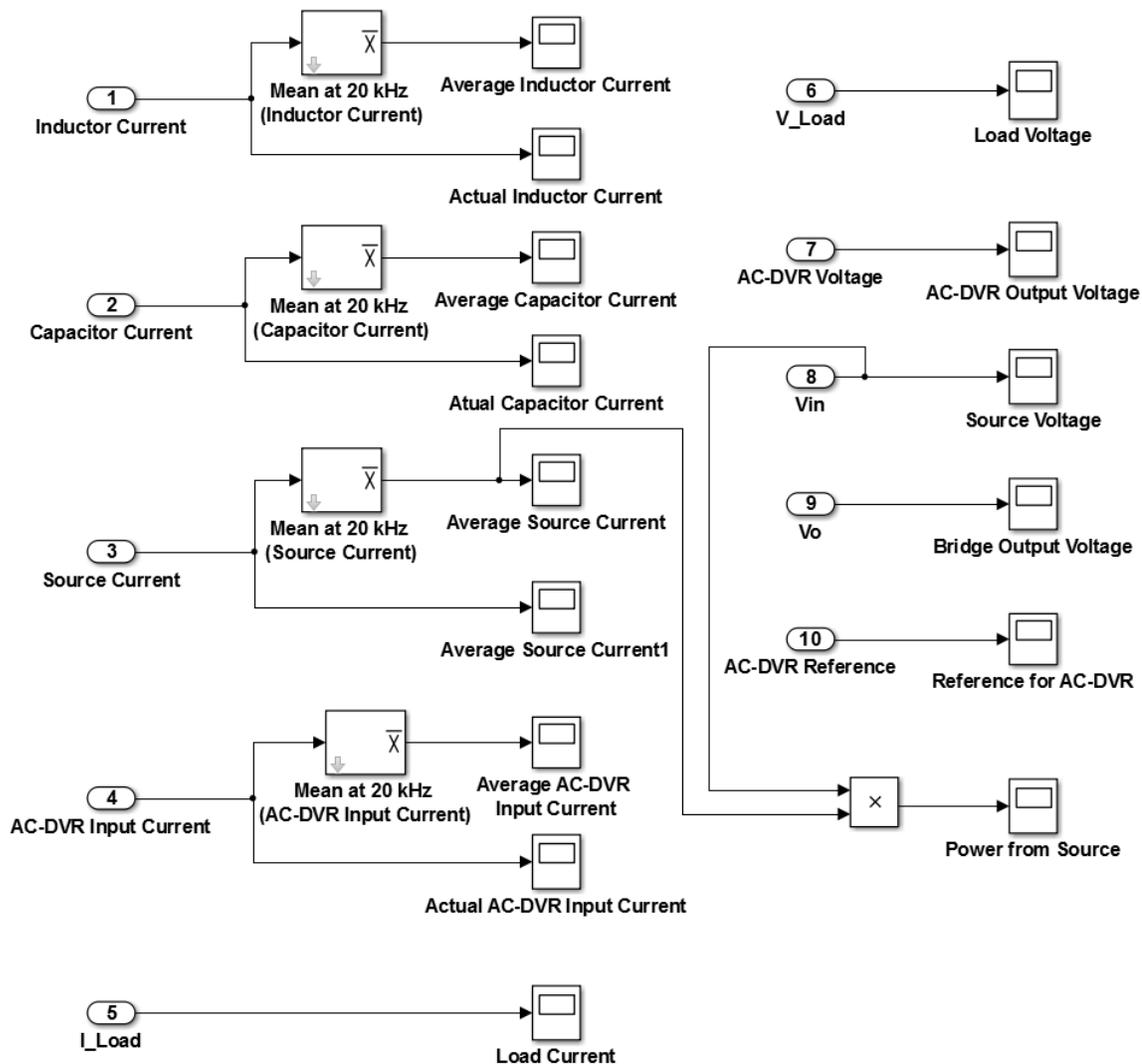
Figure 5.10: Scopes for voltage, current and power measurements
