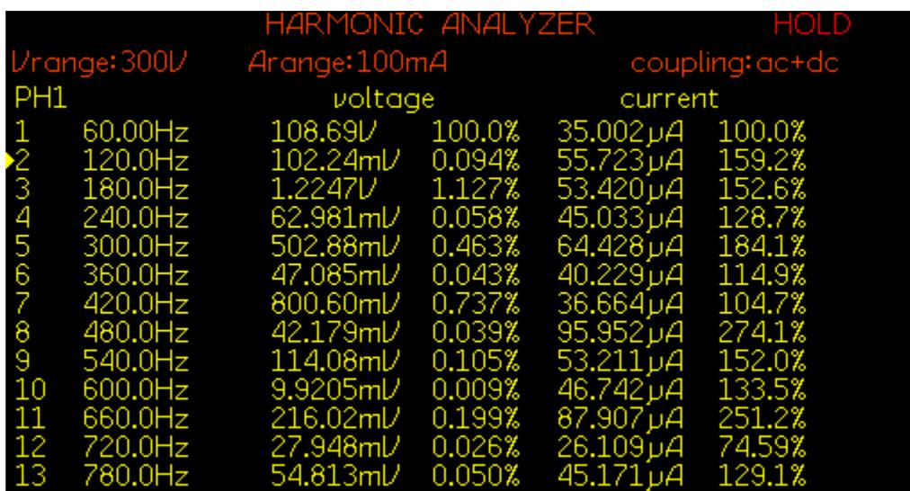
Figure 7.109: FFT-3<sup>rd</sup> of load voltage  $V_{Load}$  for experiment scenario XVII
