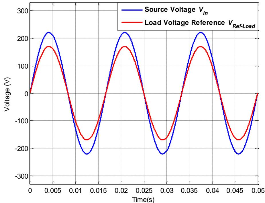
Figure 6.42: Source voltage  $V_{in}$  and load reference voltage  $V_{Ref-Load}$  for operating scenario XI
