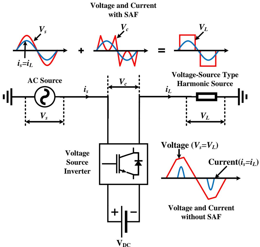
Figure 2.16: Series Active Filter (SAF) schematic and operation
