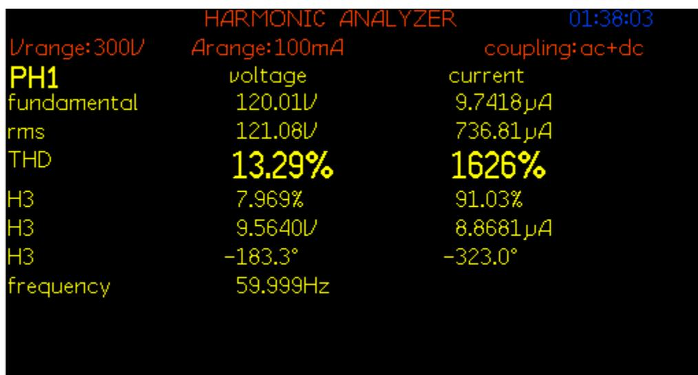
Figure 7.41: THD of source voltage  $V_{in}$  for experiment scenario VIII
