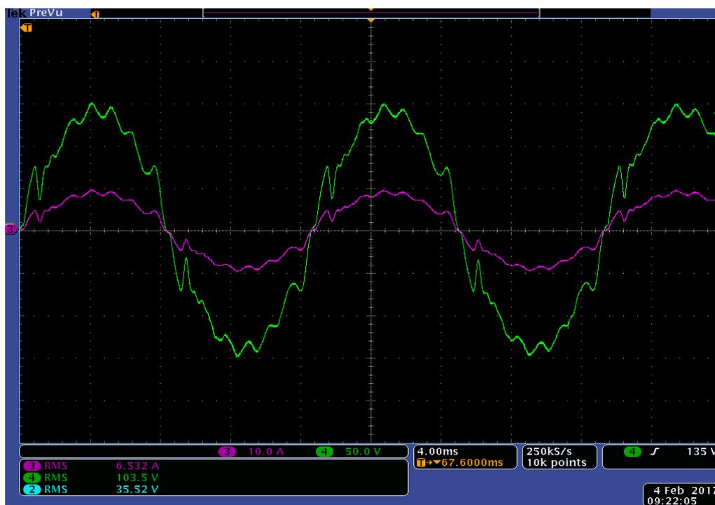
Figure 7.57: Experimental Results of Load voltage  $V_{Load}$  (Green) and load current  $I_{Load}$  (Pink) for experiment scenario IX
