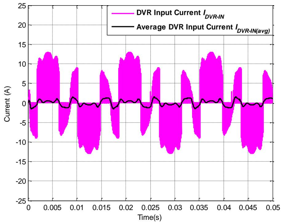
Figure 6.29: Actual DVR current  $I_{DVR-IN}$  and average DVR current  $I_{DVR-IN(avg)}$  for operating scenario VIII
