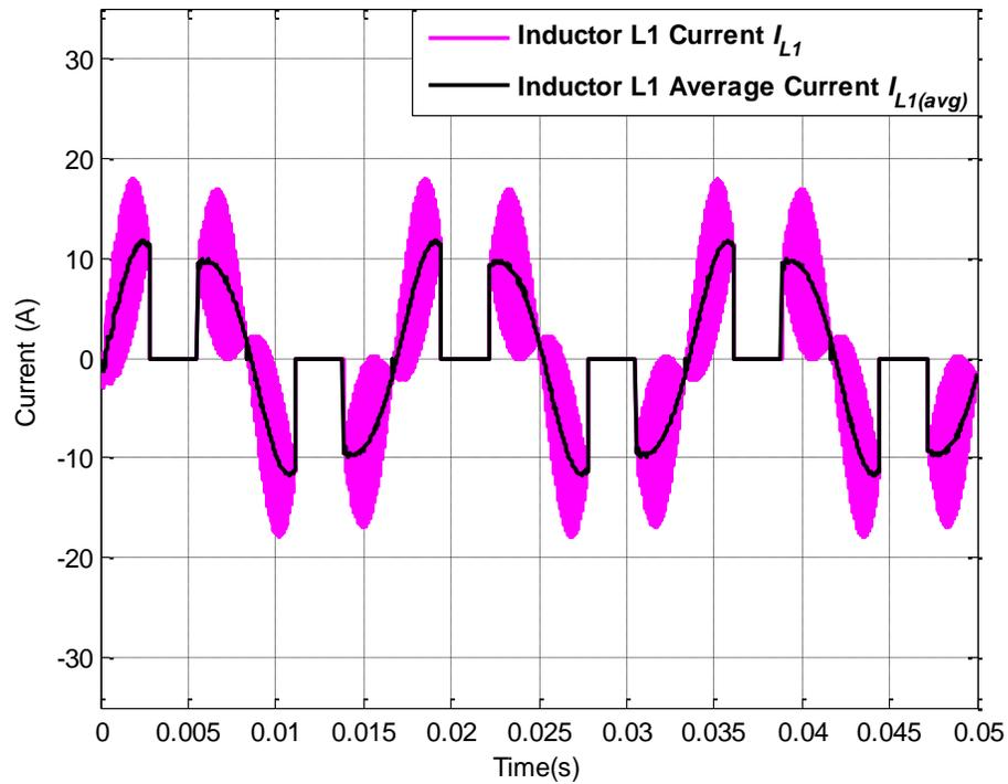
Figure A.10: Actual inductor current  $I_L$  and average inductor current  $I_{L(avg)}$  for operating scenario ii
