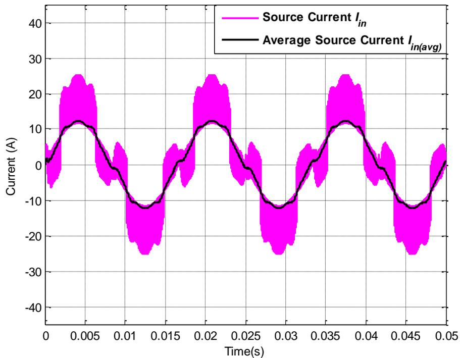
Figure A.24: Actual source current  $I_{in}$  and average source current  $I_{in(avg)}$  for operating scenario viii
