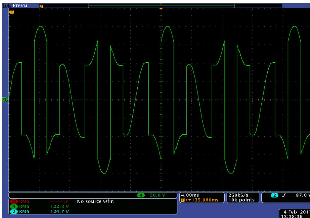
Figure 7.27: Experimental results of Bridge output voltage  $V_o$  for experiment scenario III
