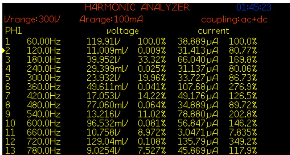
Figure 7.54: FFT of source voltage  $V_{in}$  for experiment scenario IX
