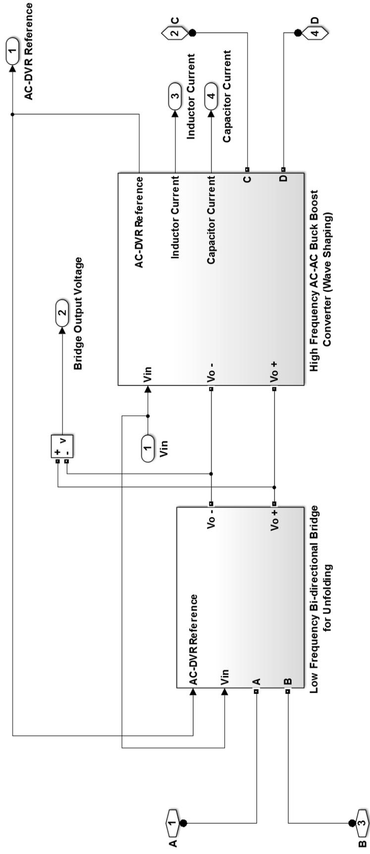
Figure 5.3: Model of proposed AC-DVR system architecture including Low Frequency Bidirectional Bridge and high frequency AC-AC buck boost converter
