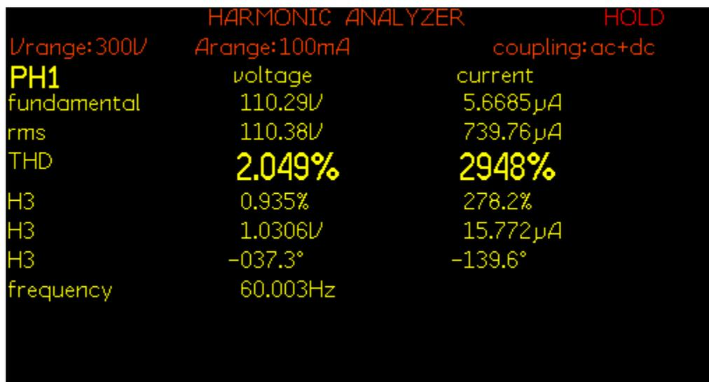
Figure 7.38: THD of load voltage  $V_{Load}$  for experiment scenario IV
