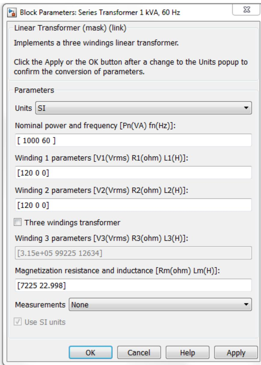
Figure 5.9: Series transformer parameters
