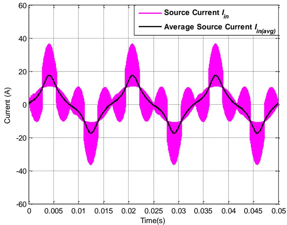
Figure A.8: Actual source current  $I_{in}$  and average source current  $I_{in(avg)}$  for operating scenario ii
