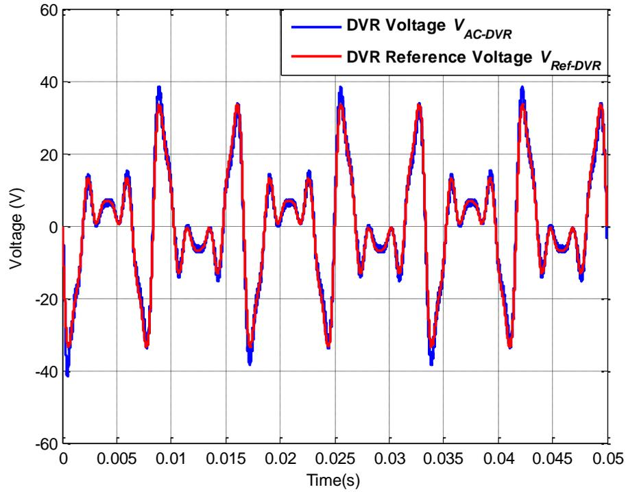
Figure 6.26: AC-DVR voltage  $V_{AC-DVR}$  and DVR reference voltage  $V_{Ref-DVR}$  for operating scenario VIII
