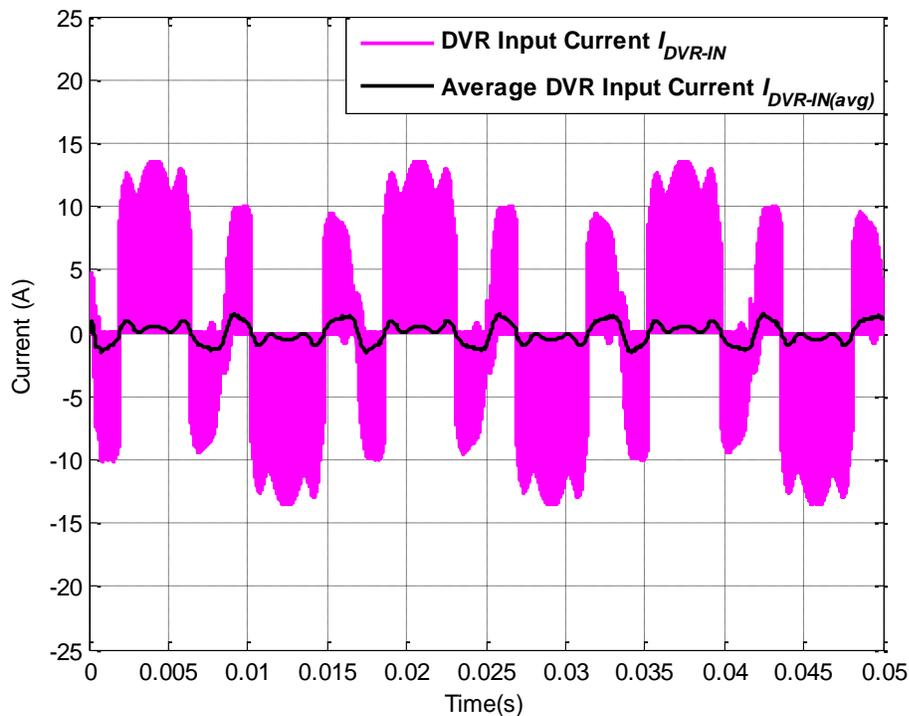
Figure A.25: Actual DVR current  $I_{DVR-IN}$  and average DVR current  $I_{DVR-IN(avg)}$  for operating scenario viii
