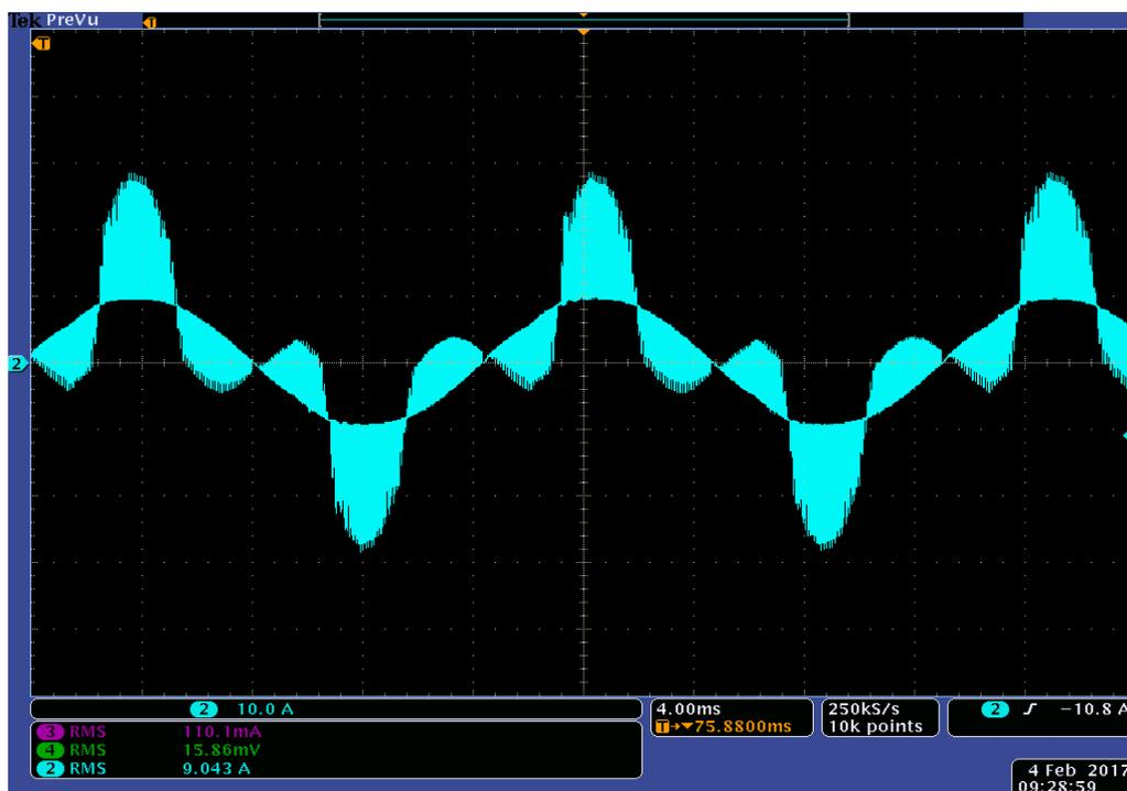
Figure 7.20: Experimental Results of Actual source current  $I_{in}$  for experiment scenario II
