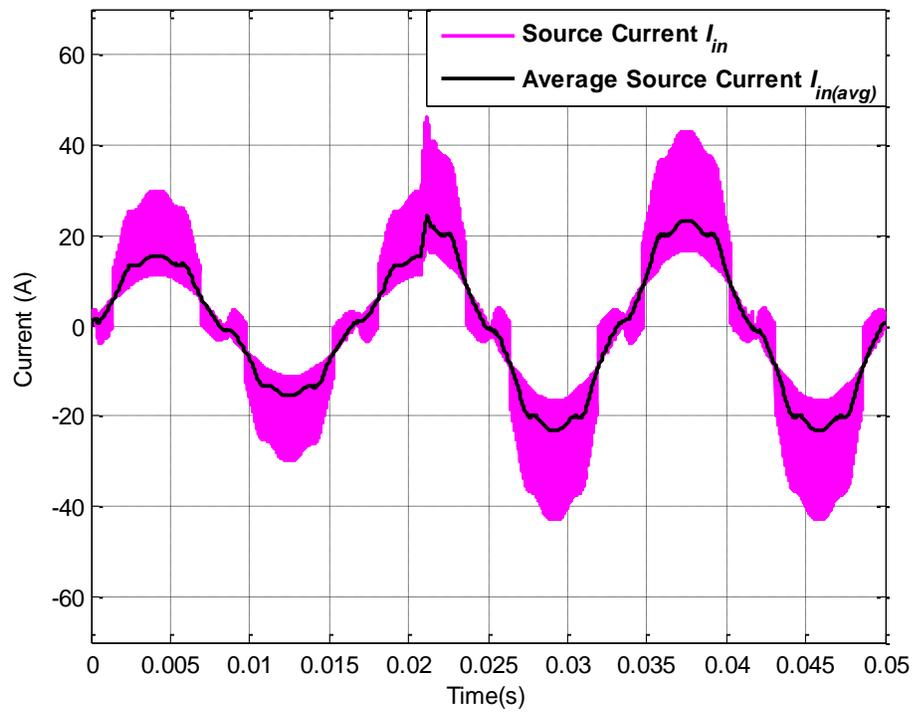
Figure 6.68: Actual source current  $I_{in}$  and average source current  $I_{in(avg)}$  for operating scenario XV
