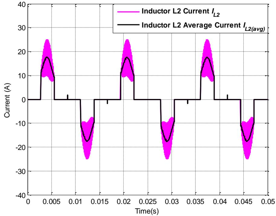
Figure A.11: Actual inductor current  $I_L$  and average inductor current  $I_{L(avg)}$  for operating scenario ii
