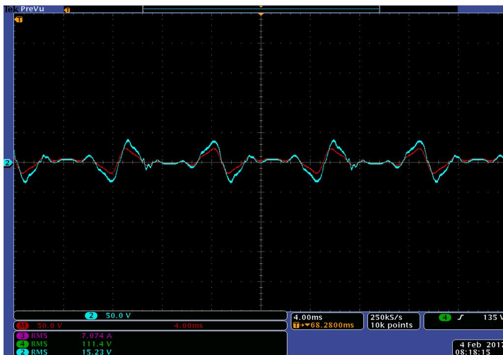
Figure 7.44: Experimental results of AC-DVR voltage  $V_{AC-DVR}$  (Blue) and DVR reference voltage  $V_{Ref-DVR}$  (Red) for experiment scenario VIII
