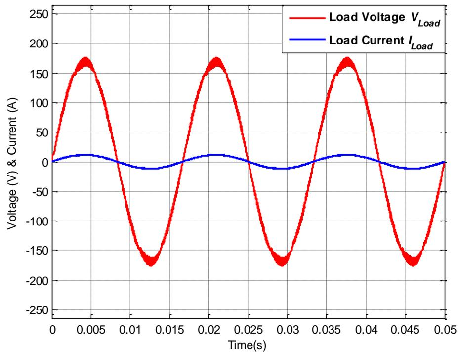
Figure 6.9: Load voltage  $V_{Load}$  and load current  $I_{Load}$  for operating scenario II
