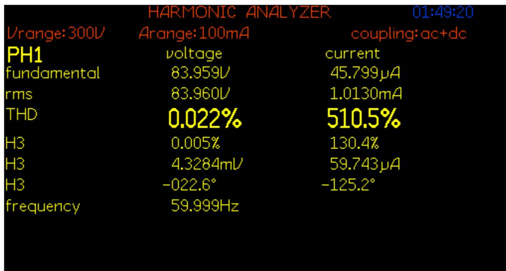
Figure 7.61: THD of source voltage  $V_{in}$  for experiment scenario X
