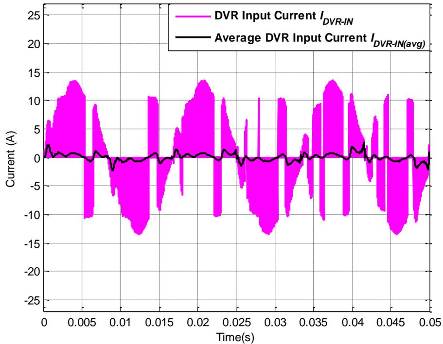
Figure 6.55: Actual DVR current  $I_{DVR-IN}$  and average DVR current  $I_{DVR-IN(avg)}$  for operating scenario XIII
