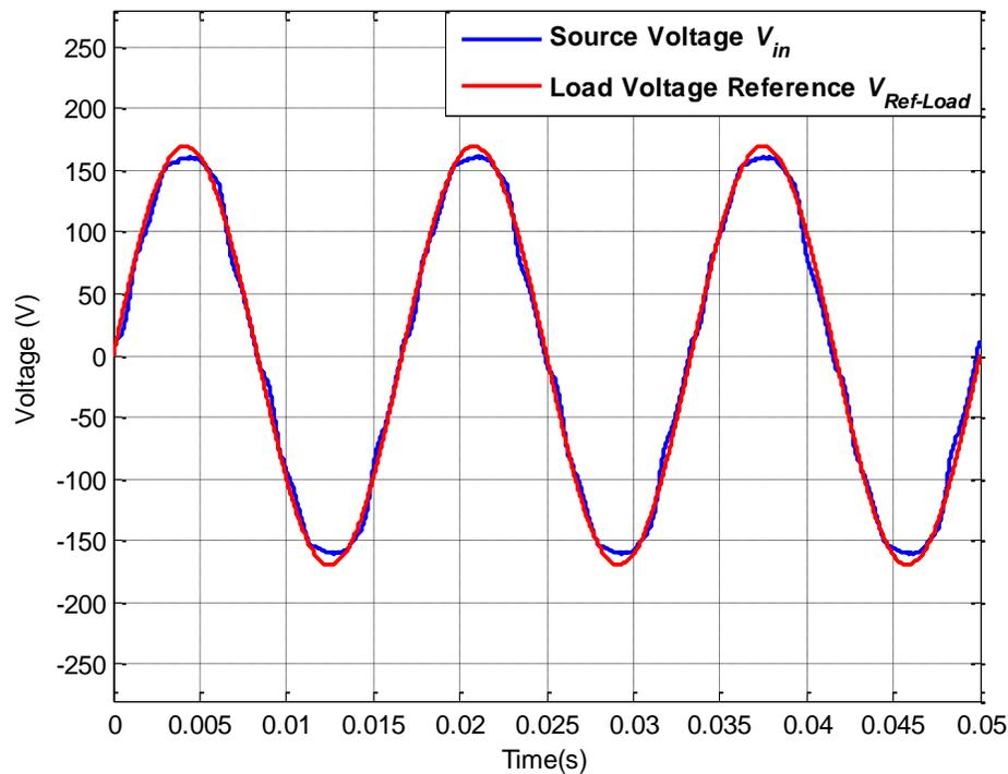
Figure A.43: Source voltage  $V_{in}$  and load reference voltage  $V_{Ref-Load}$  for operating scenario xiii
