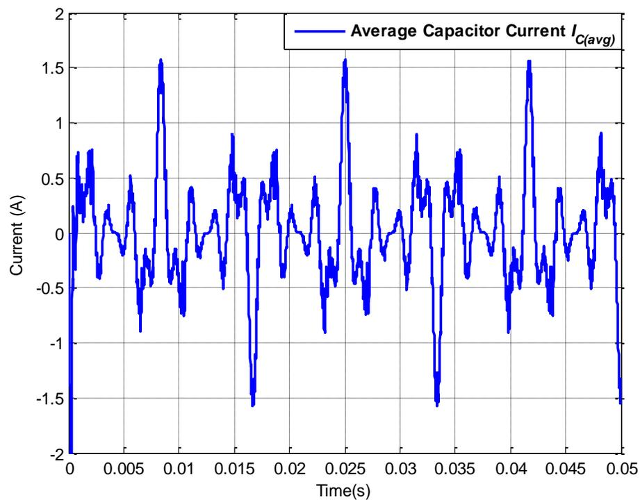
Figure A.29: Average capacitor current  $I_{C(avg)}$  for operating scenario viii
