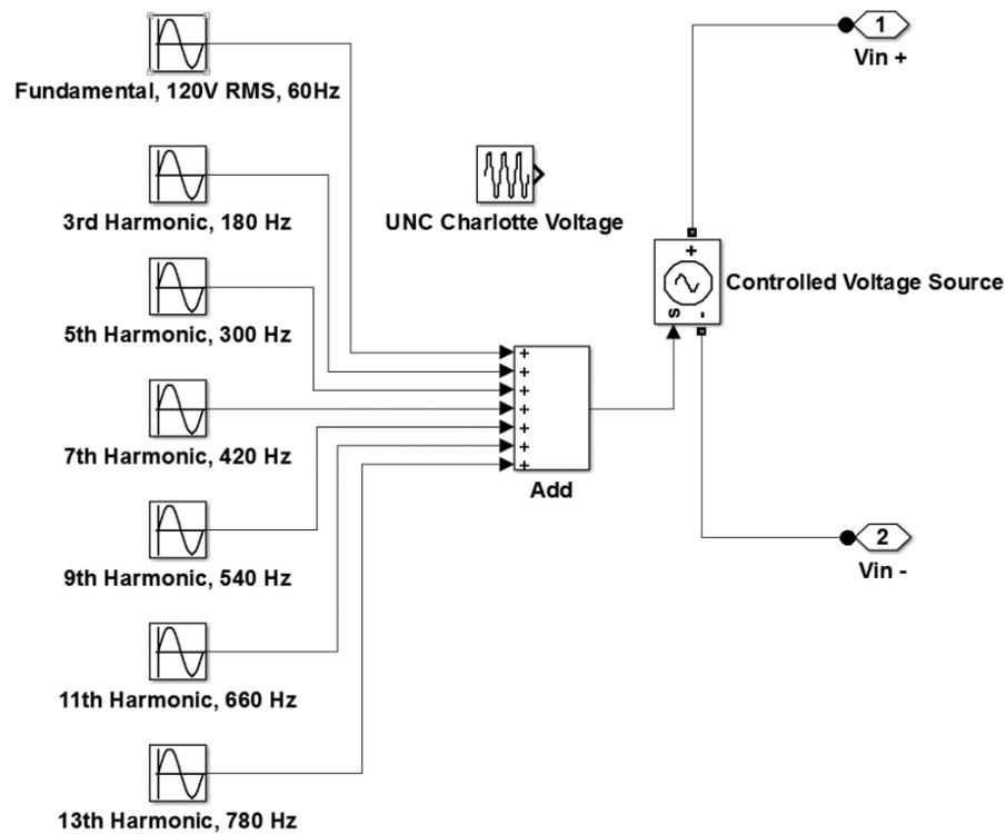
Figure 5.2: Model of unprotected source
