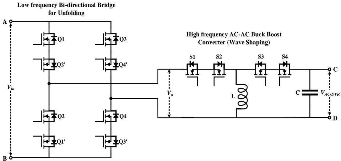
Figure 3.3: Proposed buck boost based AC-AC Dynamic Voltage Regulator (AC-DVR)
