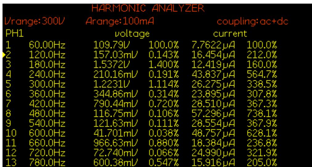
Figure 7.31: FFT of load voltage  $V_{Load}$  for experiment scenario III
