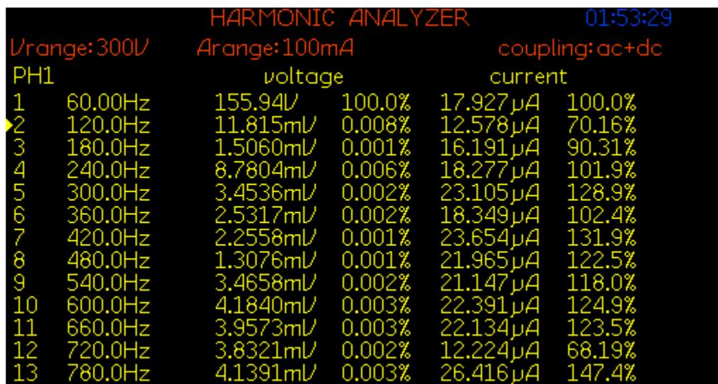
Figure 7.70: FFT of source voltage  $V_{in}$  for experiment scenario XI
