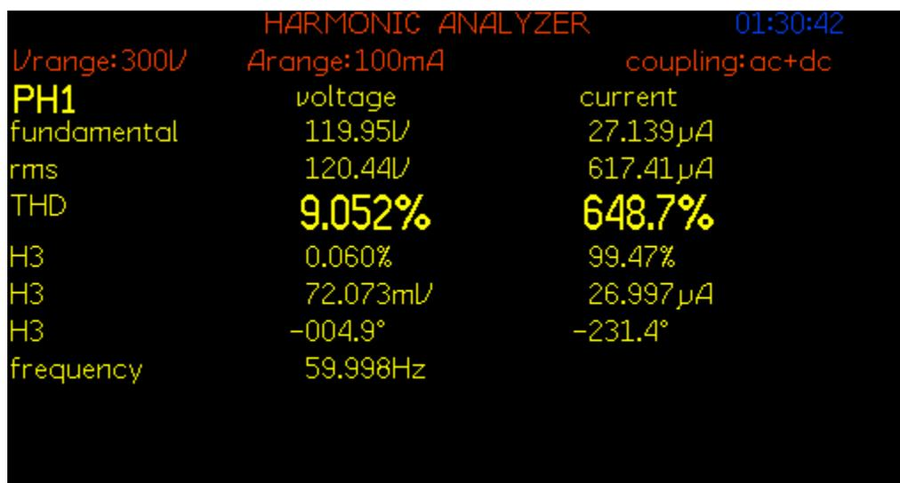
Figure 7.33: THD of source voltage  $V_{in}$  for experiment scenario IV
