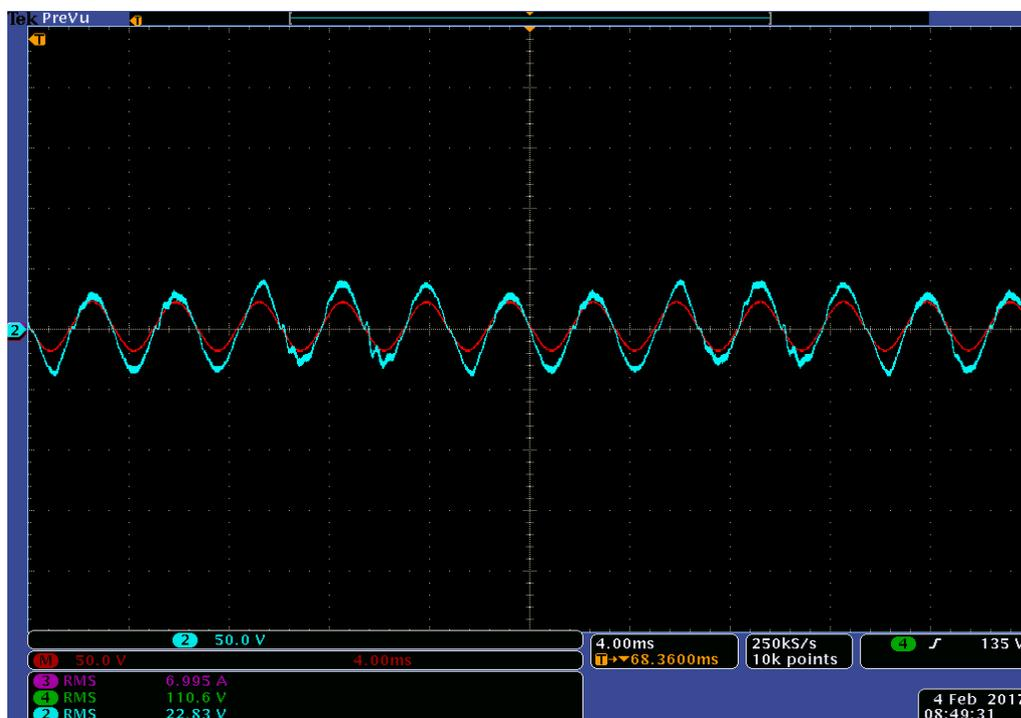
Figure 7.28: Experimental results of AC-DVR voltage  $V_{AC-DVR}$  (Blue) and DVR reference voltage  $V_{Ref-DVR}$  (Red) for experiment scenario III
