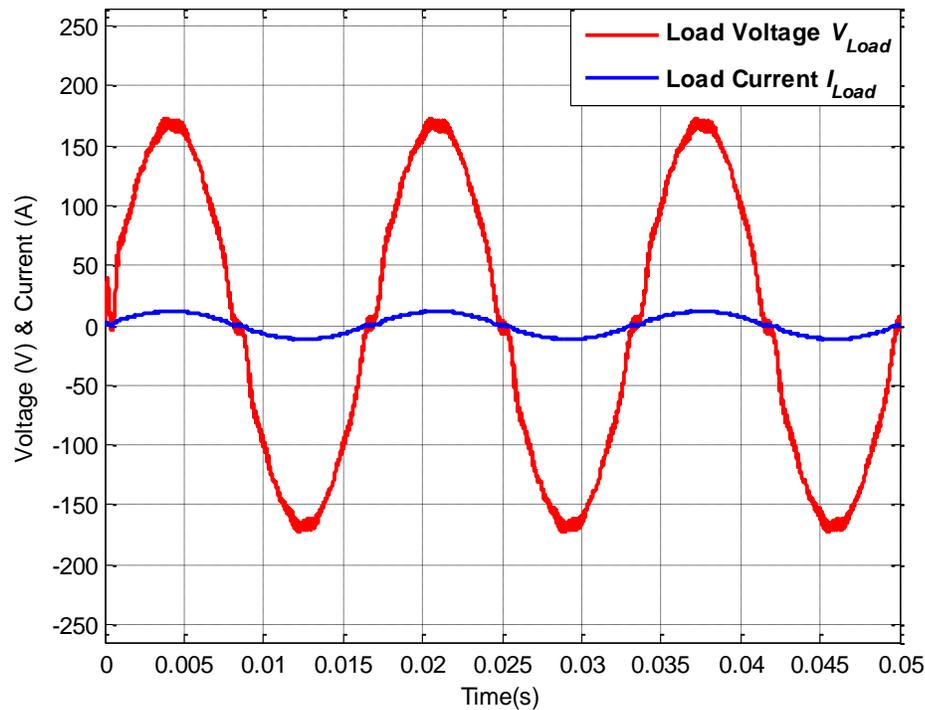
Figure 6.37: Load voltage  $V_{Load}$  and load current  $I_{Load}$  for operating scenario IX
