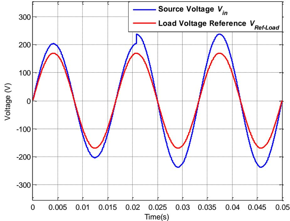
Figure A.66: Source voltage  $V_{in}$  and load reference voltage  $V_{Ref-Load}$  for operating scenario xvi
