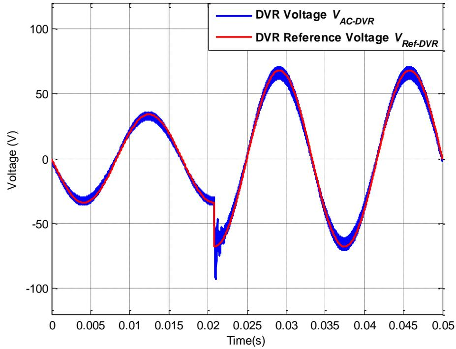
Figure 6.76: AC-DVR voltage  $V_{AC-DVR}$  and DVR reference voltage  $V_{Ref-DVR}$  for operating scenario XVI
