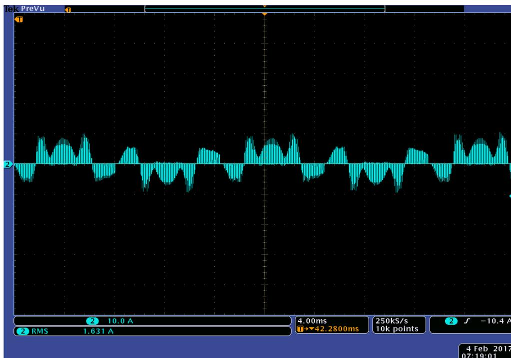
Figure 7.49: Experimental Results of Actual DVR current  $I_{DVR-IN}$  for experiment scenario VIII
