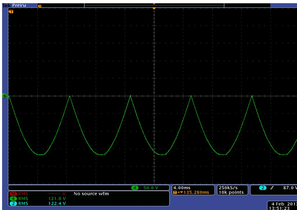
Figure 7.7: Experimental results of Bridge output voltage  $V_o$  for experiment scenario I
