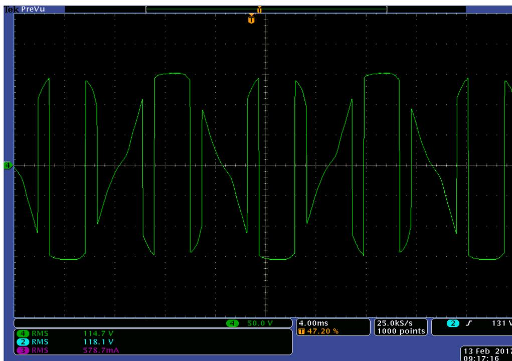
Figure 7.87: Experimental results of Bridge output voltage  $V_o$  for experiment scenario XIII
