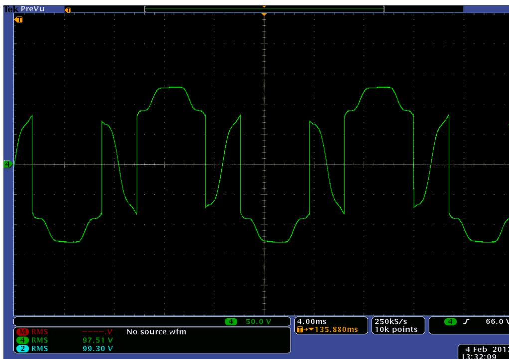
Figure 7.79: Experimental results of Bridge output voltage  $V_o$  for experiment scenario XII
