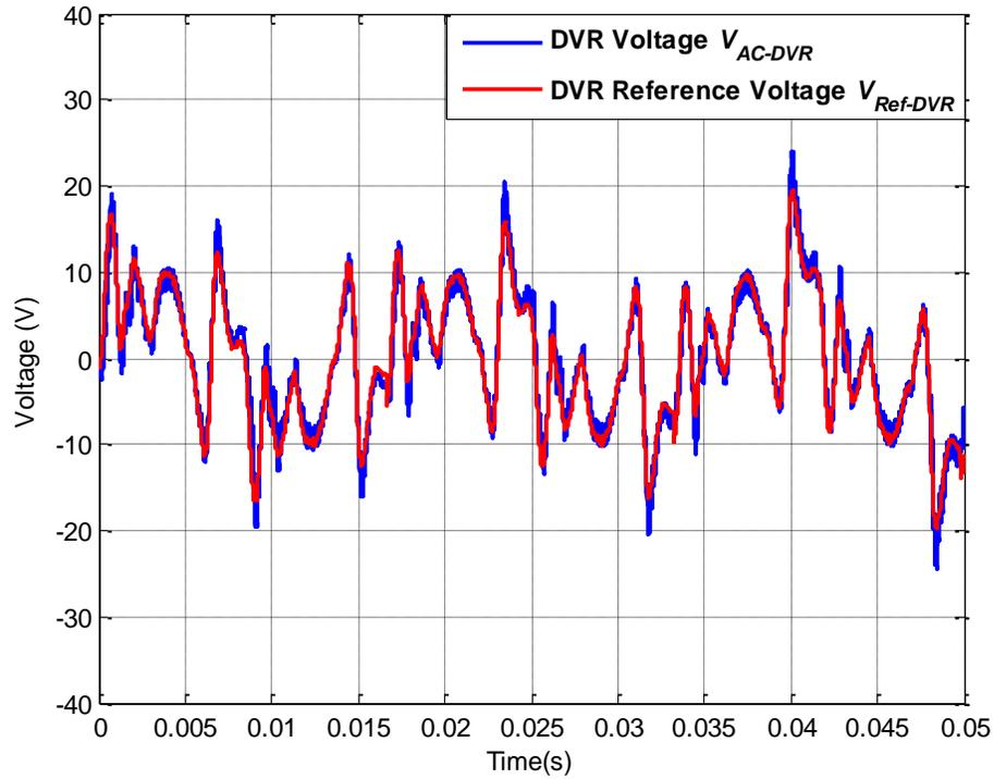
Figure 6.52: AC-DVR voltage  $V_{AC-DVR}$  and DVR reference voltage  $V_{Ref-DVR}$  for operating scenario XIII
