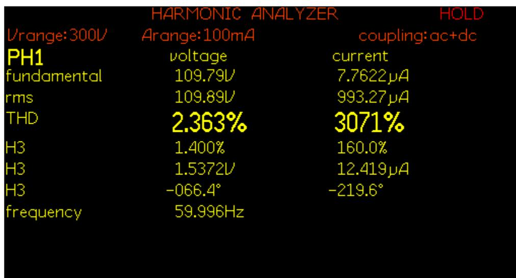
Figure 7.30: THD of load voltage  $V_{Load}$  for experiment scenario III
