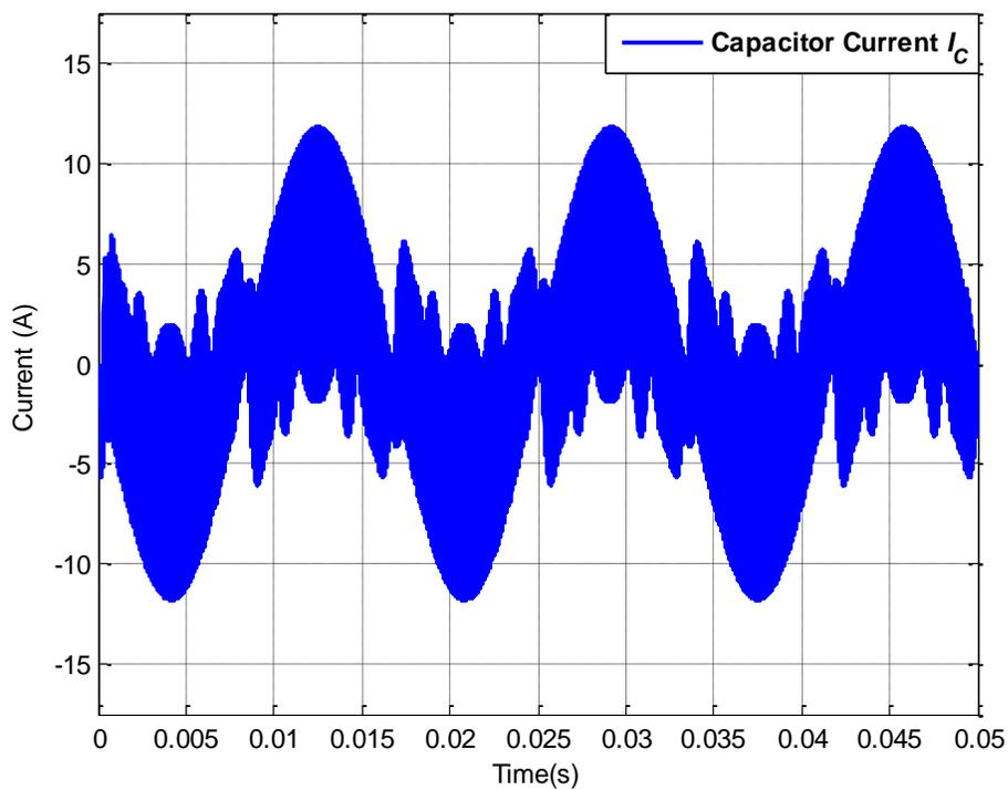
Figure A.28: Actual capacitor current  $I_C$  for operating scenario viii
