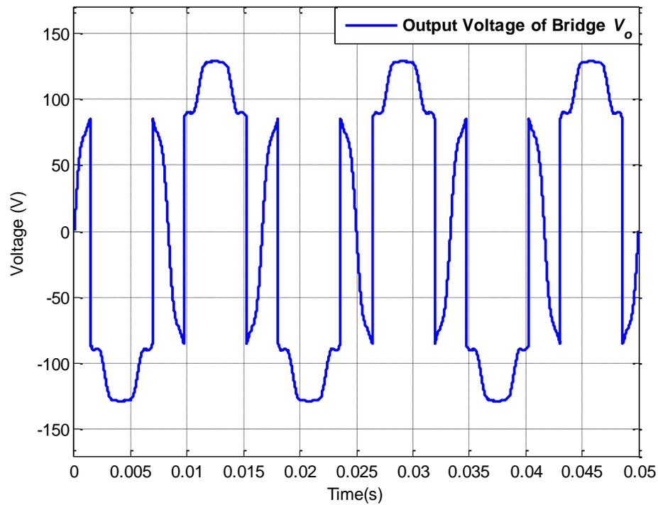
Figure 6.47: Bridge output voltage  $V_o$  for operating scenario XII
