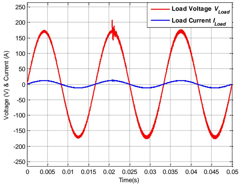
Figure 6.77: Load voltage  $V_{Load}$  and load current  $I_{Load}$  for operating scenario XVI
