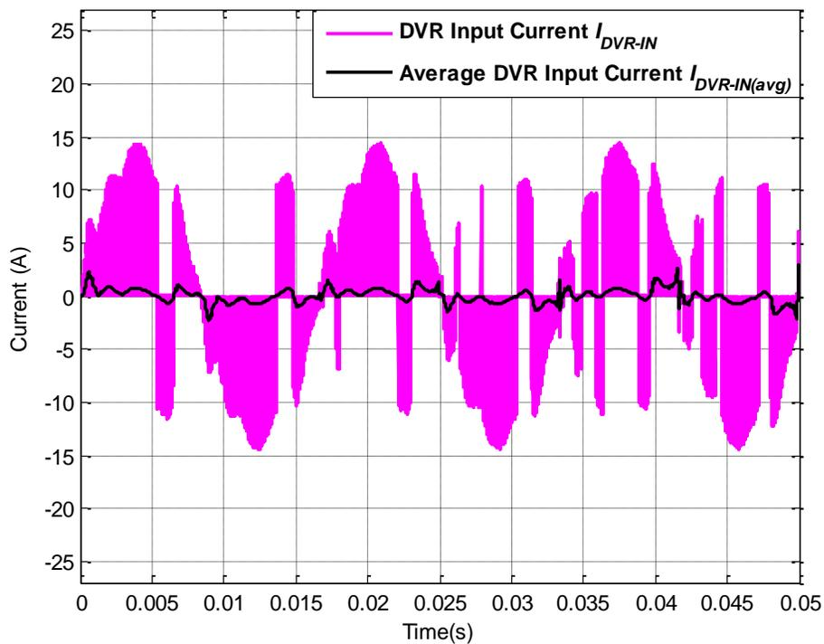
Figure A.47: Actual DVR current  $I_{DVR-IN}$  and average DVR current  $I_{DVR-IN(avg)}$  for operating scenario xiii
