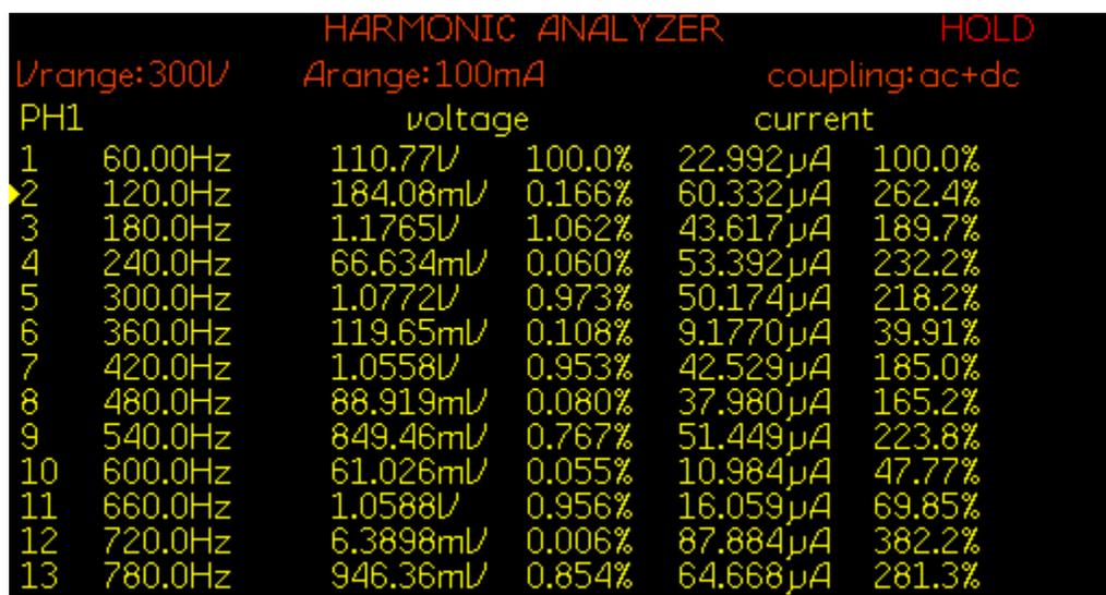
Figure 7.47: FFT of load voltage  $V_{Load}$  for experiment scenario VIII
