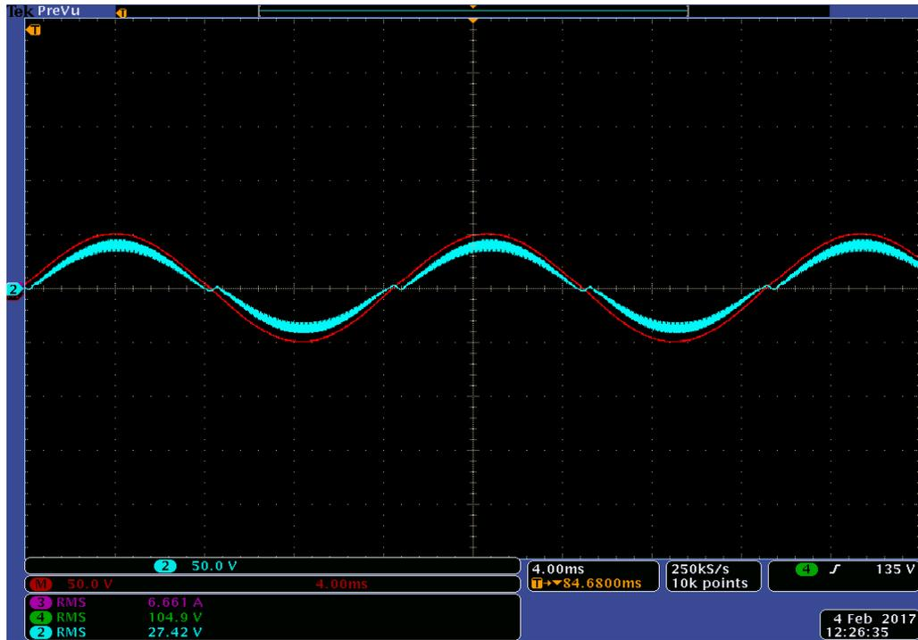
Figure 7.64: Experimental results of AC-DVR voltage  $V_{AC-DVR}$  (Blue) and DVR reference voltage  $V_{Ref-DVR}$  (Red) for experiment scenario X
