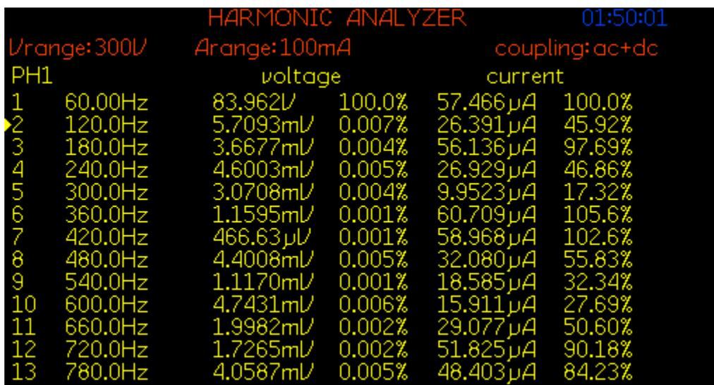
Figure 7.62: FFT of source voltage  $V_{in}$  for experiment scenario X
