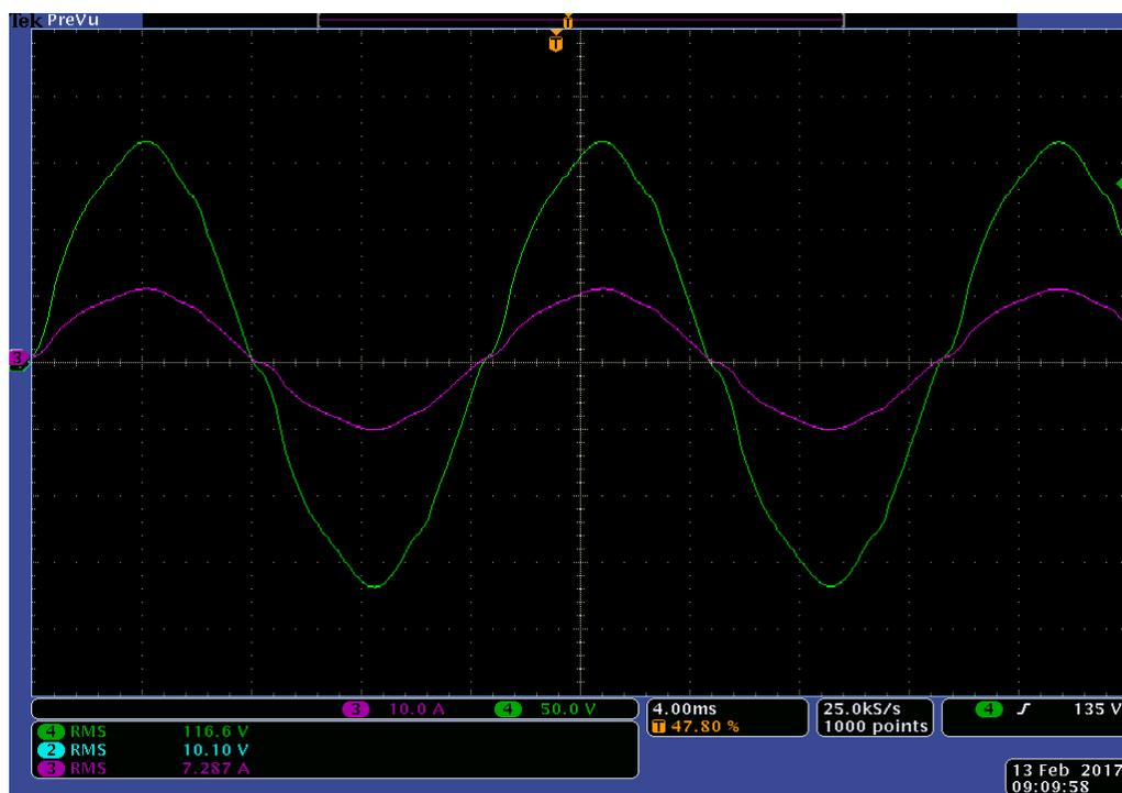
Figure 7.89: Experimental Results of Load voltage  $V_{Load}$  (Green) and load current  $I_{Load}$  (Pink) for experiment scenario XIII
