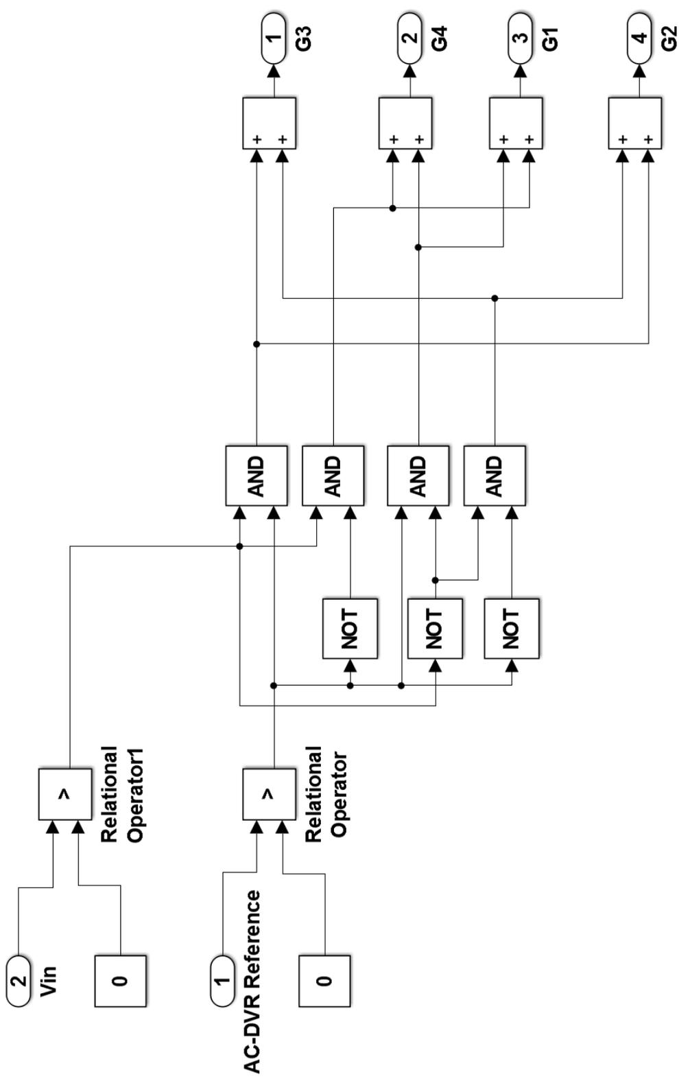
Figure 5.5: Control logic for bidirectional switches Q1Q2', Q2Q1', Q3Q4' and Q4Q3'
