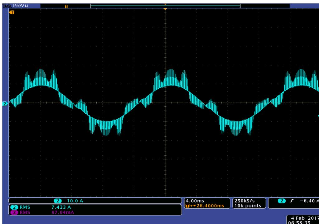
Figure 7.48: Experimental Results of Actual source current  $I_{in}$  for experiment scenario VIII
