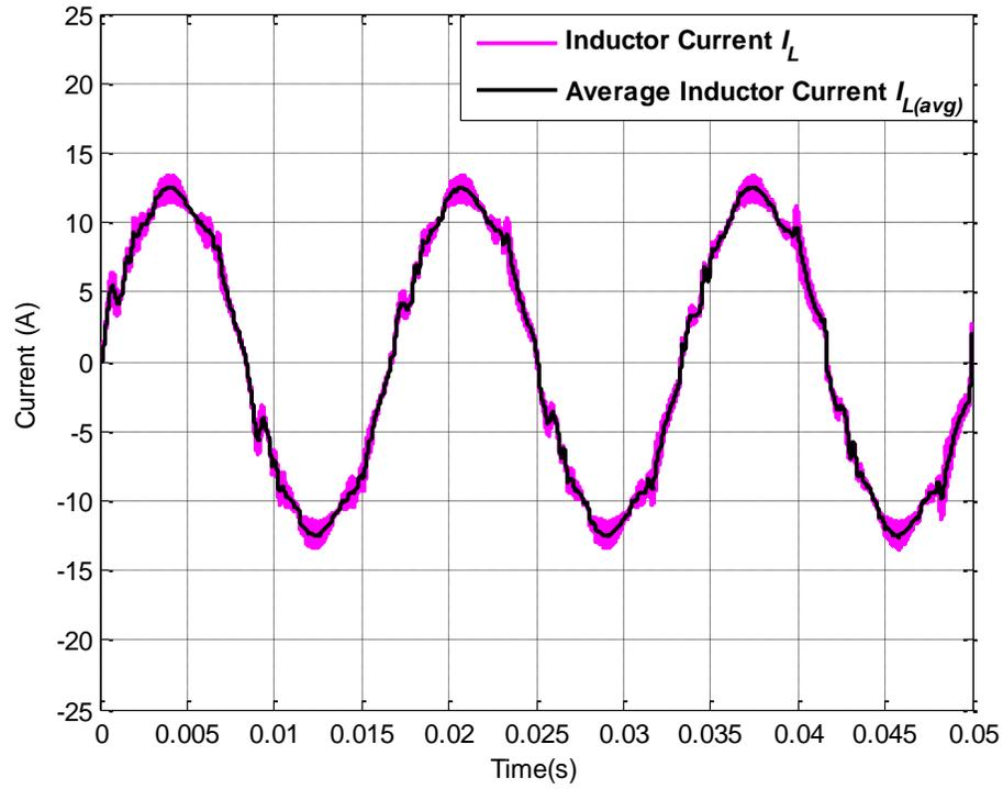
Figure 6.56: Actual inductor current  $I_L$  and average inductor current  $I_{L(avg)}$  for operating scenario XIII
