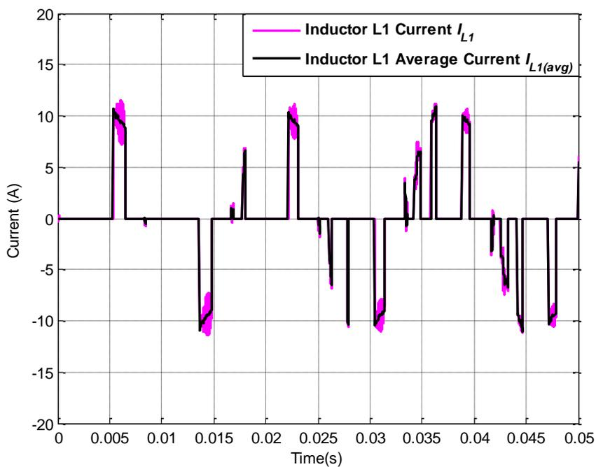
Figure A.48: Actual inductor current  $I_L$  and average inductor current  $I_{L(avg)}$  for operating scenario xiii
