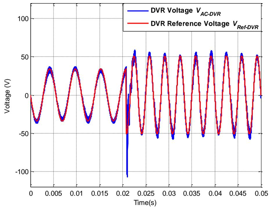
Figure 6.80: AC-DVR voltage  $V_{AC-DVR}$  and DVR reference voltage  $V_{Ref-DVR}$  for operating scenario XVII
