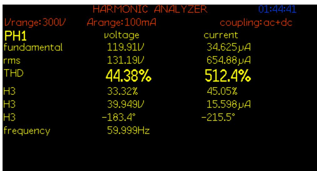
Figure 7.53: THD of source voltage  $V_{in}$  for experiment scenario IX
