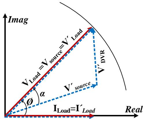
Figure 2.10: Pre-sag compensation phasor diagram
