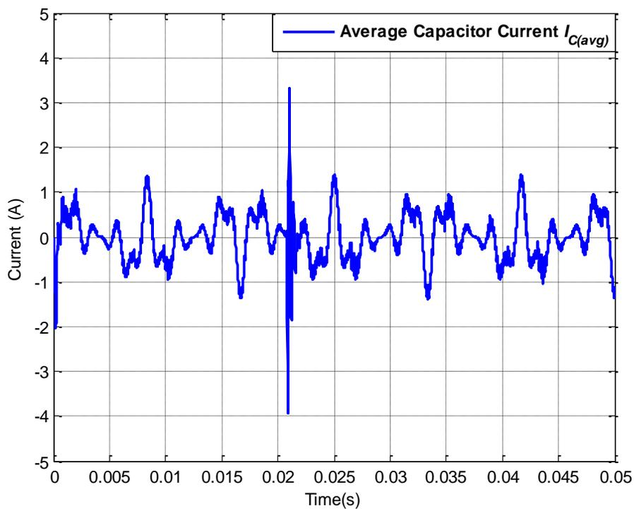
Figure A.64: Average capacitor current  $I_{C(avg)}$  for operating scenario xv
