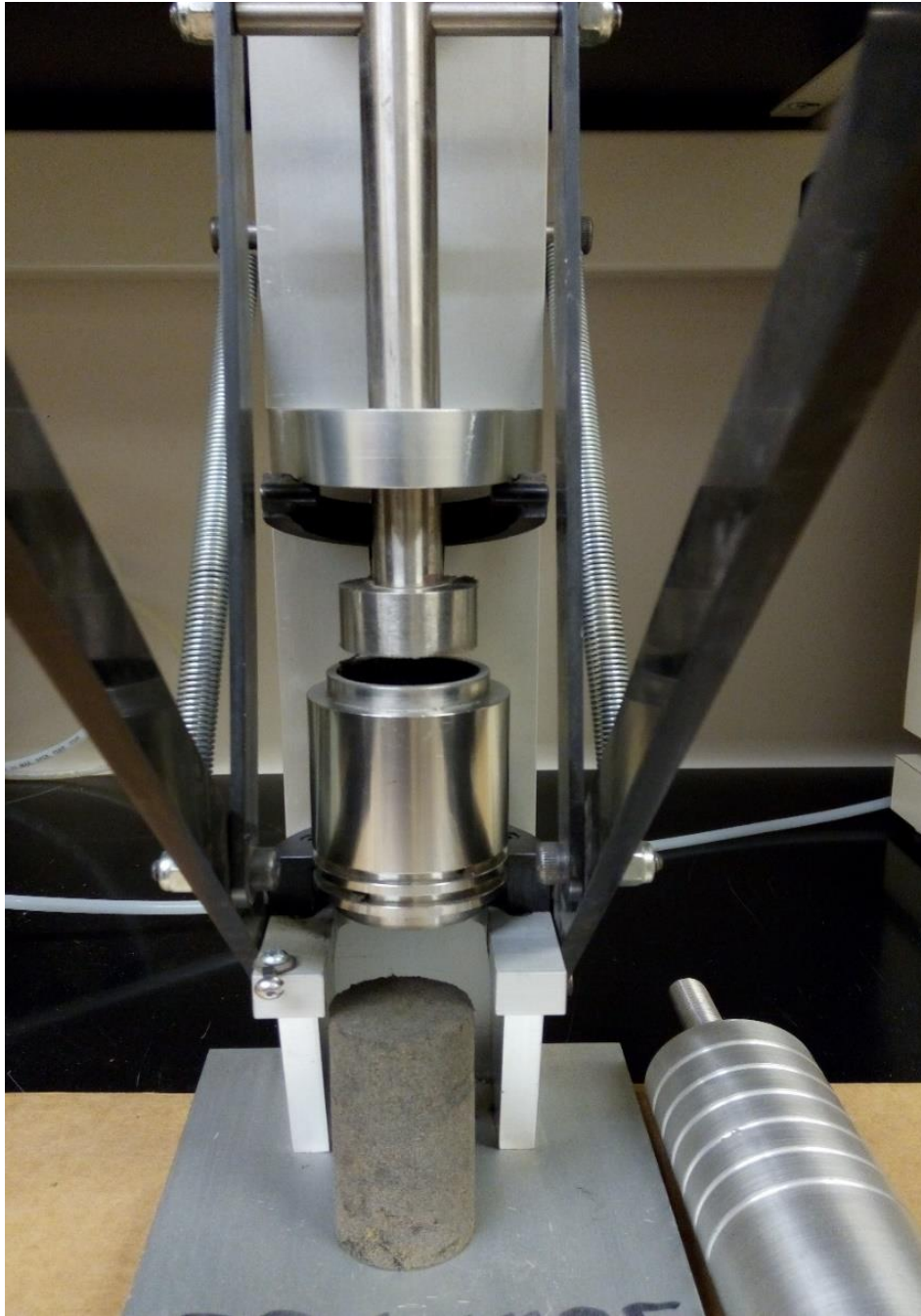
Figure 4-4 Harvard Miniature samples extraction for Unconfined Compression Testing
