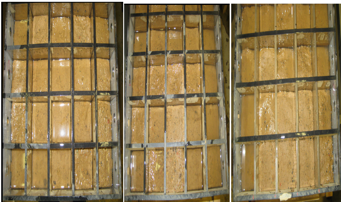
Figure 11: Setup of treated soil samples in sandboxes
