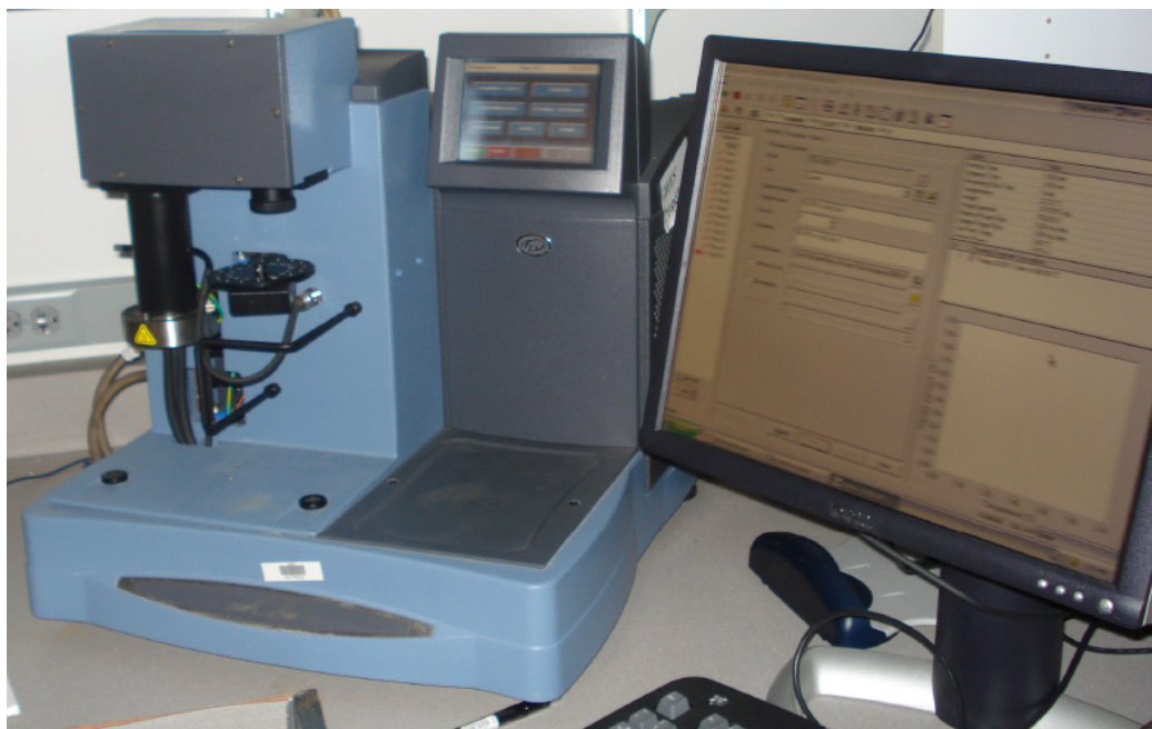
Figure 14: TGA analysis instrument used in this research
