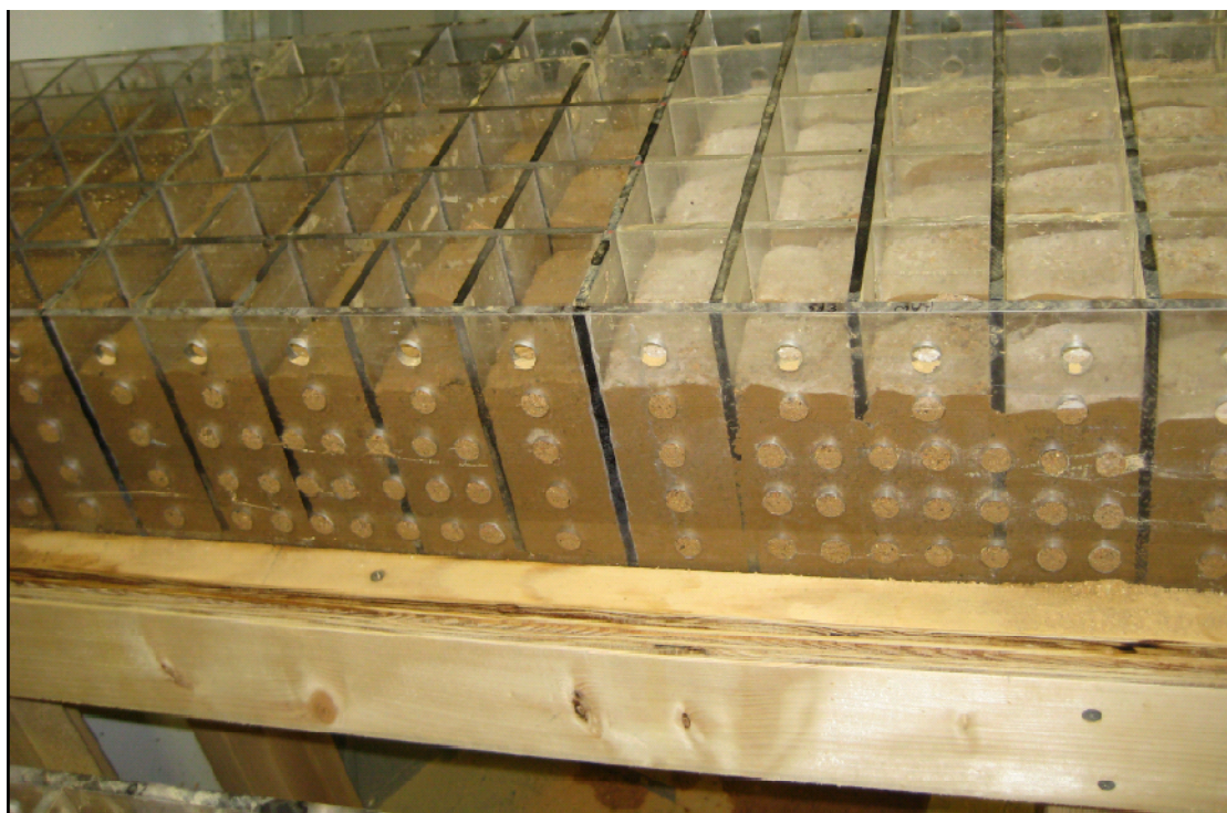
Figure 12: Soil samples after treatments in sandboxes
