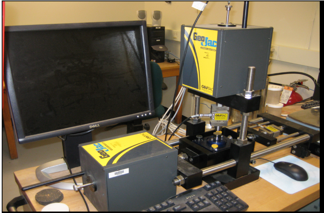
Figure 13a: Direct shear strength testing instrument used in this research
