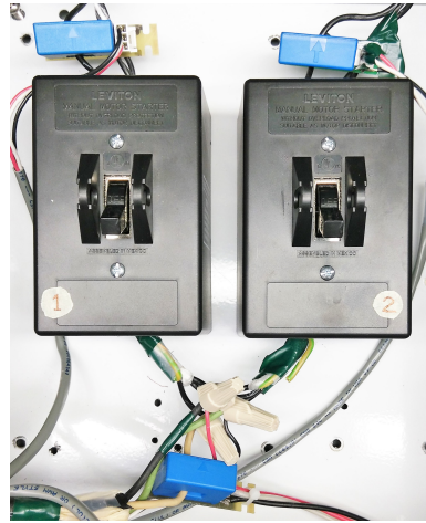
Figure 4.4: Three phase switches splitting the line for parallel connection to the motors
