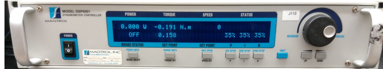
Figure 4.6: Controller for the dynamometer, amount of torque generated by the load is controlled.
