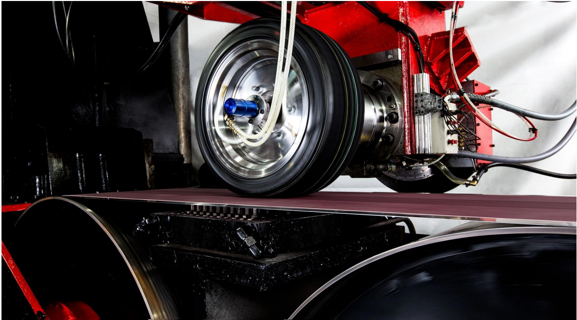
Figure 1.3: Calspan Flat Belt Tire Testing Machine
