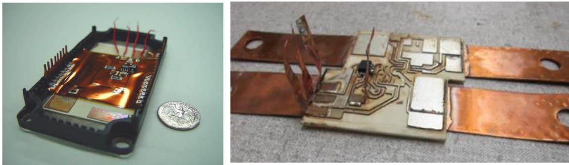
Figure 2.25: GMR current sensors implemented for measuring currents in IGBTs [84]
