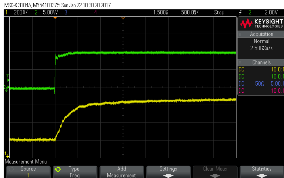
Figure 3.11: AMR sensor response for 10A step current
