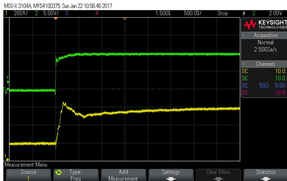
Figure 3.12: GMR sensor response for 10A step current
