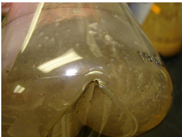
FIGURE 4.2: Stress cracks at molded vanes led to bottle leaks
