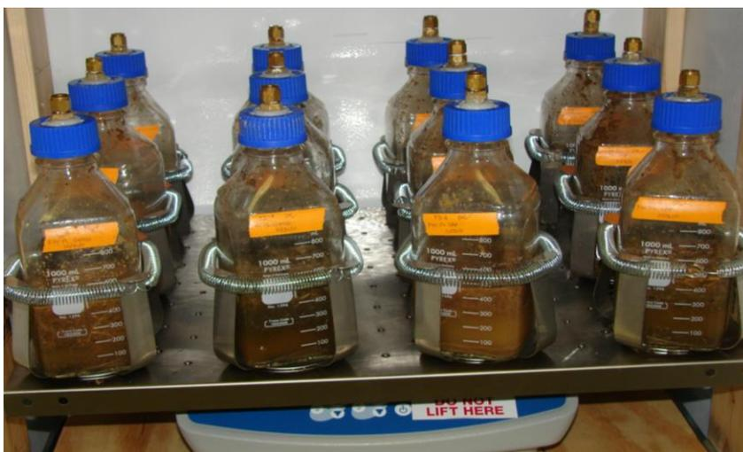
FIGURE 3.2: A photograph of the modified 1L glass bottles on a shaker
