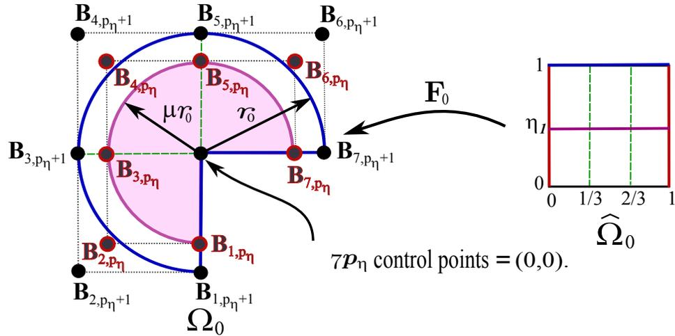
Figure 4.2: The NURBS geometrical mapping that generates singular functions on  $\Omega_0 = [0, r_0] \times [0, 3/2\pi]$  from the parameter space  $\hat{\Omega}_0 = [0, 1] \times [0, 1]$  to the singular zone  $\Omega_0$ . Note that  $\mu$  is fixed real number with  $0.5 \leq \mu \leq 0.9$ .
