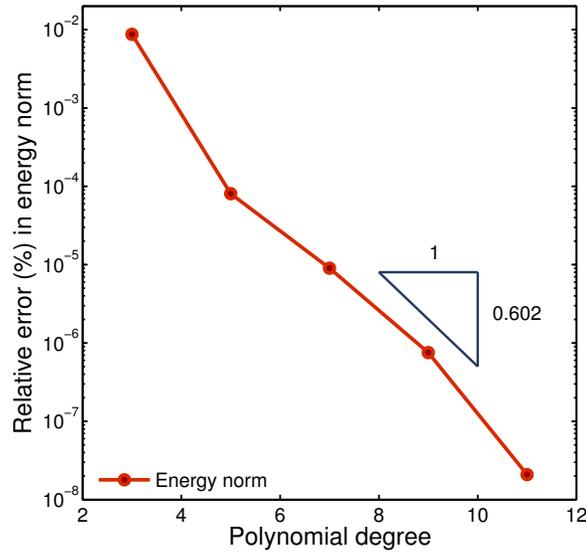
Figure 3.6: The relative error (%) in the strain energy norm of computed displacement field  $\{u, v\}^T$  of the elasticity (3.18) in the curved domain.
