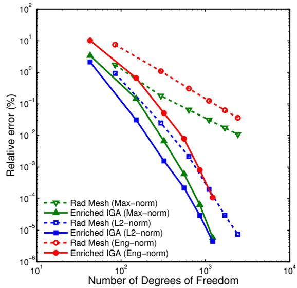
(b) Rel. errors (%) of enriched IGA and IGA with 5-radical mesh
