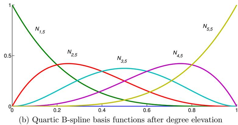
Figure 2.8: (a) The initial quadratic B-spline basis functions corresponding the open knot vector  $\Xi = \{0, 0, 0, 1, 1, 1\}$ . (b) Quartic B-spline basis functions after degree elevation of the quadratic B-spline basis functions, corresponding the open knot vector  $\bar{\Xi} = \{0, 0, 0, 0, 0, 1, 1, 1, 1, 1\}$
