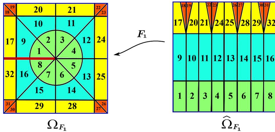
Figure 4.17: Integral areas on the parameter space  $\hat{\Omega}_{F_1}$  of the newly designed singular mapping  $F_1$ . Note that  $\Omega_{F_1}$  corresponding to  $\hat{\Omega}_{F_1}$  is the singular zone including non flat-top area of PU functions in the physical domain.
