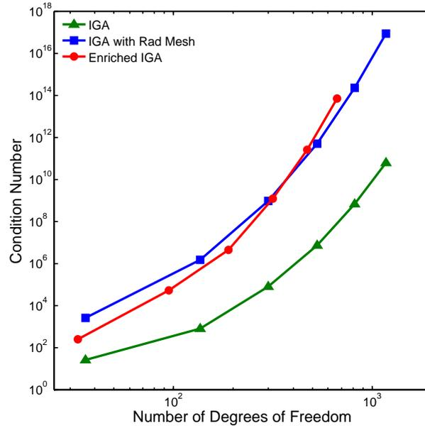
Figure 4.5: Condition numbers of constrained Stiffness matrices for IGA, enriched IGA, and IGA with radical mesh, respectively.
