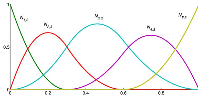
(b) Quadratic B-spline basis functions after knot insertion
