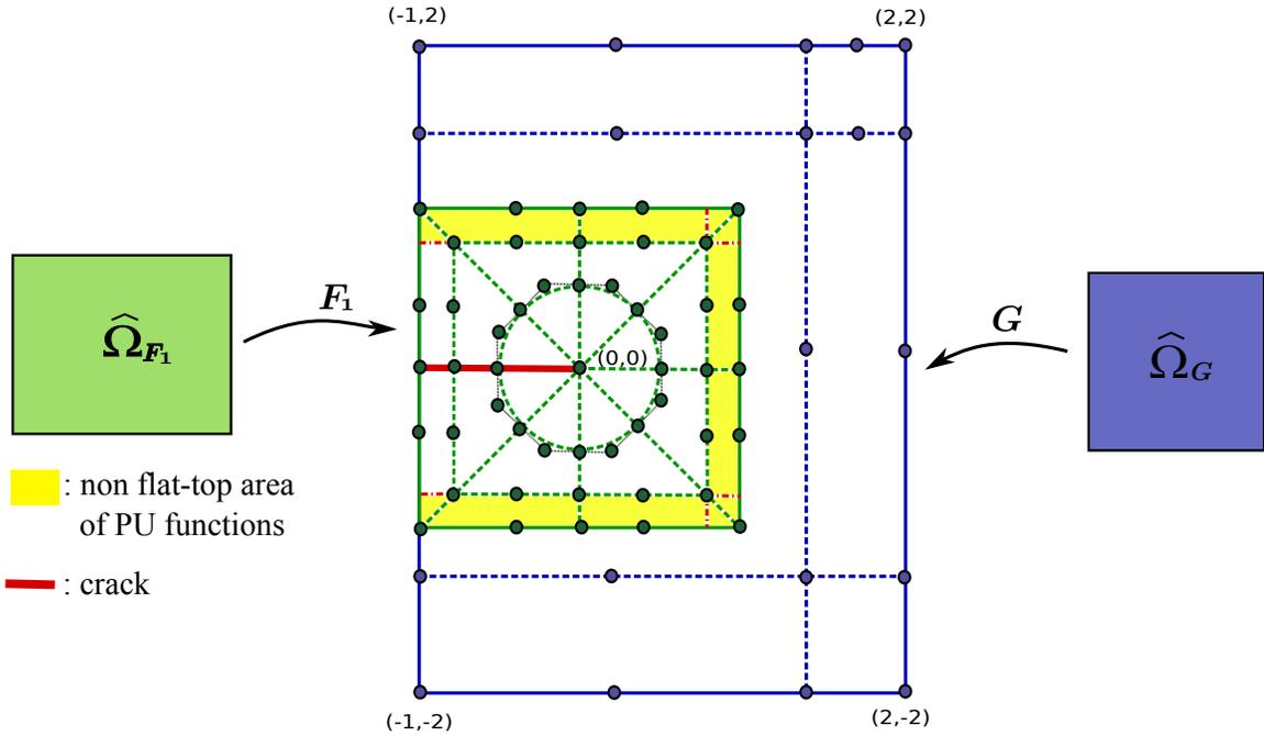
Figure 4.16: The physical domain and control points for each maps  $\mathbf{F}_1$  and  $\mathbf{G}$  of Example 4.3.1.
