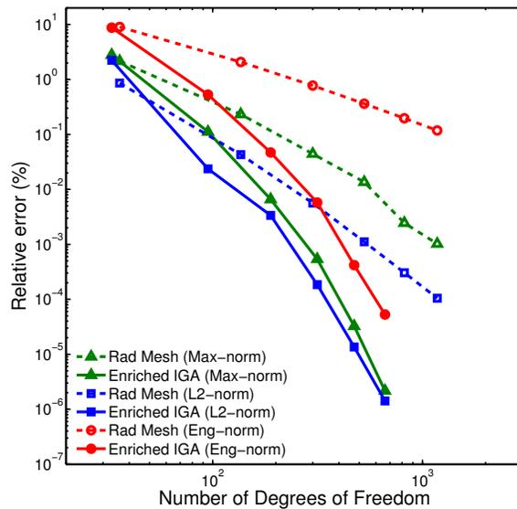
(b) Rel. errors (%) of enriched IGA and IGA with 5-radical mesh
