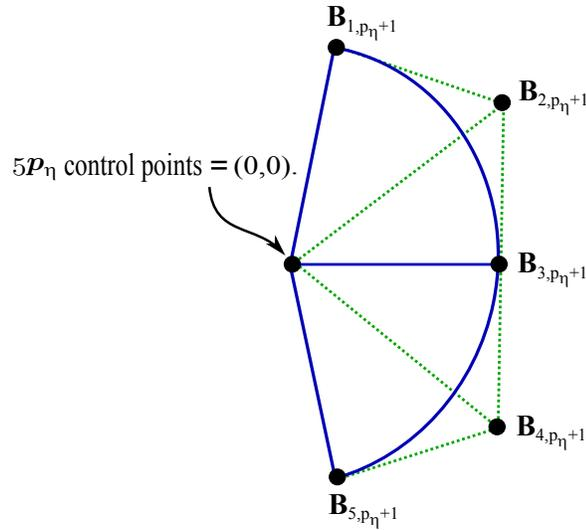
Figure 3.3: The control points for the wedge-shaped domain.
