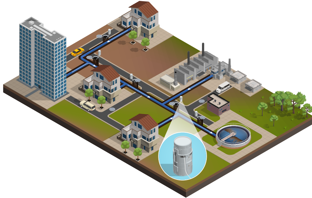
Figure 6.1: Illustration of a wastewater network with wastewater autosamplers.
