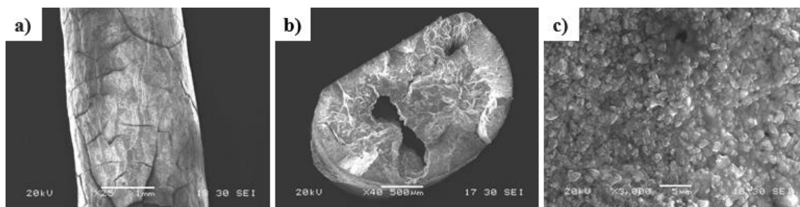
Figure 54a, b, and c SEM images of Ink D at 1000 °C, 1 °C/min, and 1 hour dwell time. (a) Surface image at 25x magnification and 1mm scale. (b) Broad cross-sectional image taken at 40x magnification and 500μm scale. (c) close-up cross-sectional image taken at 3000x magnification and 5μm scale.
