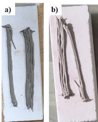
Figure 34a and b Pyrolysis of Ink A (a) before and (b) after pyrolysis at 900 °C, 3.5 °C/min, and 1 hour dwell time.
