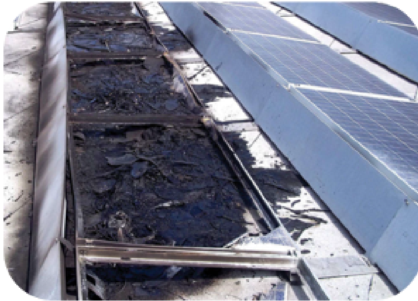
Figure 1.2: Arc fault fire hazard: 1,208kW PV array, Mount Holly, North Carolina, 2011 [6].
