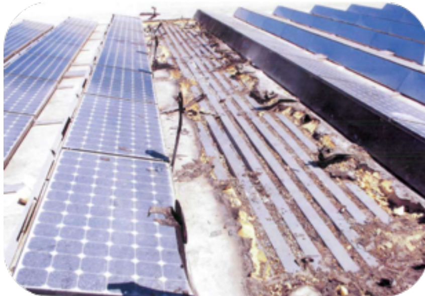
Figure 1.3: Arc fault fire hazard: 383 kW PV system, Bakersfield, CA, 2009 [7].
