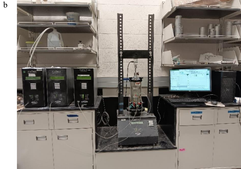
Figure 3.3: a) Schematic diagram of the testing setup (1-Cell pressure FlowTrac, 2-Inlet FlowTrac, 3-Top cap for air outlet, 4-Bottom-inlet Cap, 5-Second bottom cap used for flushing (only open during flushing), 6-Second top cap for air outlet - (closed throughout testing), 7- Inlet valve (Open only during initial permeameter filling for confining pressure), and b) actual testing setup.
