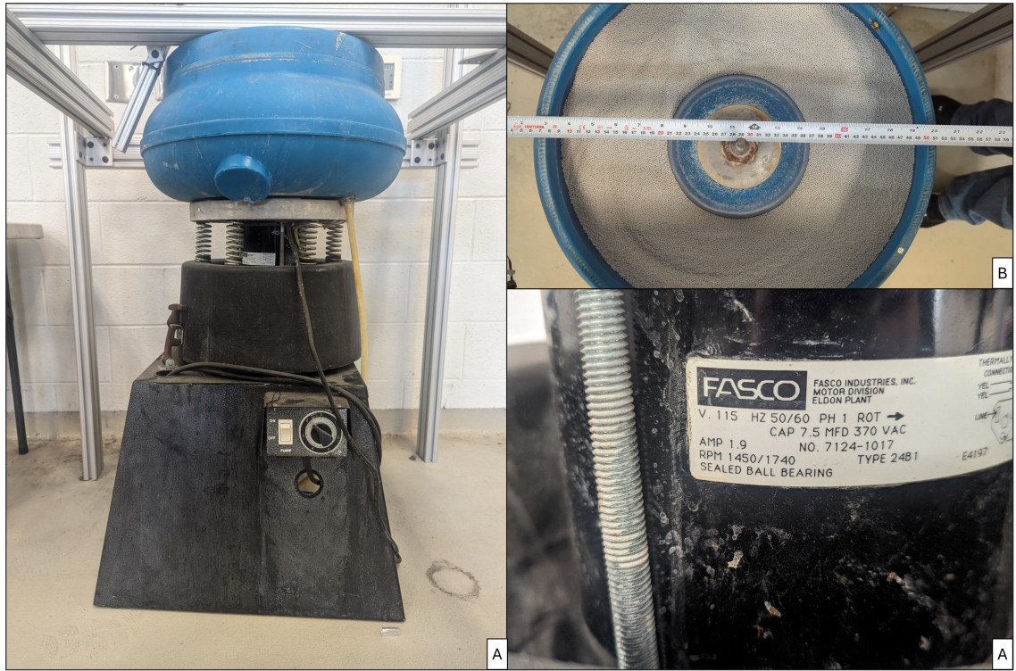
Figure 3.2: Annular shaped vibratory polishing bowl with a single-speed unbalanced motor
