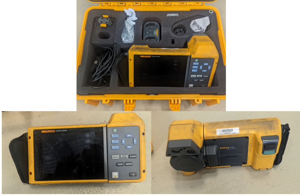
Figure 2.2: Multiple Views of the Fluke TiX580 Infrared Camera
