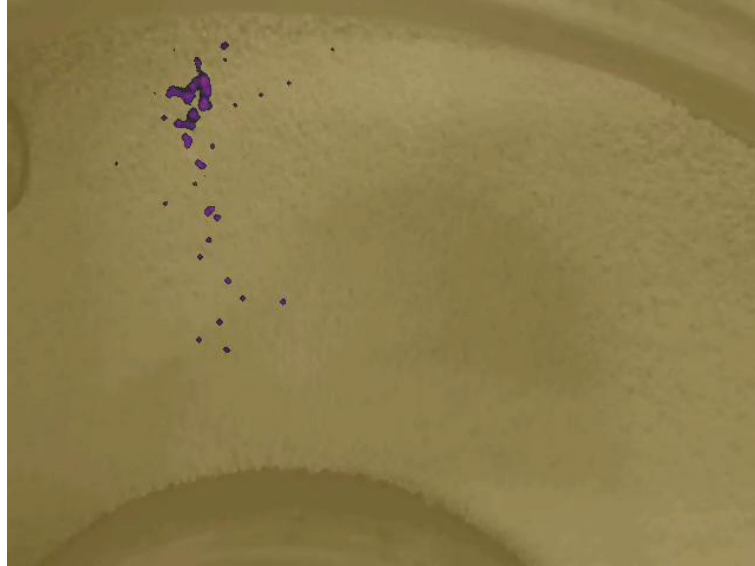
Figure 3.5: Thermal and Visible Spectrum, Blended Image of Heated Grains moving across the Flow-Field
