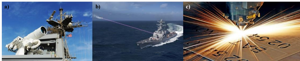
Figure 1: Applications for high energy laser systems for defense and manufacturing, a) is a 30-kilowatt AN/SEQ-3 laser weapon system (LaWS) aboard a U.S. destroyer (US Navy USS Ponce, 2014), b) is the Optical Dazzling Interdictor, Navy, or ODIN system, and c) a commercial application of HEL systems used for laser cutting.
