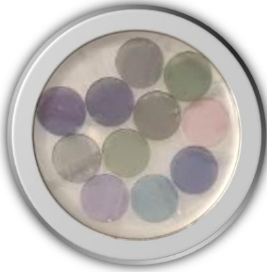
Figure 21: Fused silica substrates with various metal masks fabricated on the surface. The wide range of colors are a result of a wide range of Au feature geometries and spacings.
