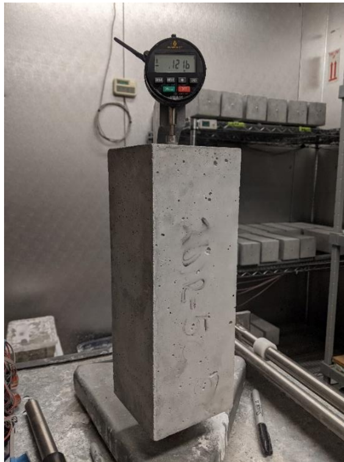
Figure 3-4. Photograph of shrinkage testing performed on a 4- by 4- by 10-in concrete prism
