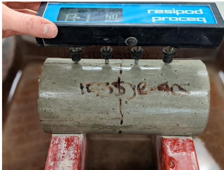
Figure 3-3. Photograph of surface resistivity testing performed on 4- by 8-in concrete cylinder
