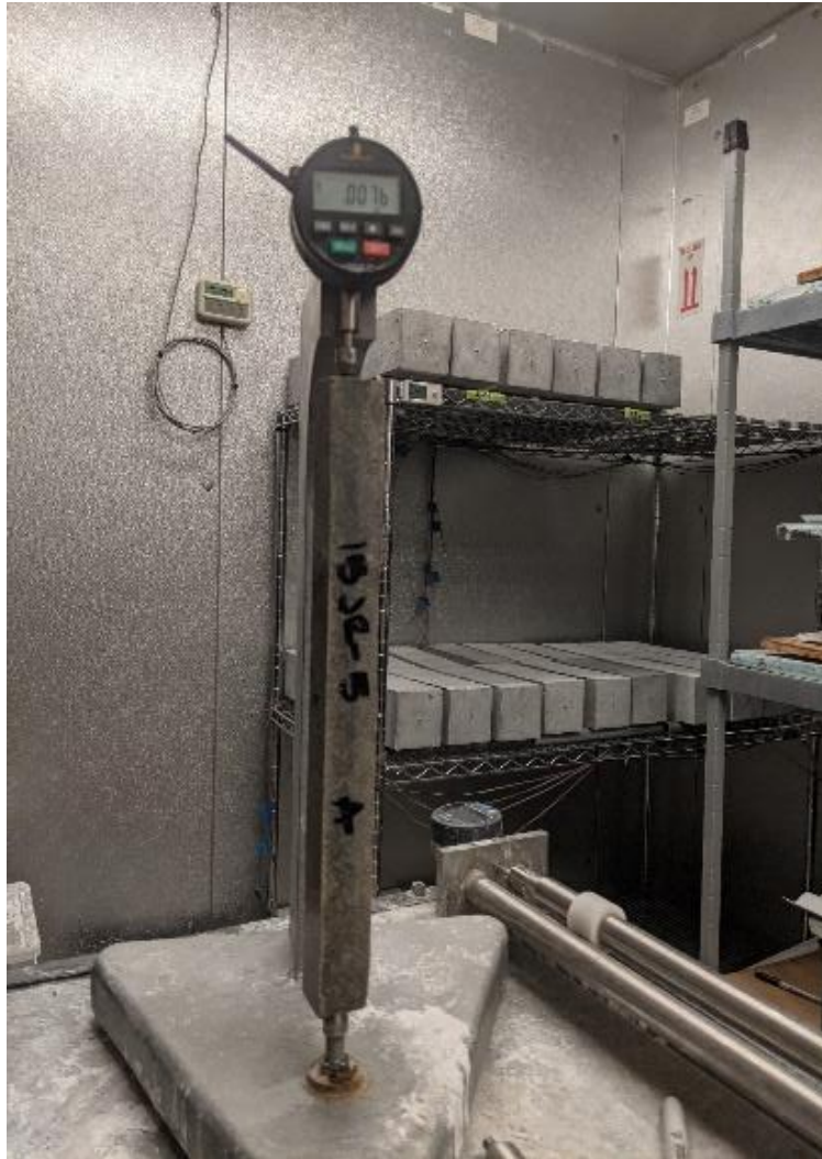
Figure 3-2. Photograph of sulfate attack testing on 1- by 1- by 11-in mortar bar
